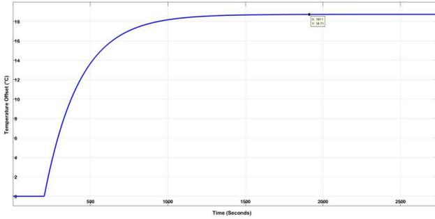
图 47. MATLAB Simulation of Thermal Offset From Load To Ambient
