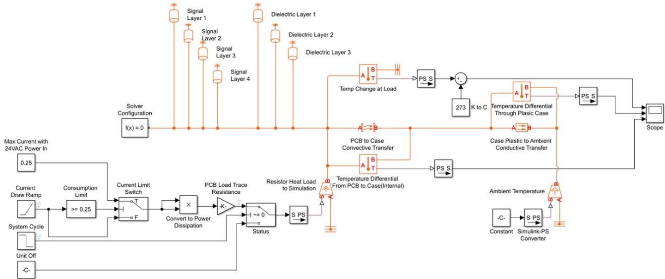
图 17. MATLAB Thermodynamic Simulation Schematic
