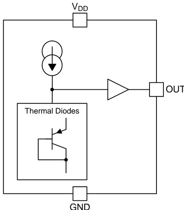
图 6. Functional Block Diagram of LMT84
