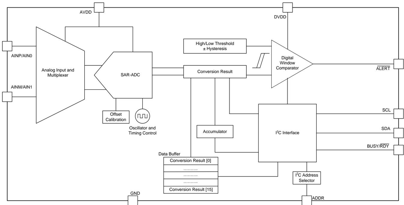
图 5. Functional Block Diagram of ADS7142
