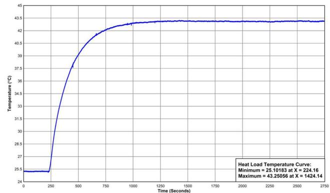
图 46. TIDA-01596 Measured Heat at 250 mA
