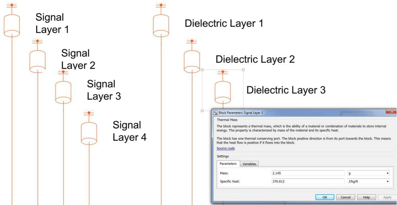
图 19. Simulation Definition of Thermal Mass
