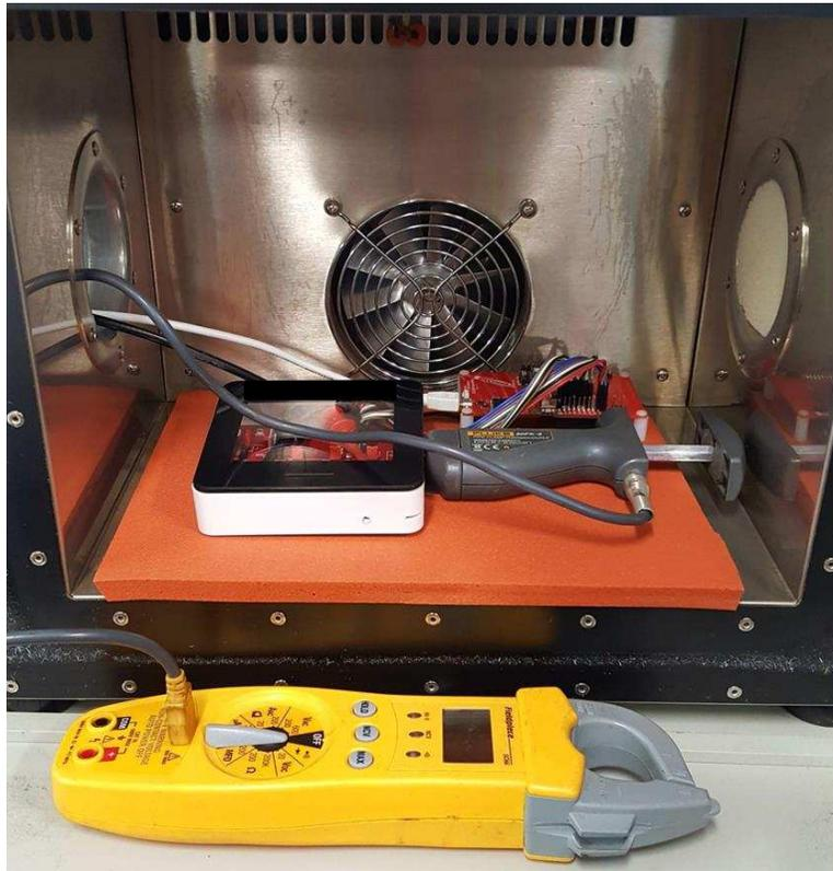
图 43. Test Setup of Temperature Chamber System
