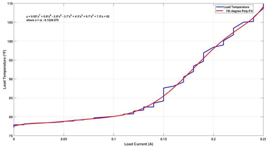
图 24. Test Circuit Load Current vs Sensed Load Surface Temperature
