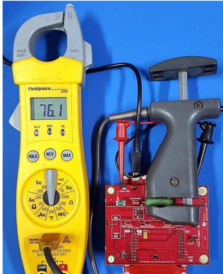
图 41. Test Setup of Ambient Load Temperature
