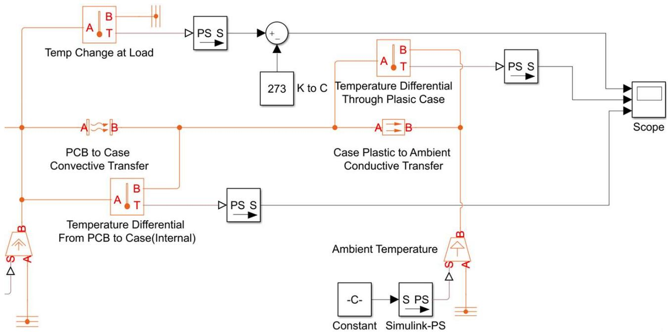
图 20. Model of Thermal Energy Dissipation
