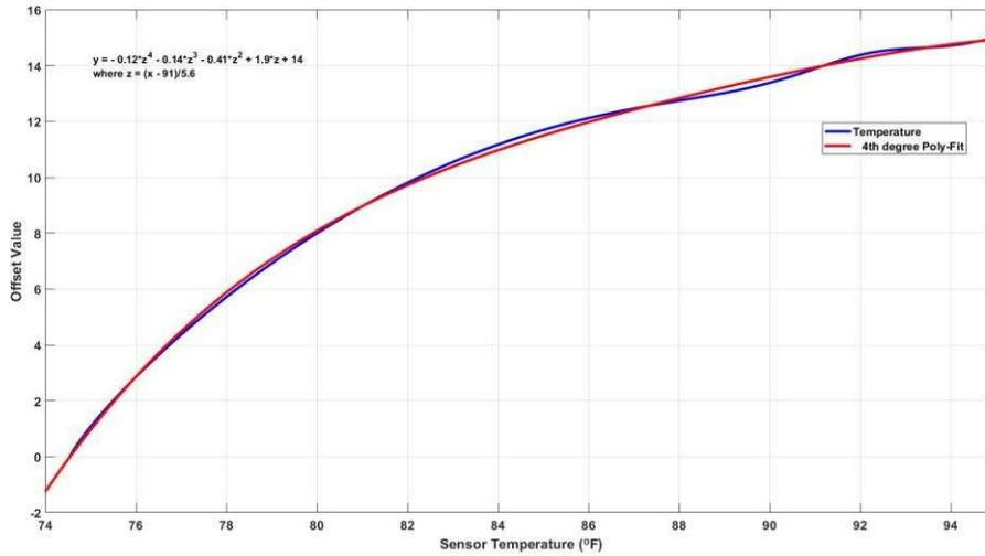
图 26. Load to Sensor Offset Curve
