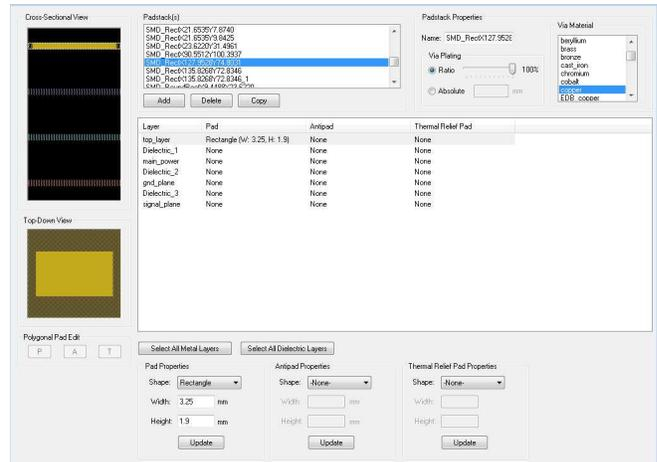
图 9. Slwave Padstack Parameter Definition
