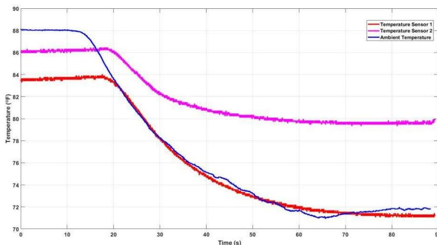
图 30. TMP235 Sensed Temperature vs Ambient Air Temperature
