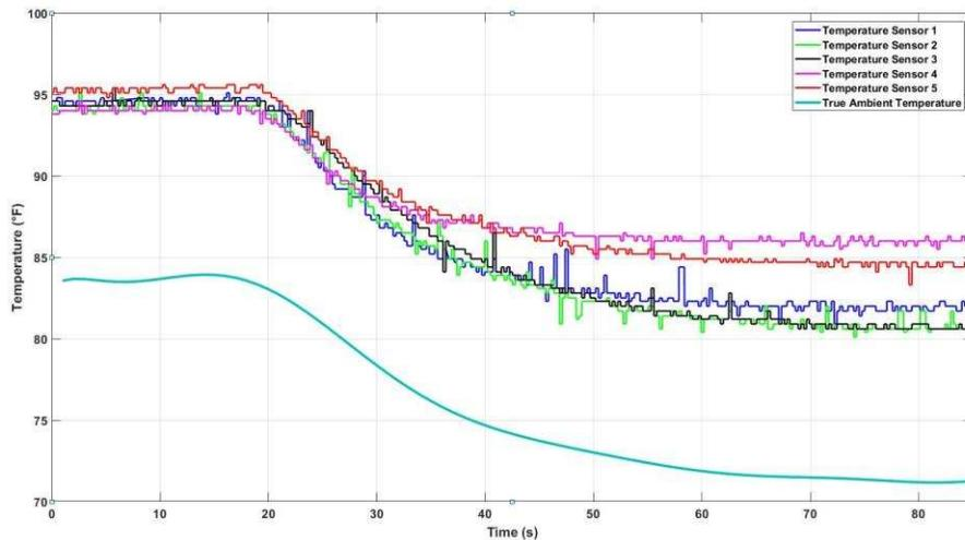
图 32. LMT84 Convective Sensing Output vs True Ambient Temperature
