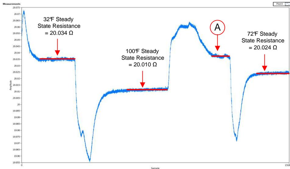
图 11. Resistance Variation Over Temperature
