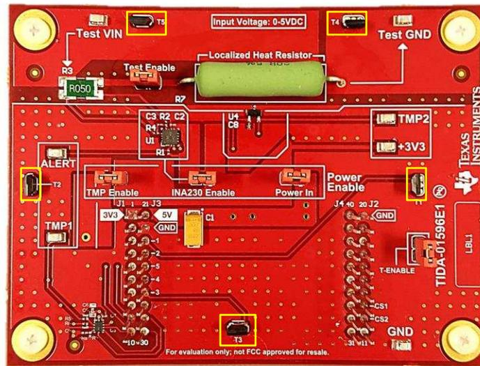
图 16. LMT84 PCB Locations for Convective Sensing
