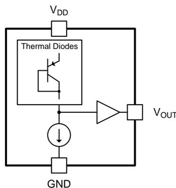
图 2. Functional Block Diagram of TMP235
