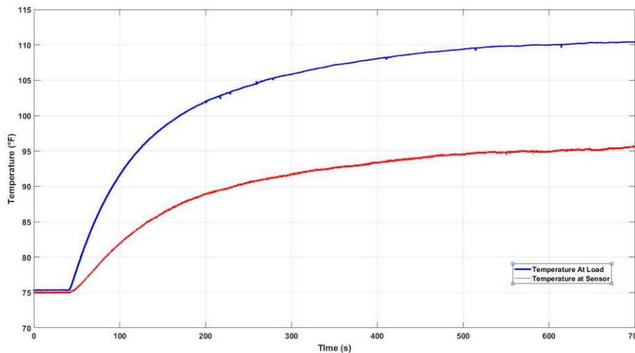
图 25. System Load Temperature vs Temperature Sensor Near Load
