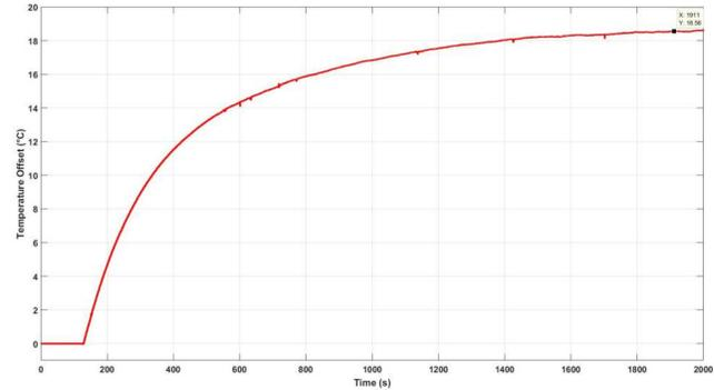
图 48. TIDA-01596 Measured Thermal Offset From Load to Ambient
