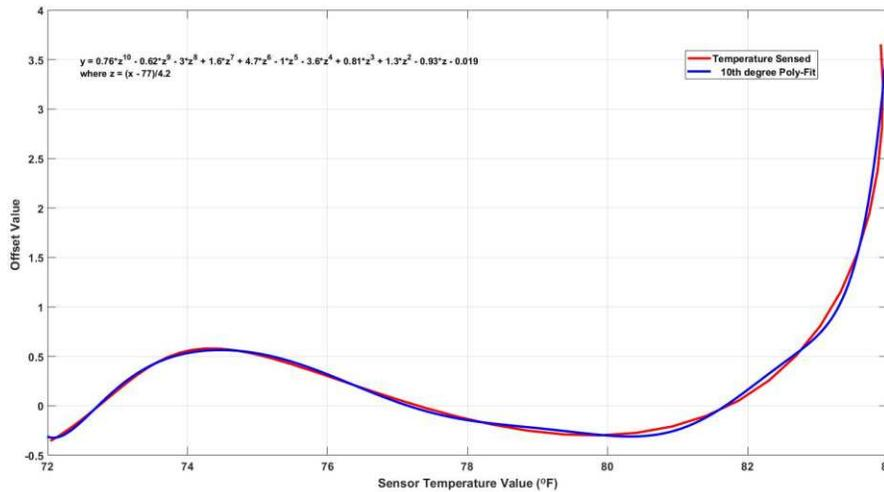
图 31. Sensor 1 vs Ambient Temperature Curve
