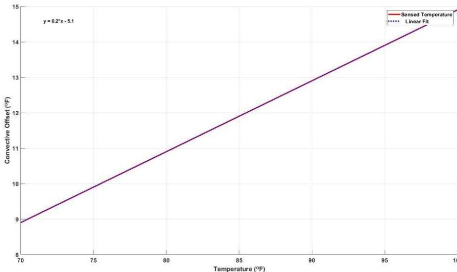
图 33. Poly-Fit Curve of Convective Sensing Offset Value
