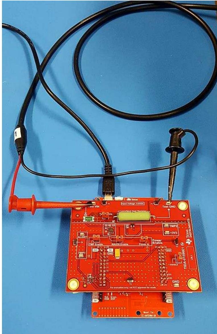
图 36. Board Setup for Firmware Deployment
