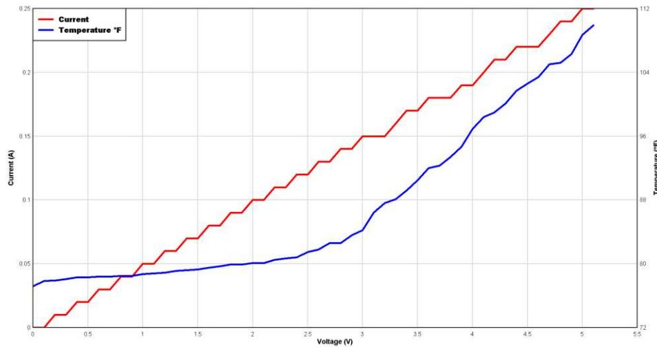
图 23. Current and Temperature Relation Based on Applied Voltage
