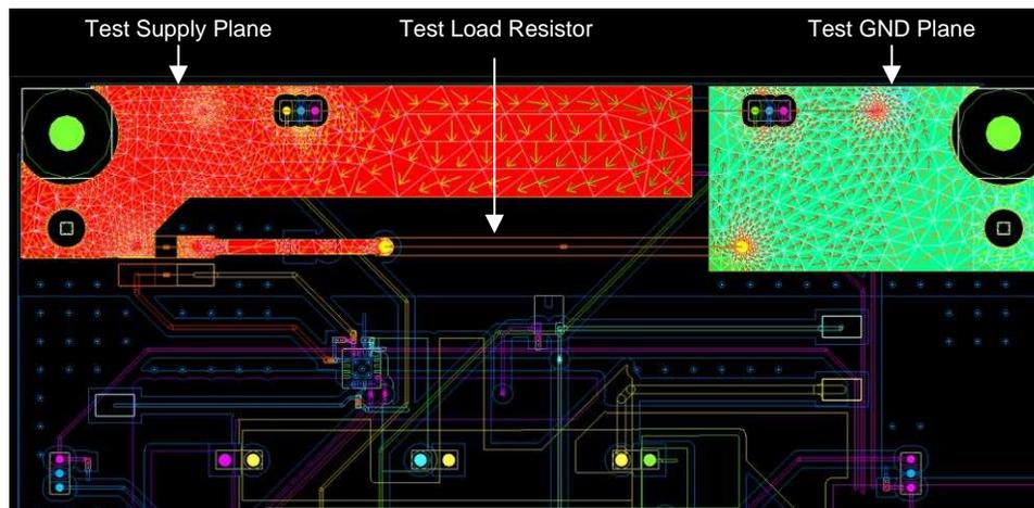
图 10. Siwave DC-IR Simulation Results
