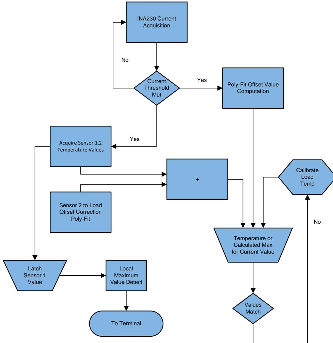
图 29. Flow Chart of Current and Temperature Monitoring Algorithm
