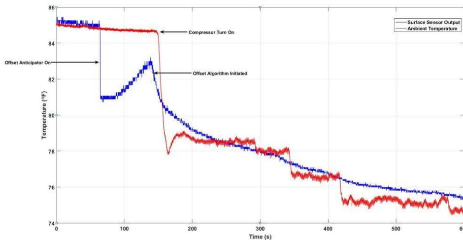
图 50. Results of Surface Sensor Offset Correction
