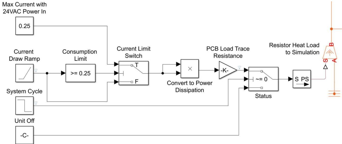
图 18. Simulation of Signal Chain of HVAC Thermostat Cycle
