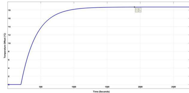
图 22. Estimated Temperature Offset From Load to Ambient in °C
