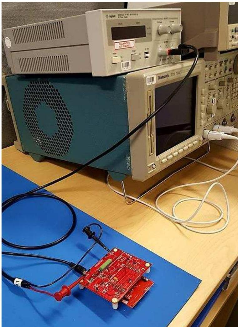
图 40. Test Setup of Initial Sensor Data Acquisition and Circuit Resistance
