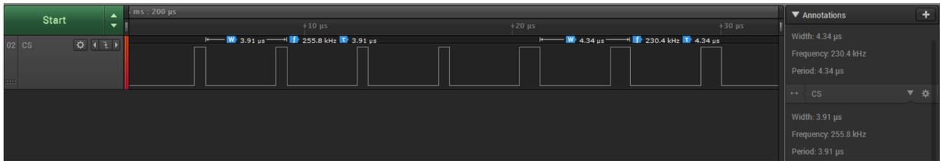
图 26. Adjusting CS for Coherent Sampling
