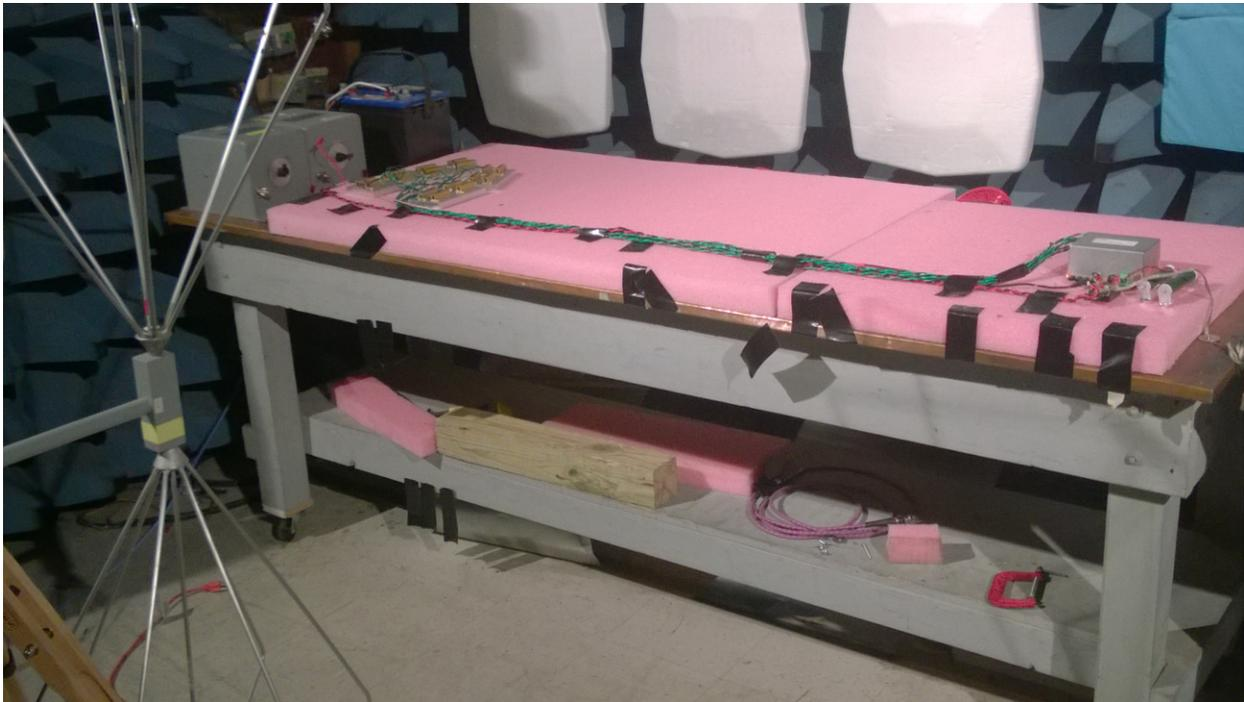
图 29. Radiated Emissions Test Setup
