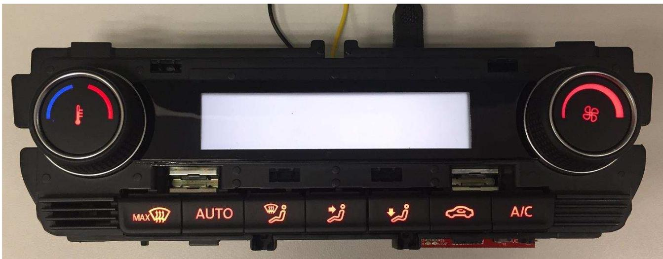
图 13. TIDA-01500 into HMI Housing
