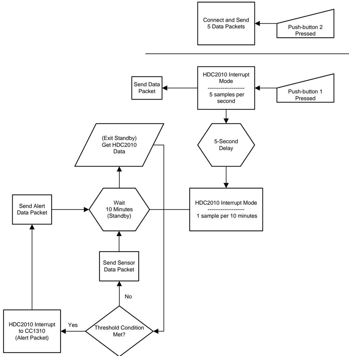
图 13. Software Flow Diagram of Main Thread
