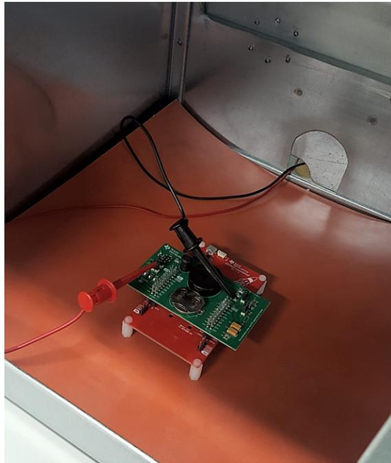
图 24. Test Setup of HDC Temperature and Humidity Threshold
