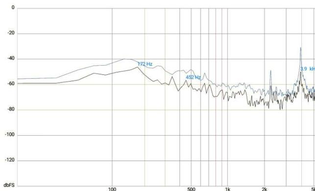
图 27. Frequency Response at 1 ft From Buzzer
