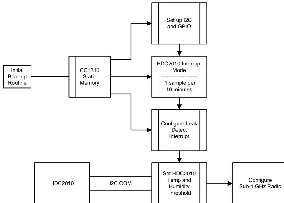
图 11. Software Flow Diagram of Initial Boot-up
