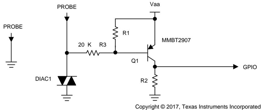
图 7. TIDA-01519 Leak Detection Schematic
