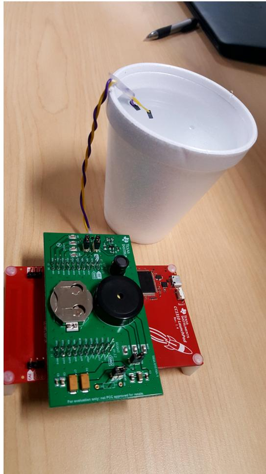
图 23. Test Setup of Water Leak Detection
