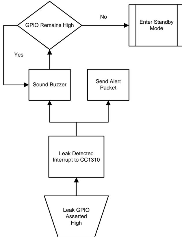
图 12. Software Flow Diagram of Water Leak Detected
