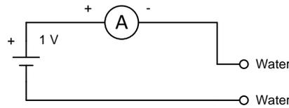
图 8. Test Setup of Water Resistance Measurement
