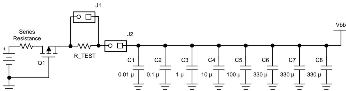
图 4. Battery Input Power Stage
