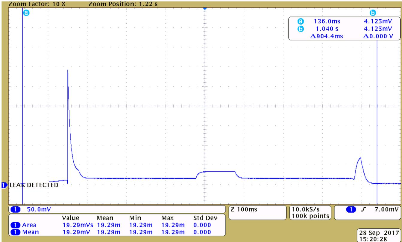
图 31. Leak Detected Packet TX With Active Buzzer Alert
