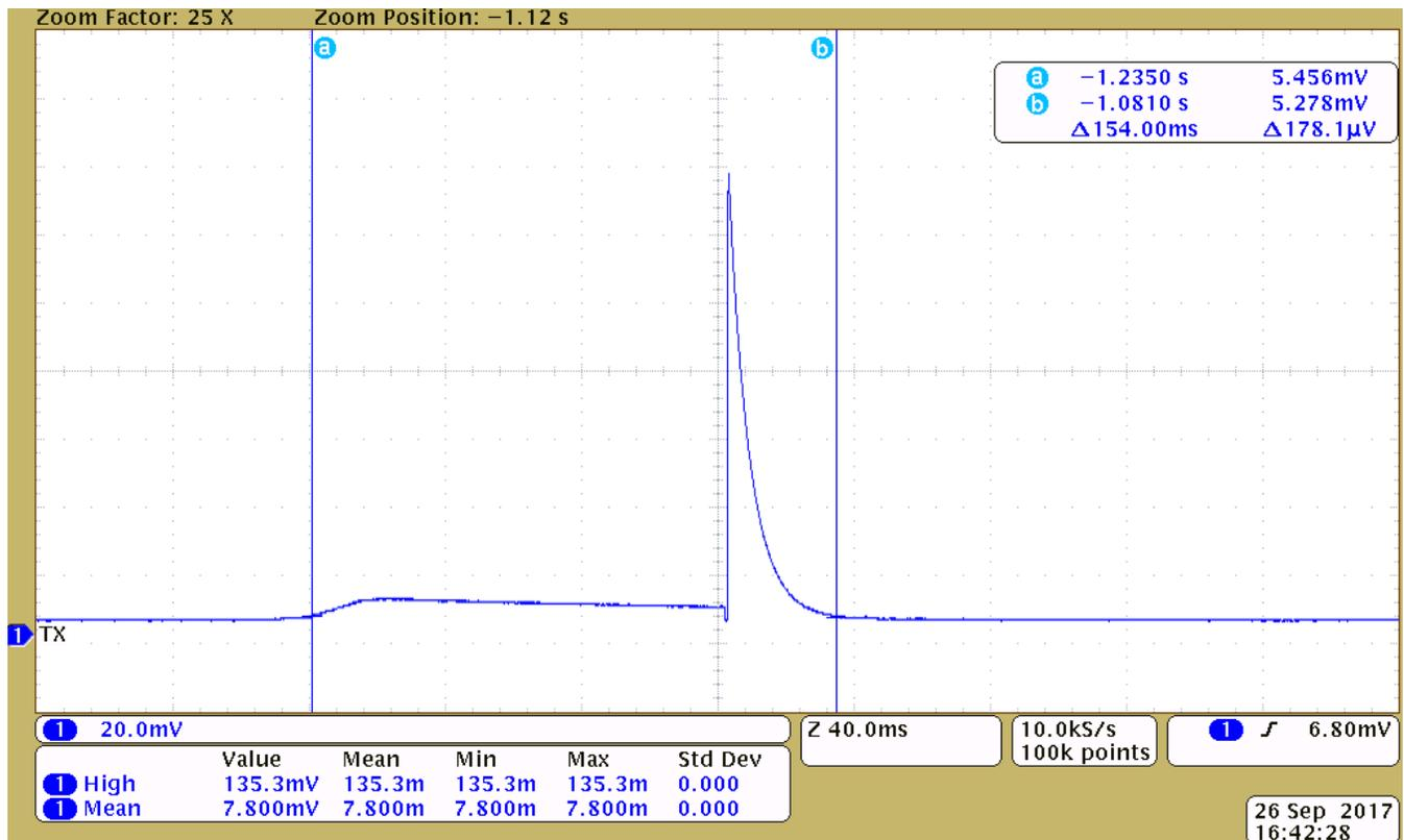
图 30. Temperature and Humidity Packet TX Waveform
