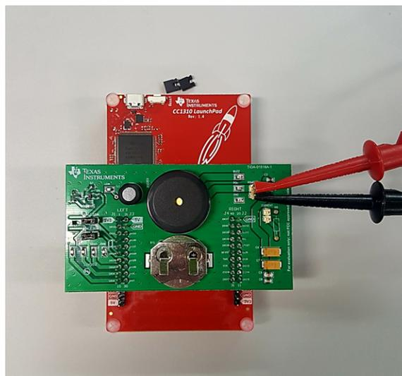
图 25. Test Setup of Main Supply Current Consumption
