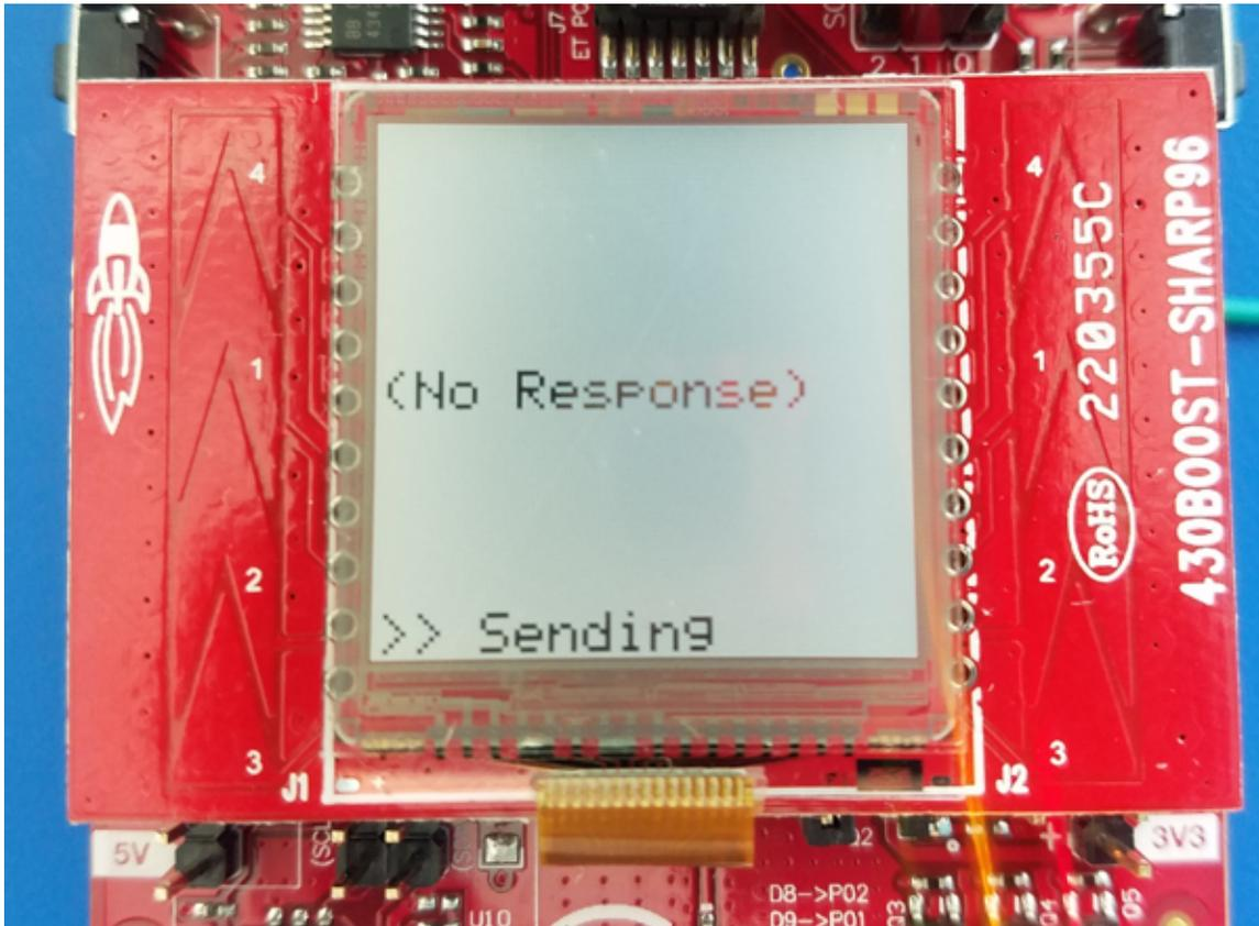
图 46. Sharp<sup>®</sup> LCD Indicates Sending Audio to IBM Watson<sup>®</sup> Servers in Progress
