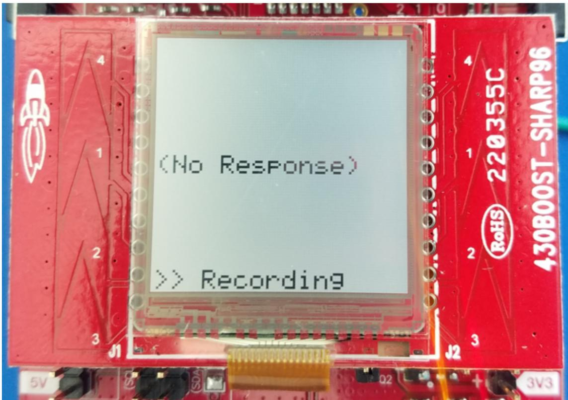
图 45. Sharp<sup>®</sup> LCD Indicates Recording in Progress
