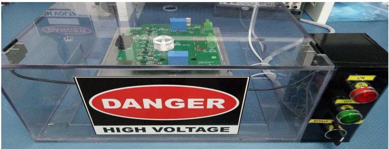
图 33. Image of Board Inside High-Voltage Safety Box
