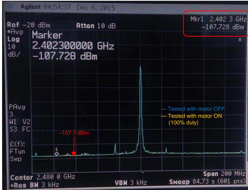
图 42. TX Performance With Bluetooth Channel Frequency of 2480 MHz
