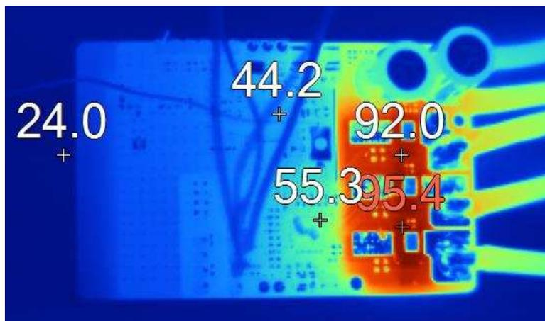
图 27. Thermal Image at 18-V DC Input, 25.6-A<sub>RMS</sub> Winding Current, 100% Duty Cycle
