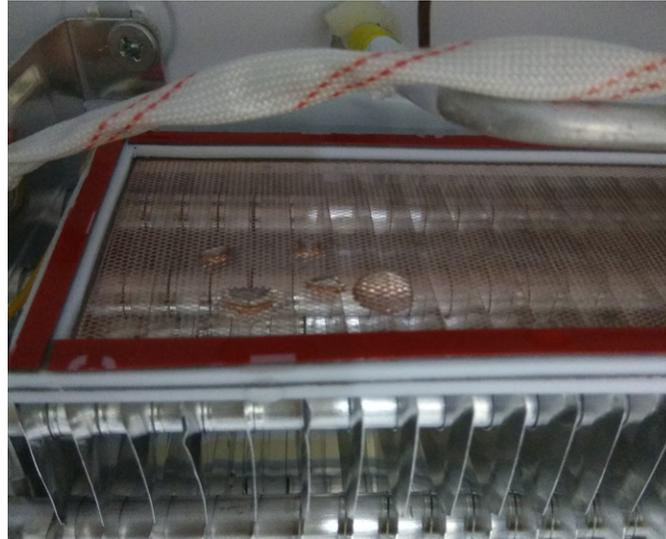
图 34. Waterdrop on Surface of Sensor
