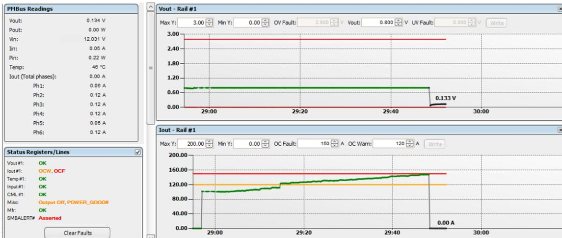
图 28. Overcurrent Shutdown as Seen in Fusion GUI
