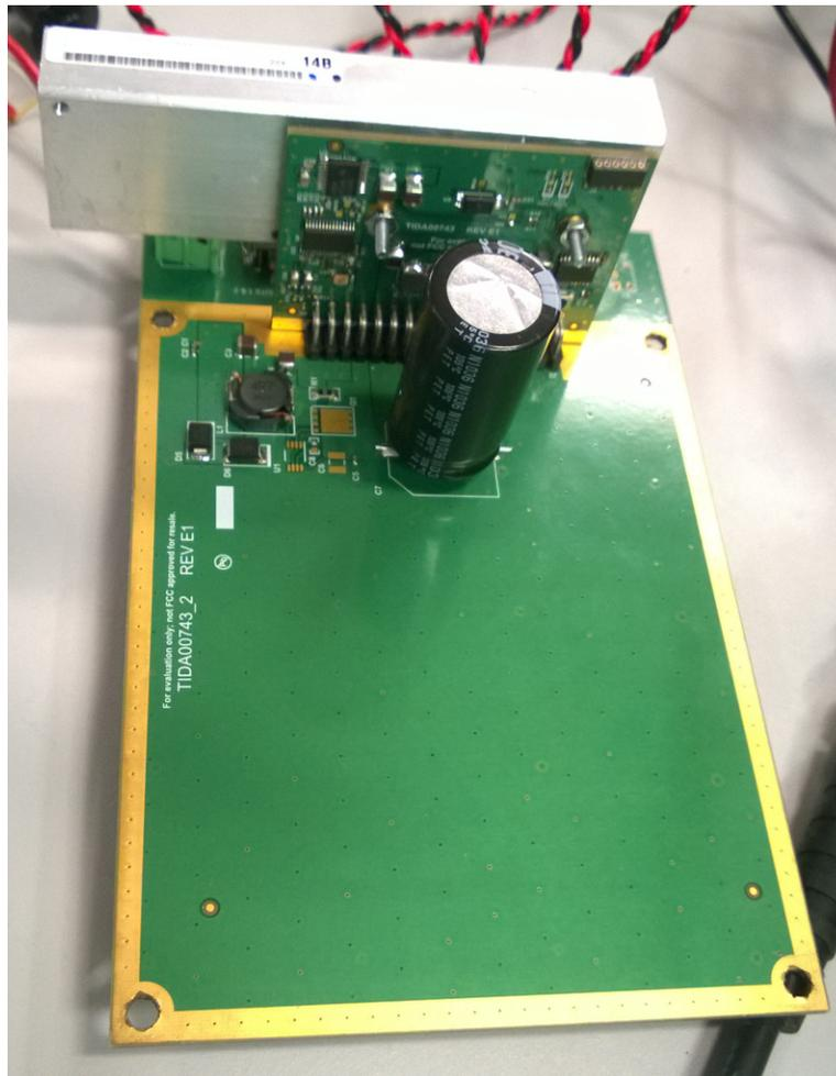
图 15. TIDA-00743 Module Board With Heat Sink Attached to Carrier Board
