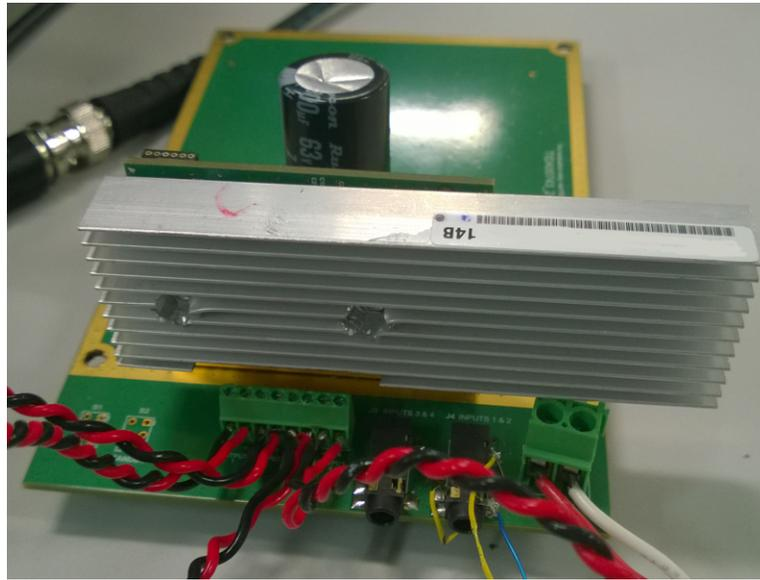
图 16. Connections for TIDA-00743 Assembly
