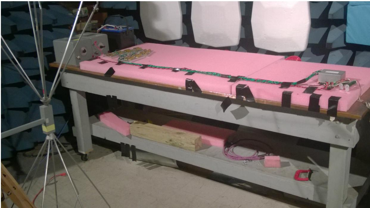
**图 20. Radiated Emissions Test Setup**
