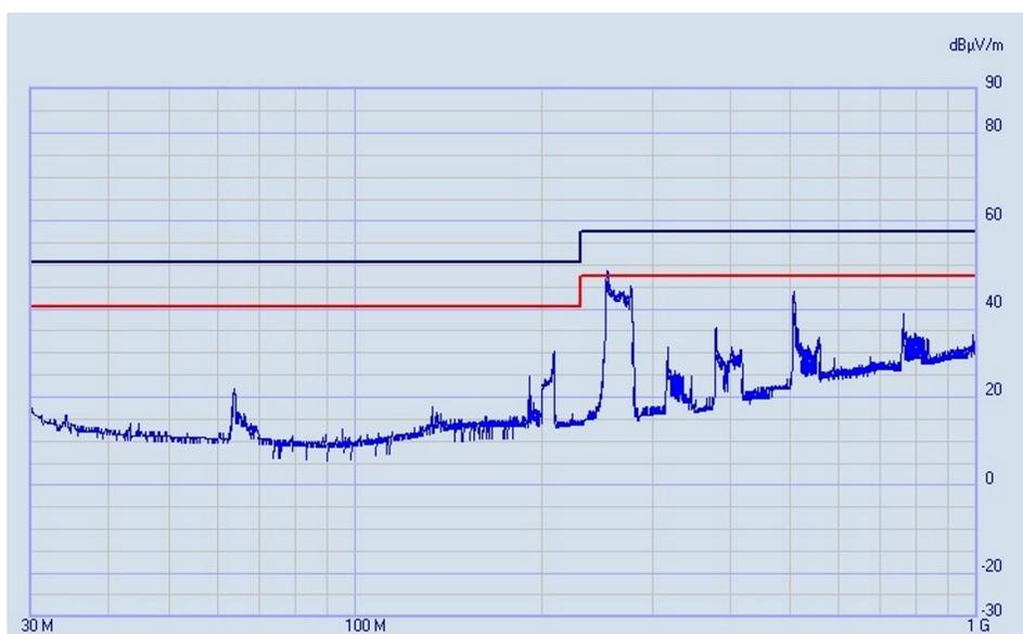
图 16. Radiated Emission Plot for ISOW7841-Based BIM at 3 m
