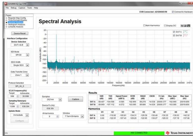
图 21. ADC AC Performance With Gain of 10 at 20 kHz (Same Gain on Both Channels)
