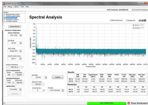
图 23. ADC Performance With Gain of 10 at 2 kHz (Same Gain on Both Channels)
