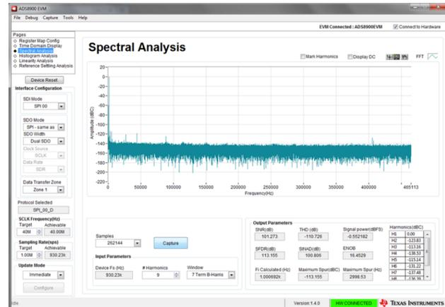
图 12. ADS8900B GUI Demonstrate AC Parameter—Spectral Analysis
