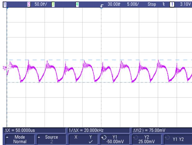
图 61. Output Voltage Ripple for -HV Output
