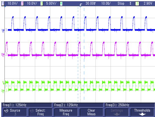
图 96. External SYNC Clock = 250 kHz (Channel 3 in Green)
