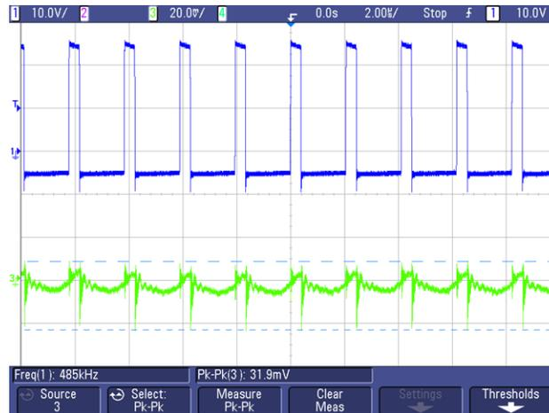
图 94. SW Node Waveform and Output Ripple for  $V_{OUT} = -5\text{ V}$ ,  $I_{OUT} = -1\text{ A}$
