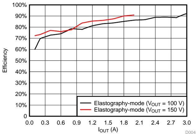
图 46. Elastography Mode Efficiency (+HV Output)
