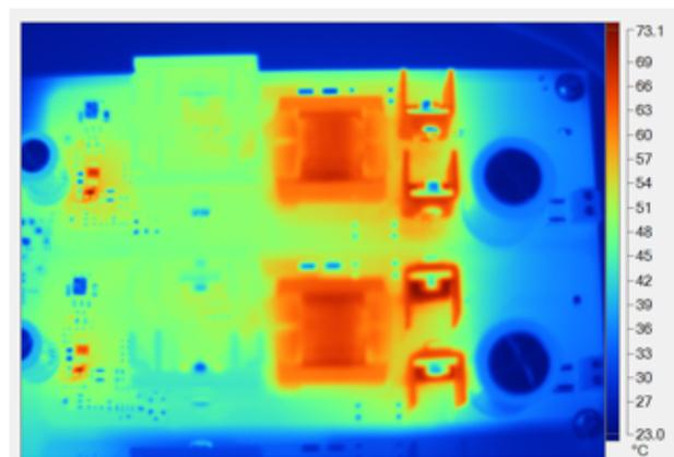
图 71. Thermal Image for  $\pm$ LV or MID Sections
