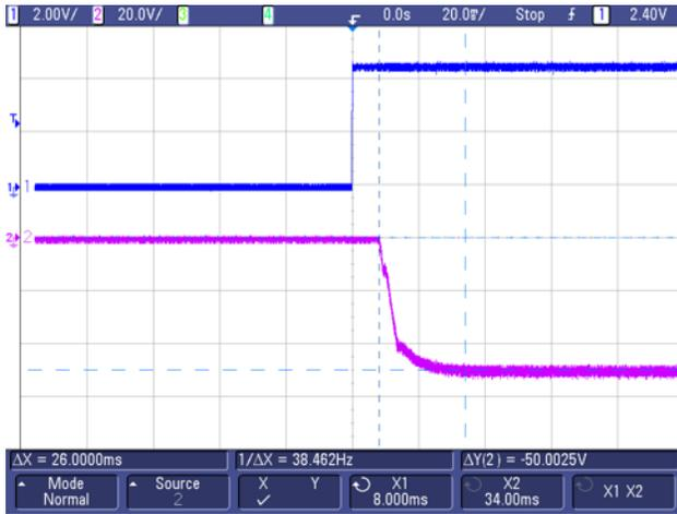
图 78. -LV/Mid-Out (Turnon) From 0 to -50 V at Full Load
