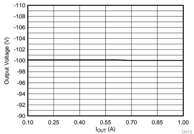
图 58. Load Regulation for  $V_{IN} = 24\text{ V}$ ,  $V_{OUT} = -100\text{ V}$
