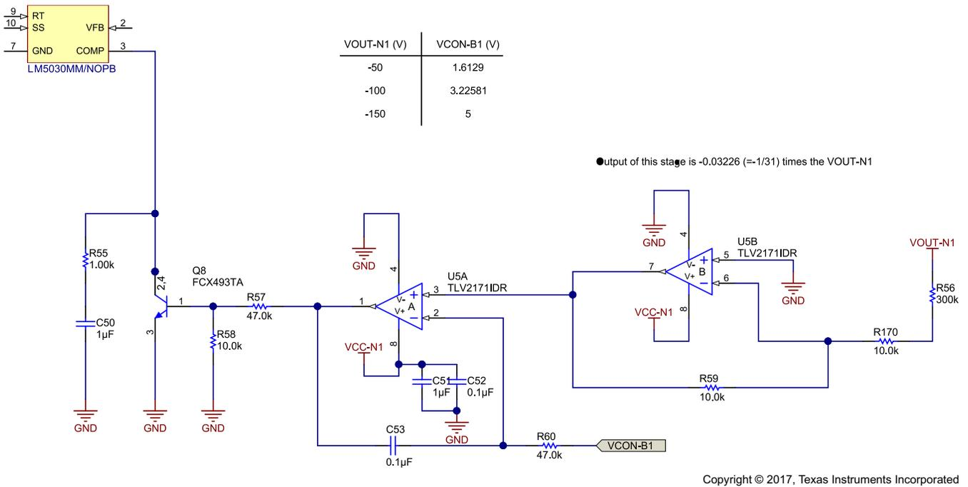
图 17. Feedback Circuit for Negative Rail for HV Section
