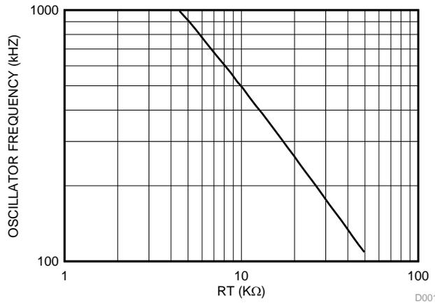
图 9. LM5030 Oscillator Frequency versus RT
