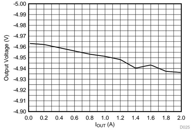
图 91. Load Regulation at  $V_{IN} = 24\text{ V}$ ,  $V_{OUT} = -5\text{ V}$
