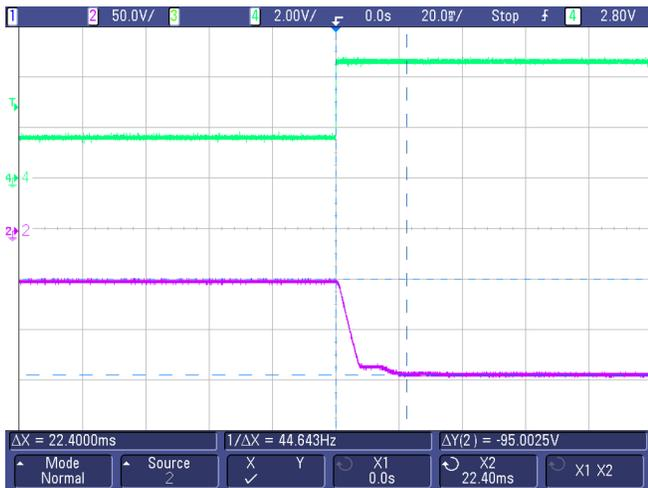
图 74. -HV-Out (Turnon) From -50 to -150 V at Full Load
