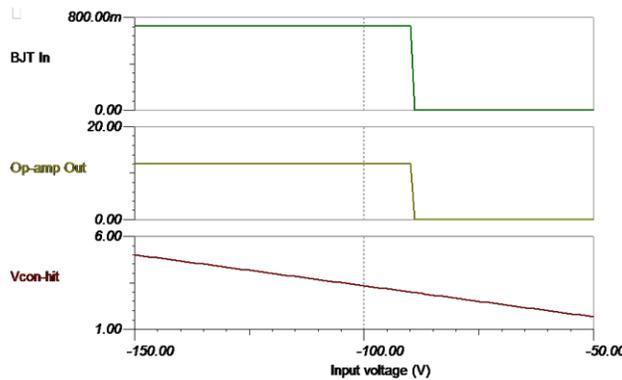
图 19. Simulation Waveform Showing Linearity (-HV Output)
