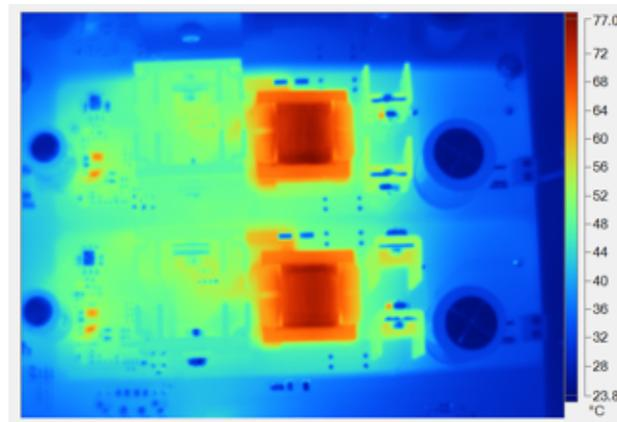
图 70. Thermal Image for  $\pm$ HV Sections
