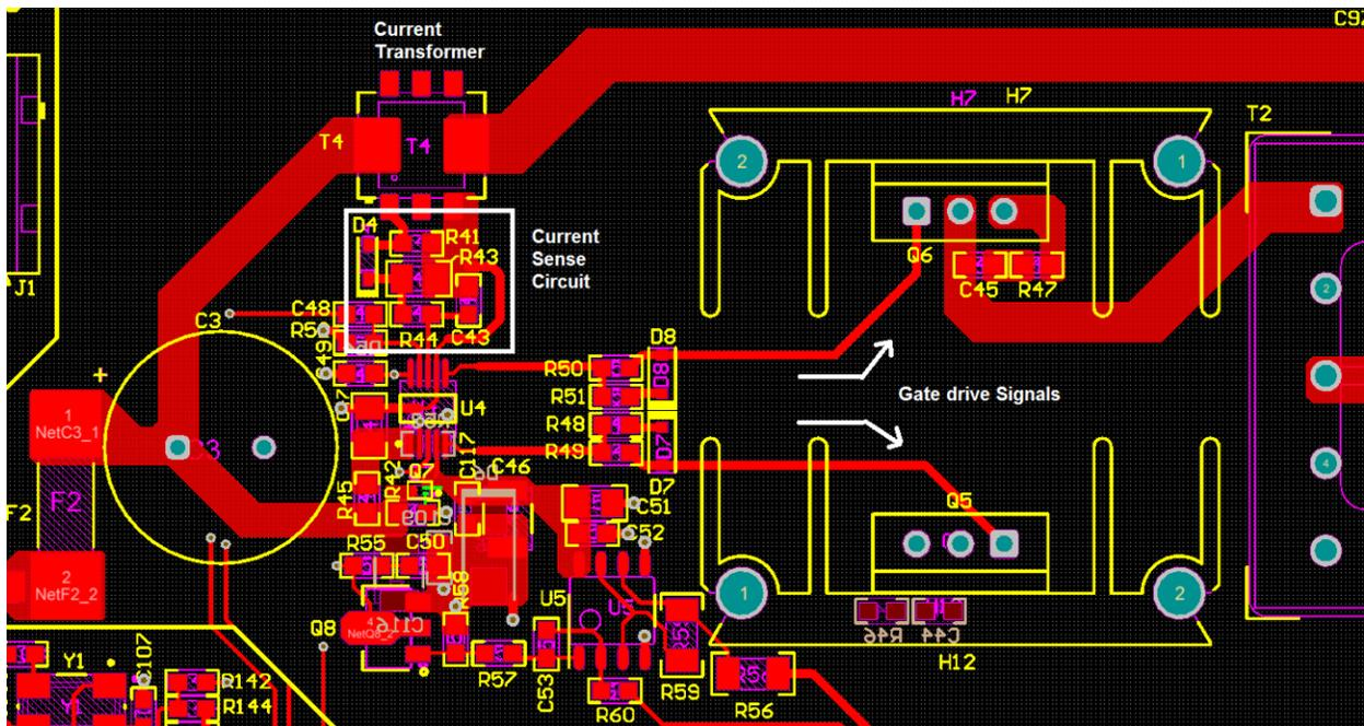
图 102. Routing for CS Pin for LM5030
