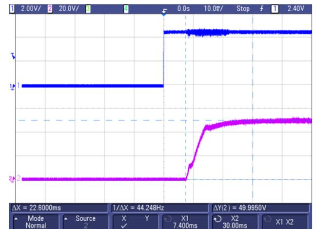
图 76. +LV/Mid-Out (Turnon) From 0 to 50 V at Full Load
