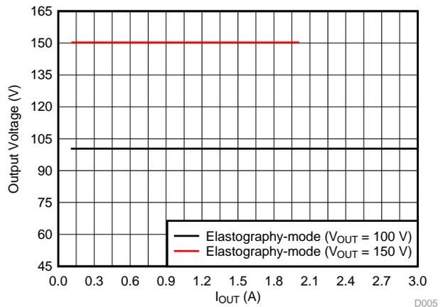
图 47. Elastography Mode Load Regulation (+HV Output)
