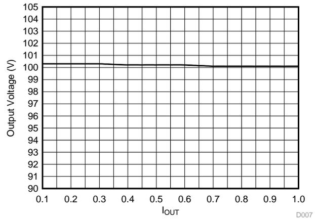
图 49. Load Regulation for  $V_{IN} = 24\text{ V}$ ,  $V_{OUT} = 100\text{ V}$
