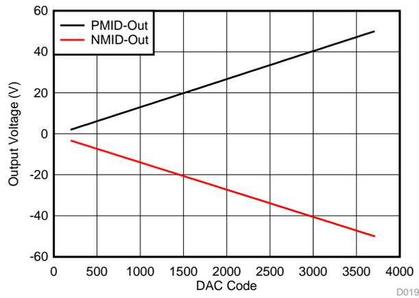
图 69. Output Voltage Linearity for U12 With Respect to Digital Input Code
