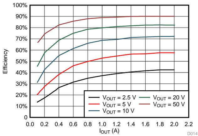
图 62. Efficiency for +LV or MID Section for CW Mode
