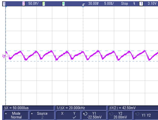
图 64. Output Voltage Ripple for +LV or MID Output at Full load
