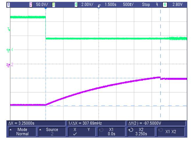
图 75. -HV-Out (Turnoff) From -150 to -50 V at Full Load
