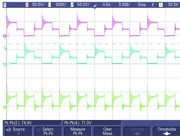
图 51. MOSFET Stress VDS for +HV Output
