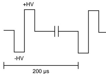
图 6. Three-Level Pulser Output Waveform
