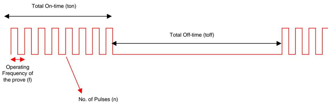
图 43. Load Profile for Testing TIDA-01352 in Different Imaging Modes
