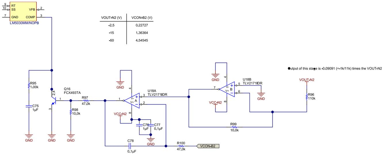
图 23. Feedback Circuit for Negative Rail for LV or MID Section
