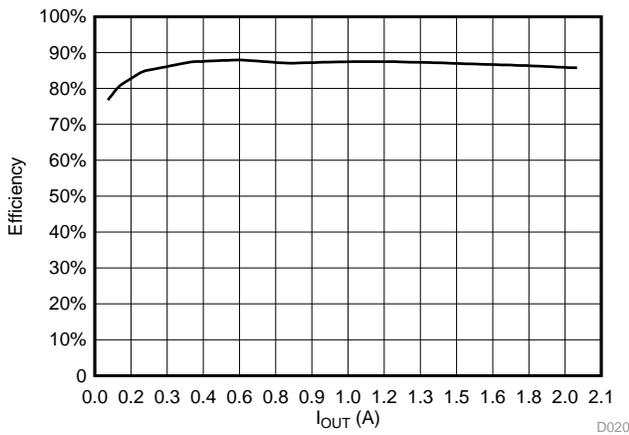
图 80. Efficiency at  $V_{IN} = 24\text{ V}$ ,  $V_{OUT} = 5\text{ V}$ ,  $I_{OUT} = 2\text{ A}$
