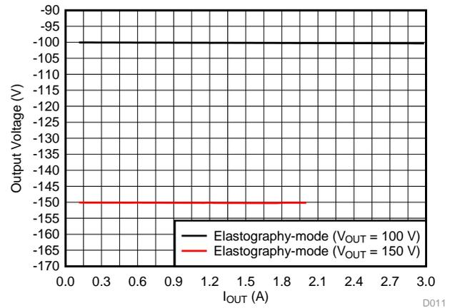
图 56. Elastography Mode Load Regulation (-HV Output)
