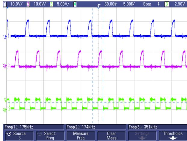
图 98. External SYNC Clock = 350 kHz (Channel 3 in Green)
