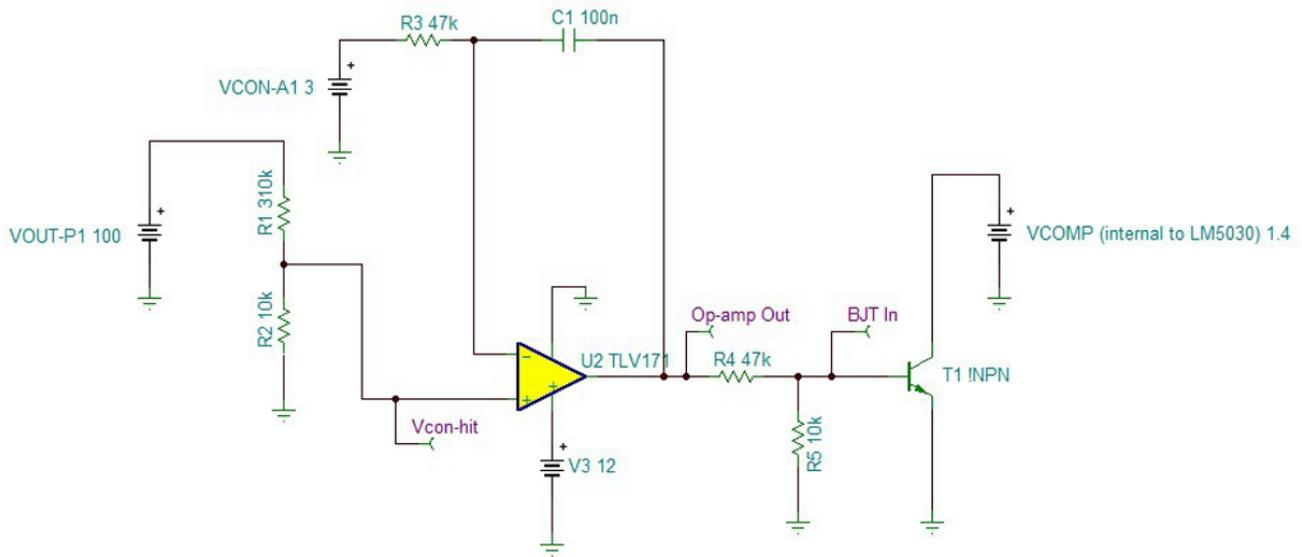
图 15. TINA Simulation for Feedback Circuit for Positive Rail for HV Section
