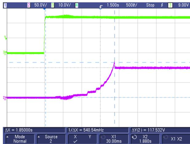
图 50. Start-up Waveform for +HV Output
