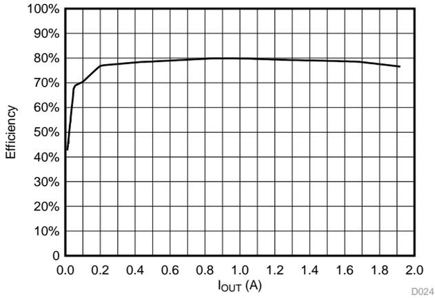
图 90. Efficiency at  $V_{IN} = 24\text{ V}$ ,  $V_{OUT} = -5\text{ V}$ ,  $I_{OUT} = -2\text{ A}$
