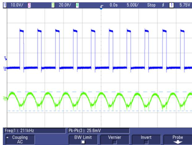
图 84. SW Node Waveform and Output Ripple for  $V_{OUT} = 5\text{ V}$ ,  $I_{OUT} = 1\text{ A}$
