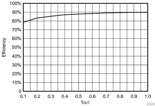
图 48. Full Load Efficiency at  $V_{IN} = 24\text{ V}$ ,  $V_{OUT} = 100\text{ V}$ ,  $I_{OUT} = 1\text{ A}$
