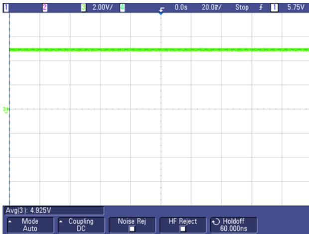
图 82.  $V_{OUT} = 5\text{ V}$  at  $V_{IN} = 24\text{ V}$
