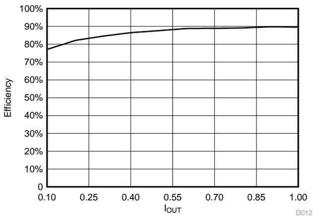
图 57. Full Load Efficiency at  $V_{IN} = 24\text{ V}$ ,  $V_{OUT} = -100\text{ V}$ ,  $I_{OUT} = -1\text{ A}$
