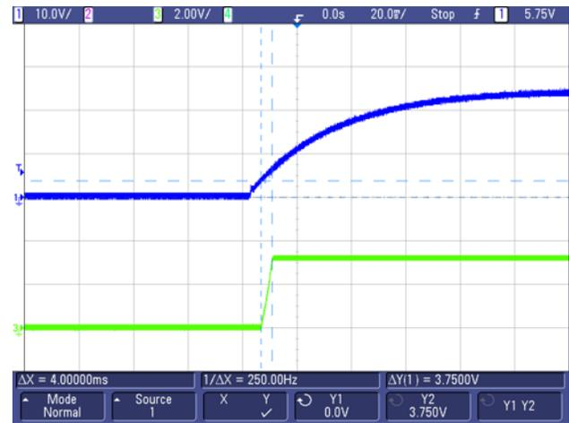
图 88. Start-up Waveform (for  $V_{OUT} = 3.3\text{ V}$ ) Showing Soft-Start Time = 4 ms
