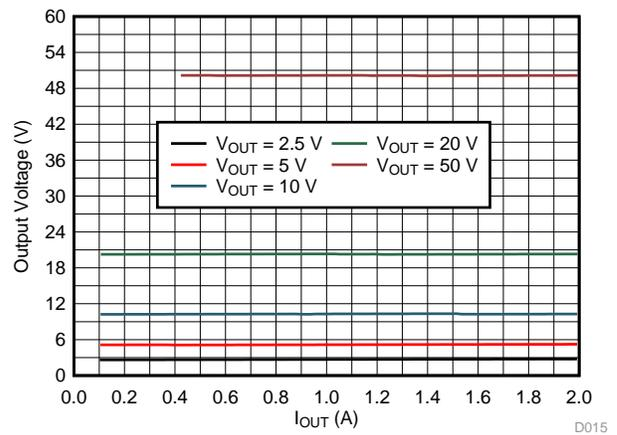
图 63. Load Regulation for +LV or MID Section for CW Mode
