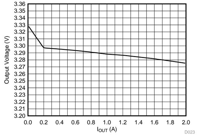
图 86. Load Regulation at  $V_{IN} = 24\text{ V}$ ,  $V_{OUT} = 3.3\text{ V}$
