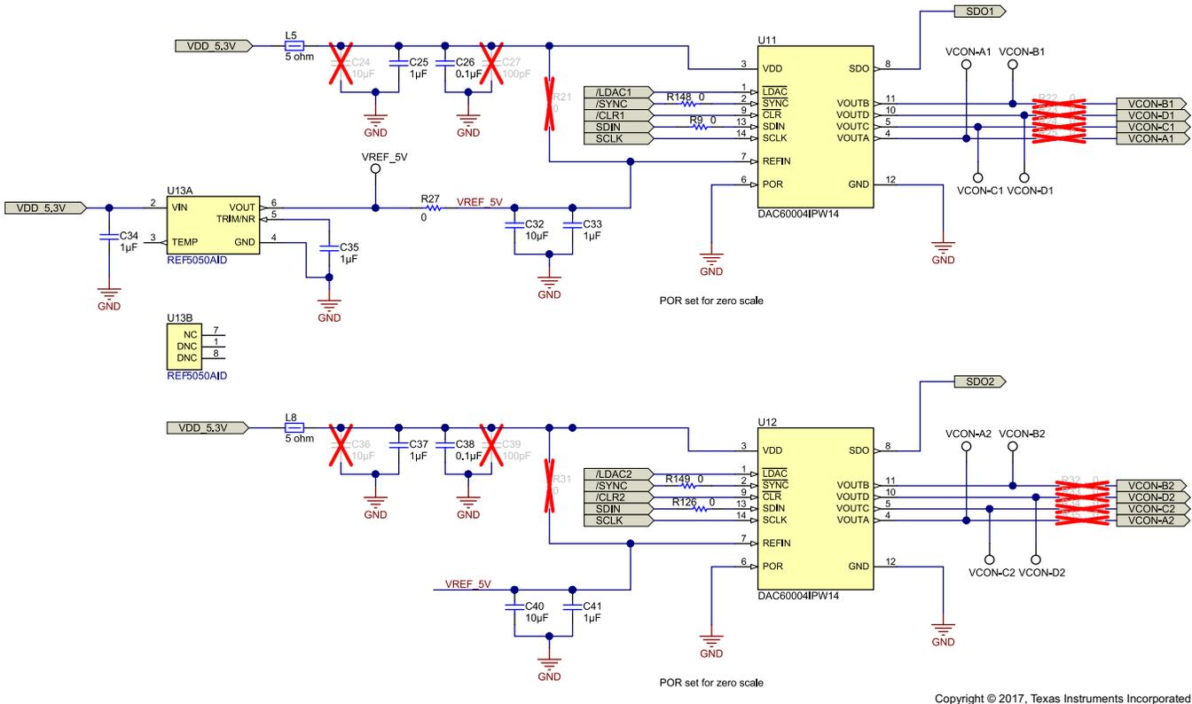
图 26. DAC60004 to set up Outputs for Power Supplies
