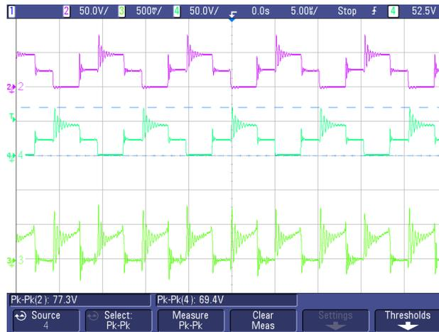
图 60. MOSFET Stress VDS for -HV Output
