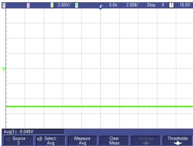
图 92.  $V_{OUT} = -5\text{ V}$  at  $V_{IN} = 24\text{ V}$
