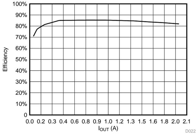
图 85. Efficiency at  $V_{IN} = 24\text{ V}$ ,  $V_{OUT} = 3.3\text{ V}$ ,  $I_{OUT} = 2\text{ A}$
