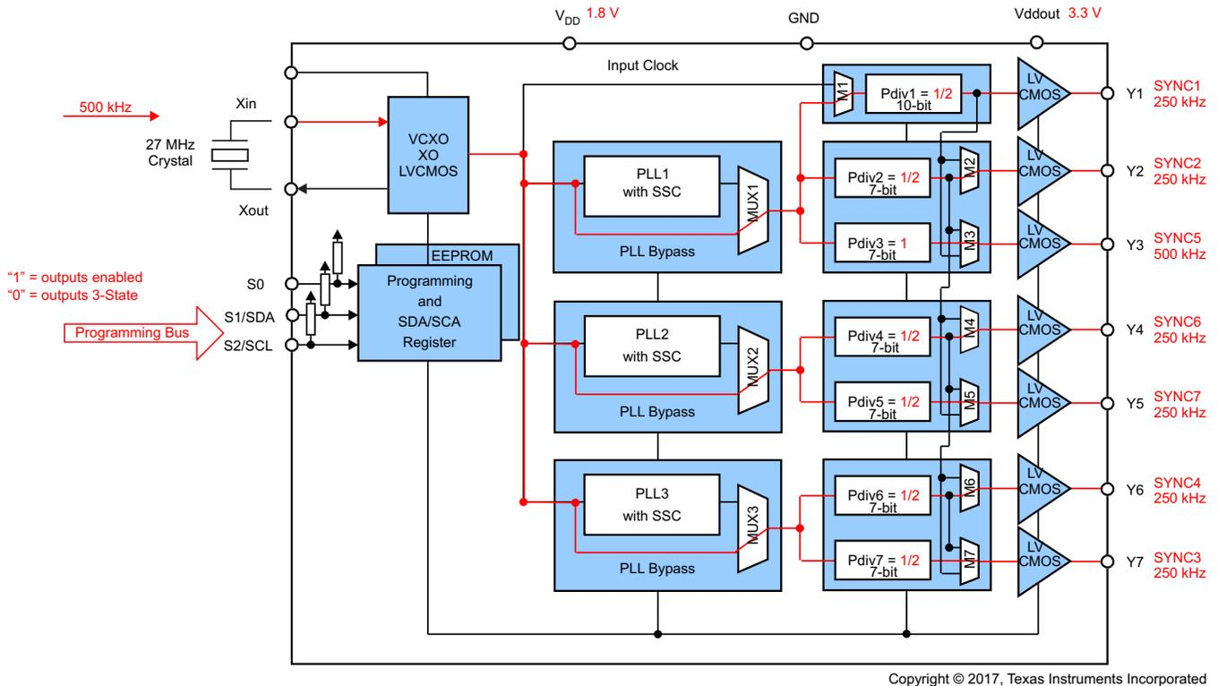
图 42. Clock Programming for Synchronization of All Devices to  $f_{IN} = 500 \text{ kHz}$
