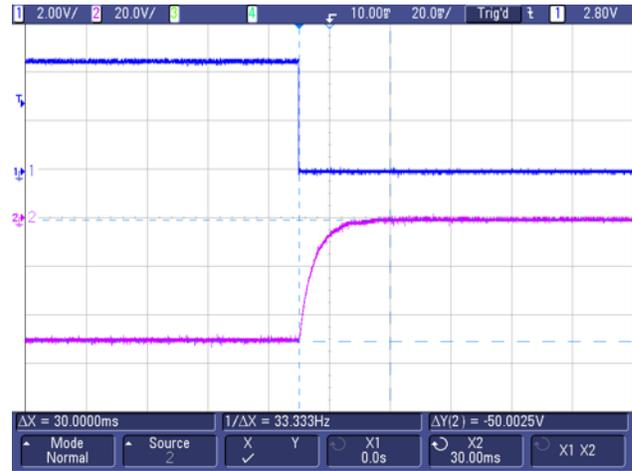
图 79. -LV/Mid-Out (Turnoff) from -50 to 0 V at Full Load
