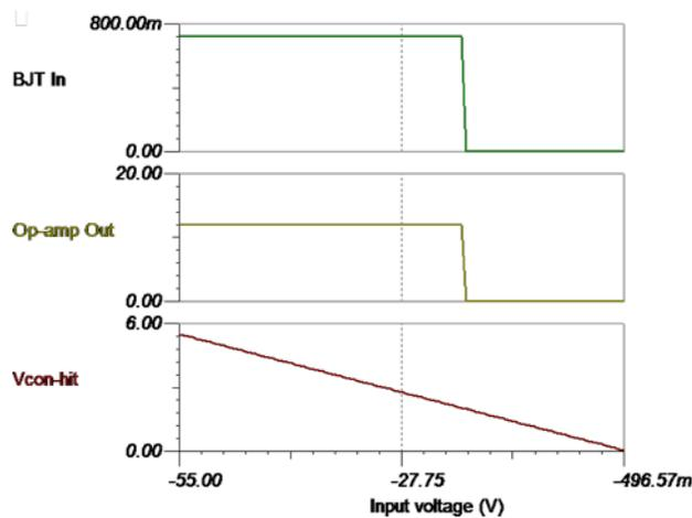
图 25. Simulation Waveform Showing Linearity (+LV or MID Output)
