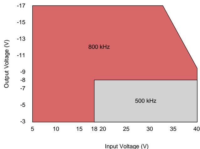
图 32. Recommended Switching Frequency for LMZ34002
