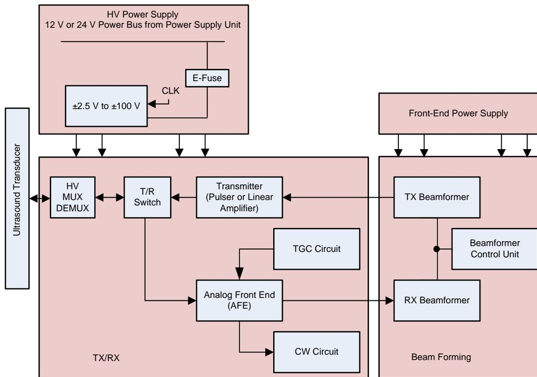
图 2. System Level Block Diagram for Cart-Based Ultrasound Scanners (Full Block Diagram Not Shown)
