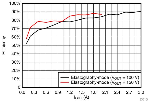
图 55. Elastography Mode Efficiency (-HV Output)
