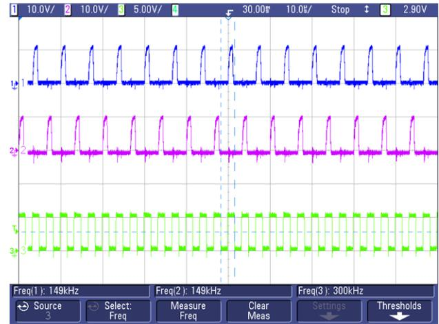
图 97. External SYNC Clock = 300 kHz (Channel 3 in Green)
