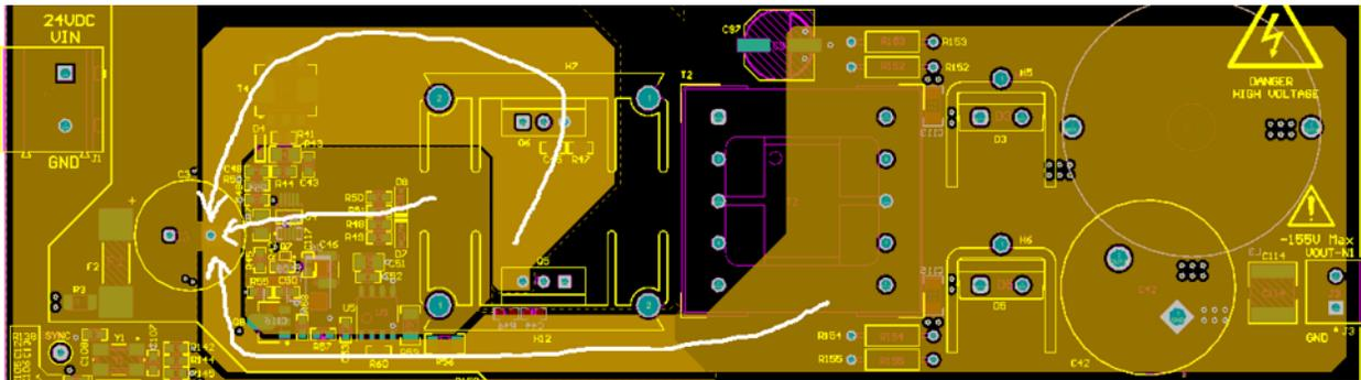
图 101. Star Ground Topology for Power Supply
