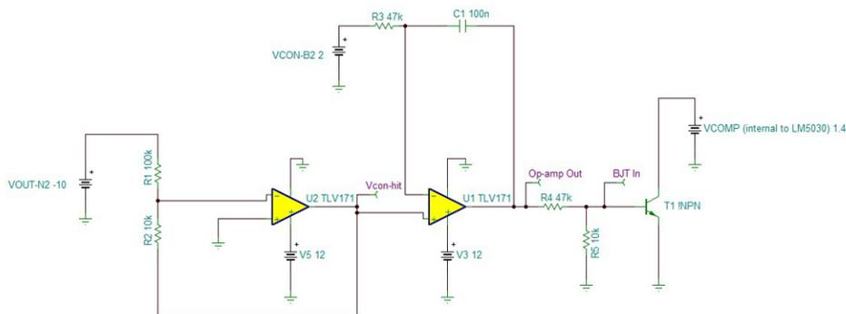
图 24. TINA Simulation for Feedback Circuit for Negative Rail for LV or MID Section
