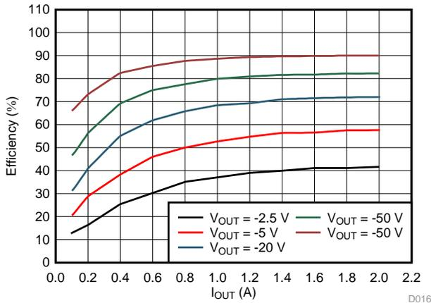
图 65. Efficiency for -LV or MID Section for CW Mode
