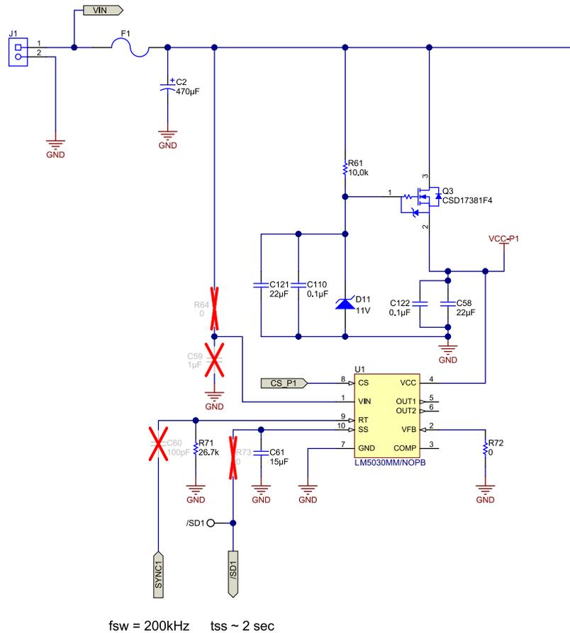
图 8. Input Section and Turnon Mechanism for LM5030
