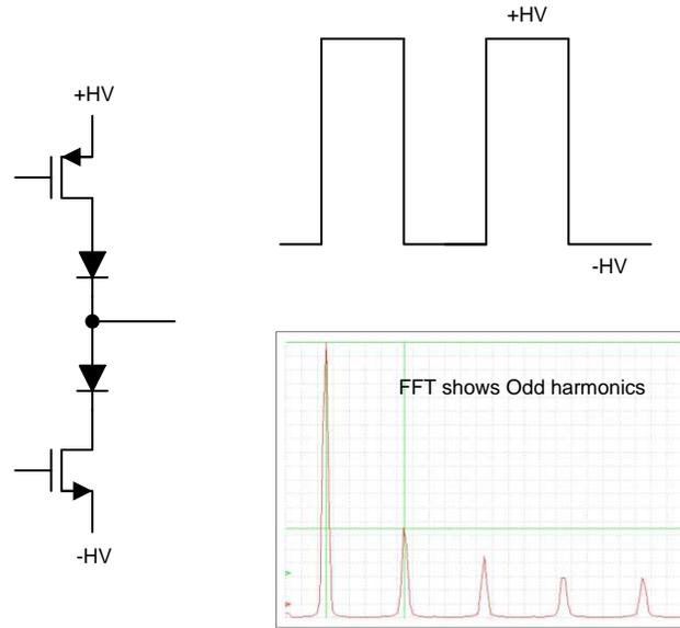
图 4. Pulser—Output Waveform and FFT of Output
