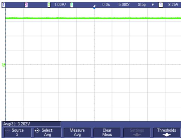
图 87.  $V_{OUT} = 3.3\text{ V}$  at  $V_{IN} = 24\text{ V}$
