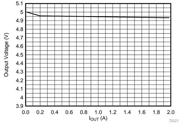
图 81. Load Regulation at  $V_{IN} = 24\text{ V}$ ,  $V_{OUT} = 5\text{ V}$
