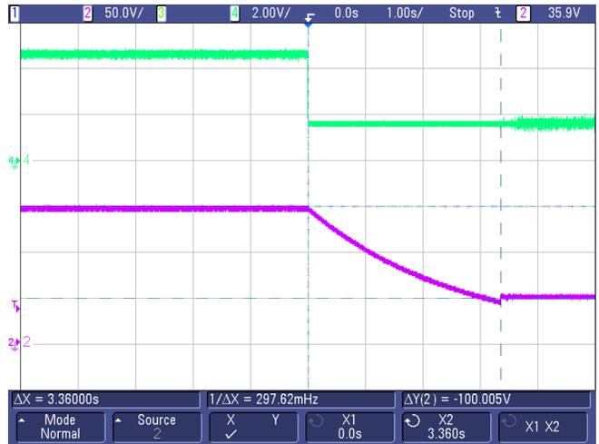
图 73. +HV-Out (Turnoff) From 150 to 50 V at Full Load
