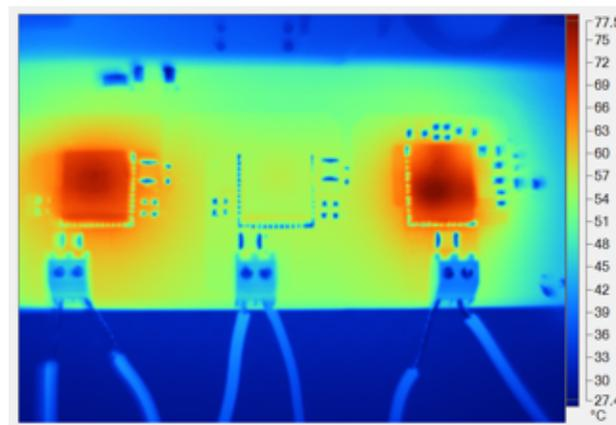
图 95. Thermal Image for LMZ Modules at Full Load
