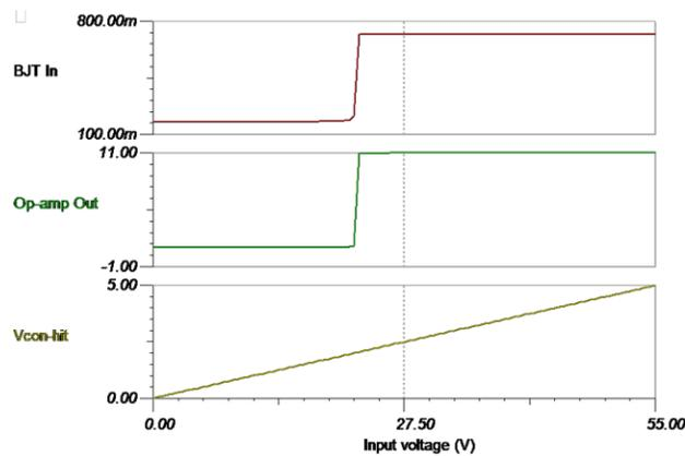
图 22. Simulation Waveform Showing Linearity (+LV or MID Output)
