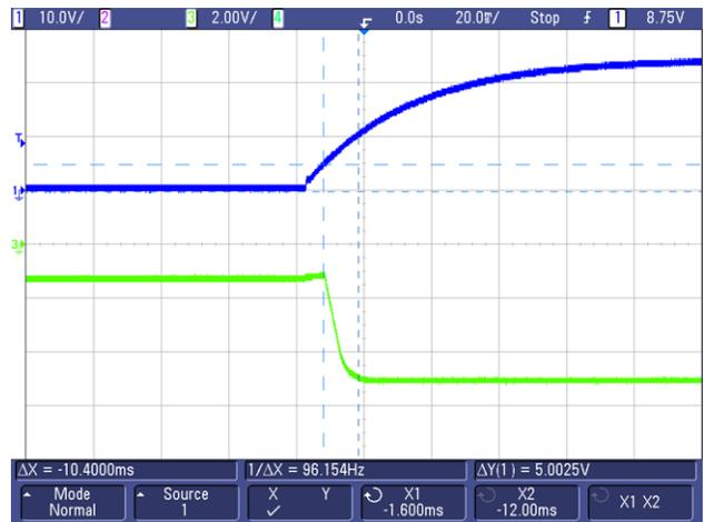
图 93. Start-up Waveform (for  $V_{OUT} = -5\text{ V}$ ) Showing Soft-Start Time = 10.4 ms
