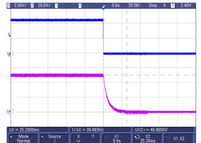
图 77. +LV/Mid-Out (Turnoff) From 50 to 0 V at Full Load
