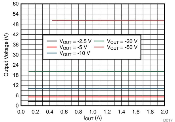
图 66. Load Regulation for -LV or MID Section for CW Mode
