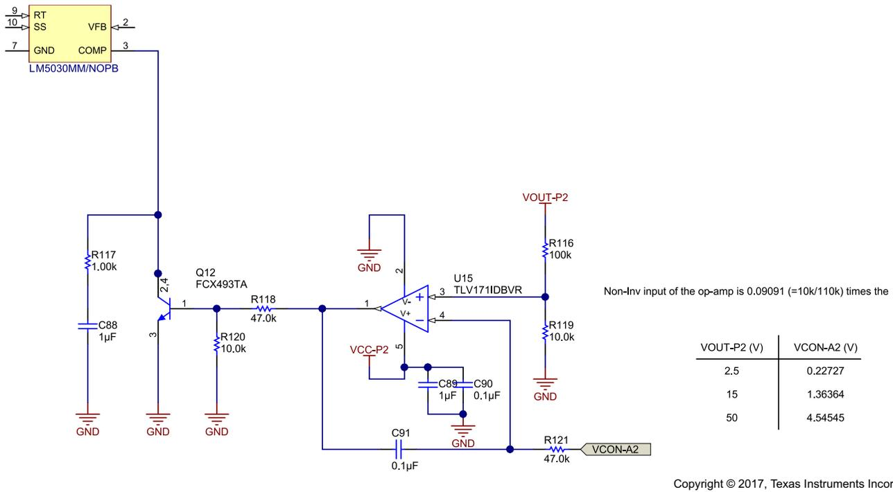
图 20. Feedback Circuit for Positive Rail for LV or MID Section
