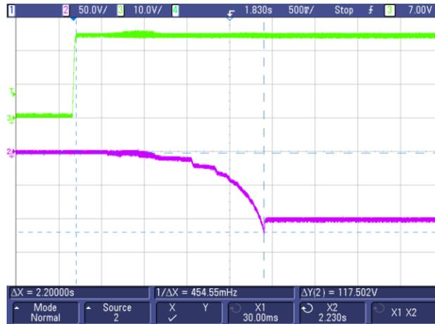
图 59. Start-up Waveform for -HV Output
