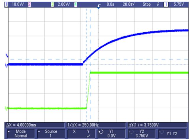
图 83. Start-up Waveform (for  $V_{OUT} = 5\text{ V}$ ) Showing Soft-Start Time = 4 ms
