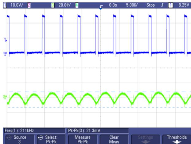
图 89. SW Node Waveform and Output Ripple for  $V_{OUT} = 3.3\text{ V}$ ,  $I_{OUT} = 1\text{ A}$
