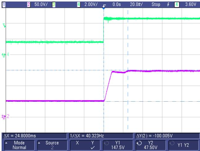
图 72. +HV-Out (Turnon) From 50 to 150 V at Full Load
