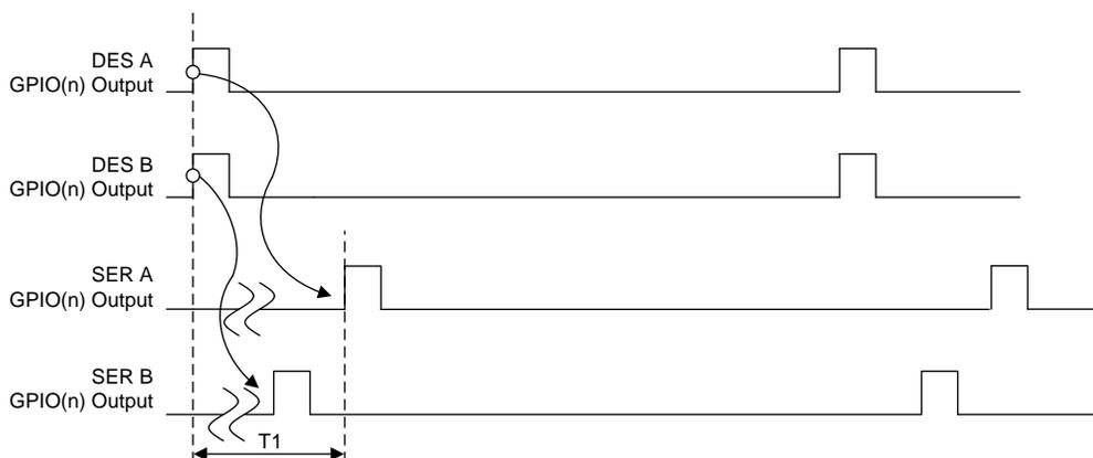
图 9. GPIO Maximum Latency
