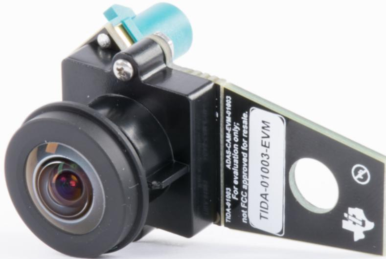
图 11. TIDA-01003 Completed Assembly
