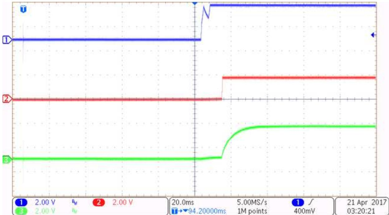
图 16. Power-up Sequence Waveform
