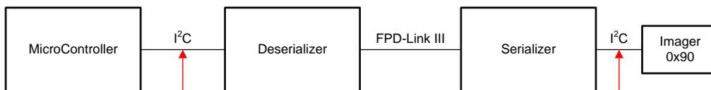
图 14. Setup for Monitoring I<sup>2</sup>C Transactions
