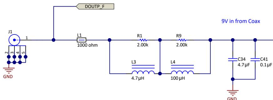
图 6. Power Over Coax Schematic
