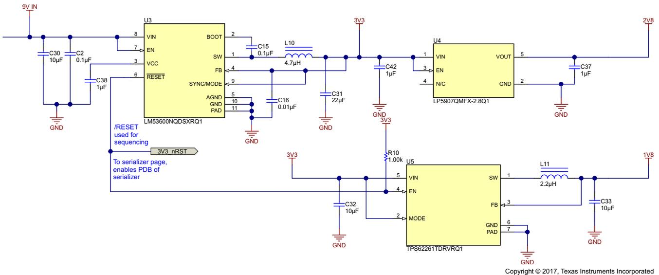
图 4. Power Supply Schematic
