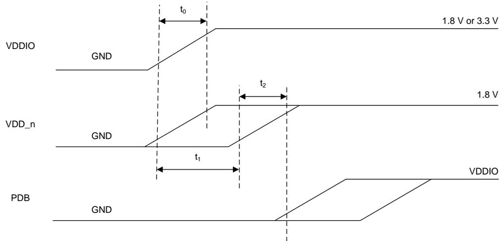
图 15. Target Power-up Sequence
