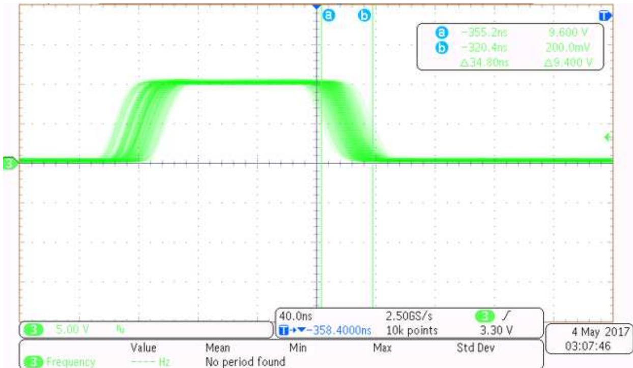
图 19. Spread Spectrum Operation
