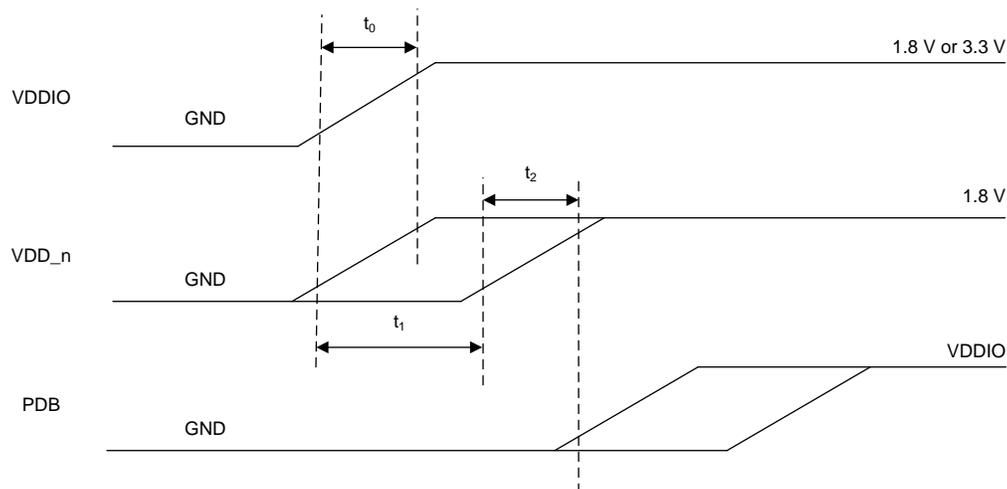
图 10. Target Power-up Sequence
