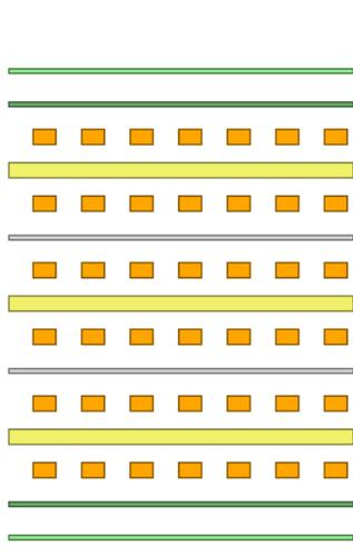
The diagram shows a cross-section of a 12-layer PCB stackup. From top to bottom, the layers are: Top Overlay (green), Top Solder (green), Layer 1 - Top Layer (orange), Dielectric 1 (yellow), Layer 2 - GND (orange), Dielectric 2 (yellow), Layer 3 - Signal (orange), Dielectric 3 (yellow), Layer 4 - Power (orange), Dielectric 4 (yellow), Layer 5 - GND (orange), Dielectric 5 (yellow), Layer 6 - Bottom Layer (orange), Bottom Solder (green), and Bottom Overlay (green).
