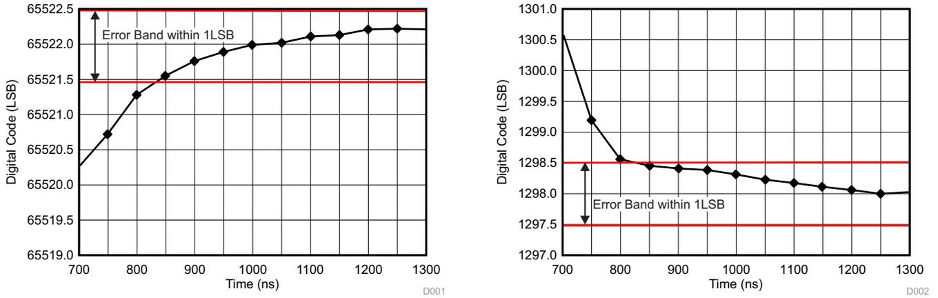
图 1. Measurement Result of Settling Time Plot for Multiplexed Data Acquisition Block<sup>(1)</sup>
