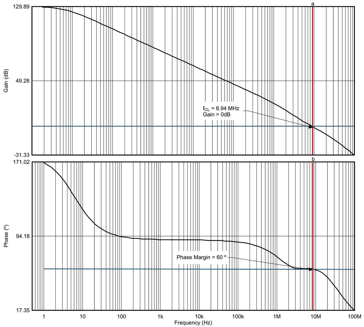
图 23. TINA-TI™ Simulation Result—Loop Gain Magnitude and Phase Plot for Input Driver Stability
