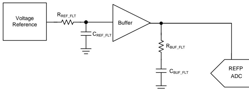
图 14. Block Diagram of Reference Driver
