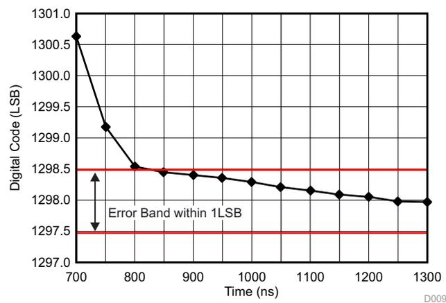
图 27. Measurement Data—Acquired Code in Different Settling Time for Falling Full-Scale Input
