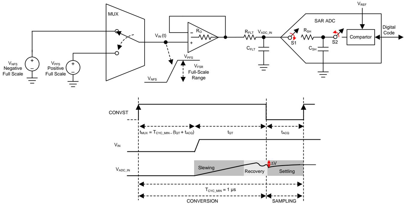
图 9. Timing Diagram of Settling Time in DAQ
