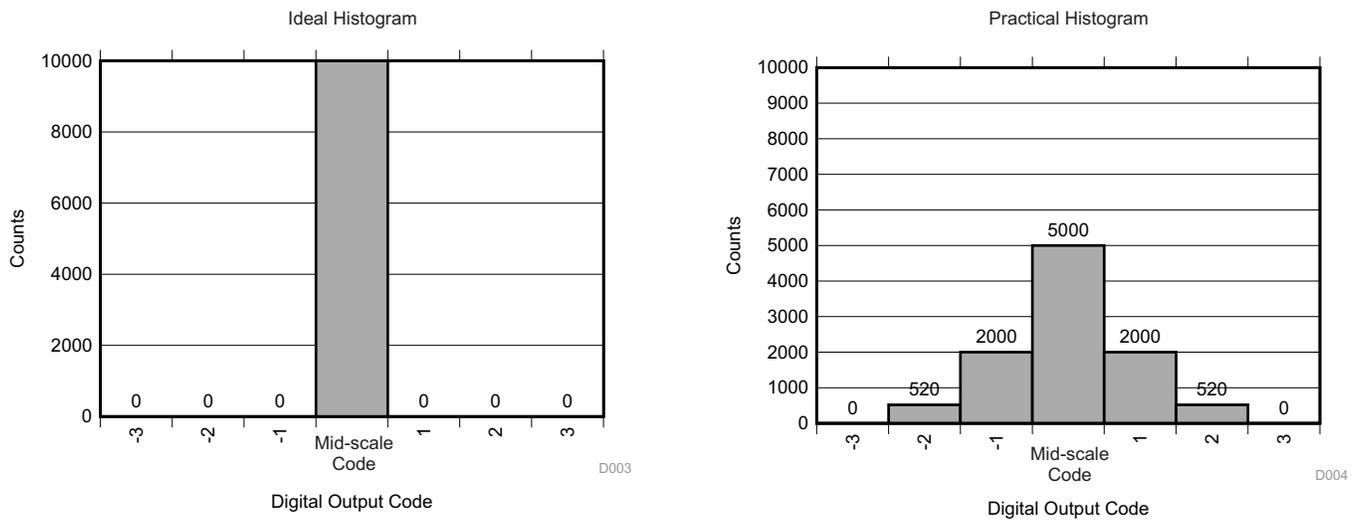
图 5. Histogram of ADC Output Codes for Constant Midscale DC Input
