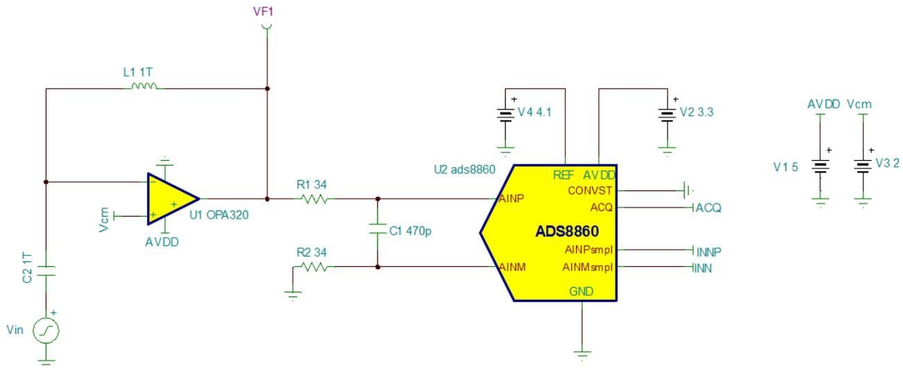
图 22. TINA-TI™ Schematic—Checking Input Amplifier Stability
