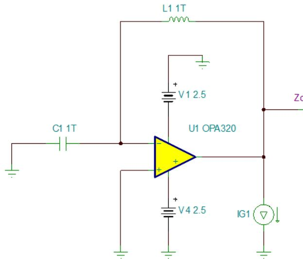
图 16. TINA-TI™ Schematic—Measuring Open-Loop Output Impedance of OPA320
