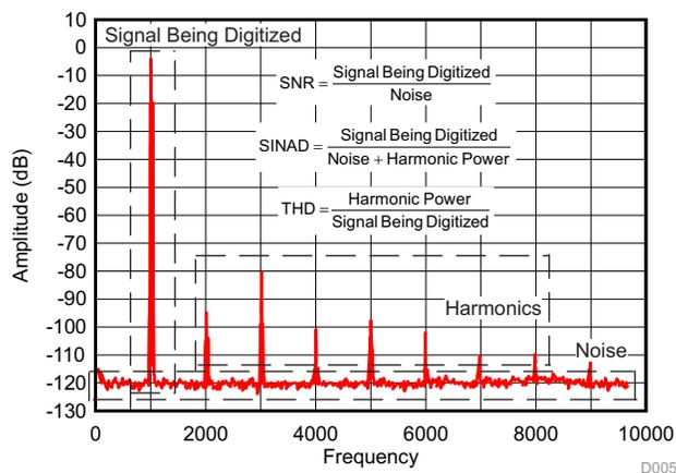
图 8. Dynamic Specifications of ADC
