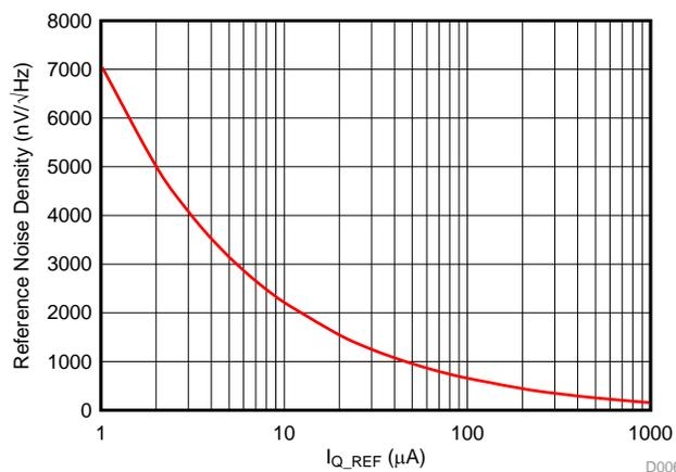
图 15. Characteristic Curve of Reference Noise versus Quiescent Current – Approximation of Noise Density for Band Gap References
