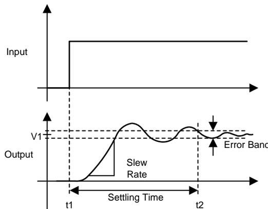
图 3. Definition of Settling Time
