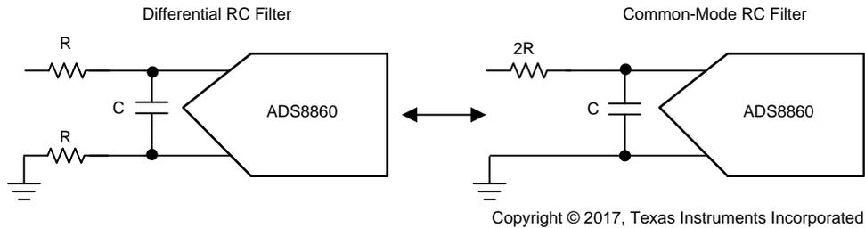
图 18. Design Configuration for Charge Bucket at ADC Input
