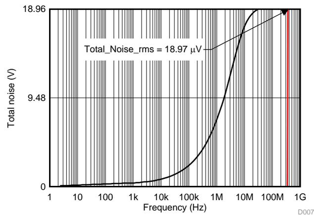
图 25. TINA-TI™ Simulation Result—Integrated Input Amplifier RMS Noise
