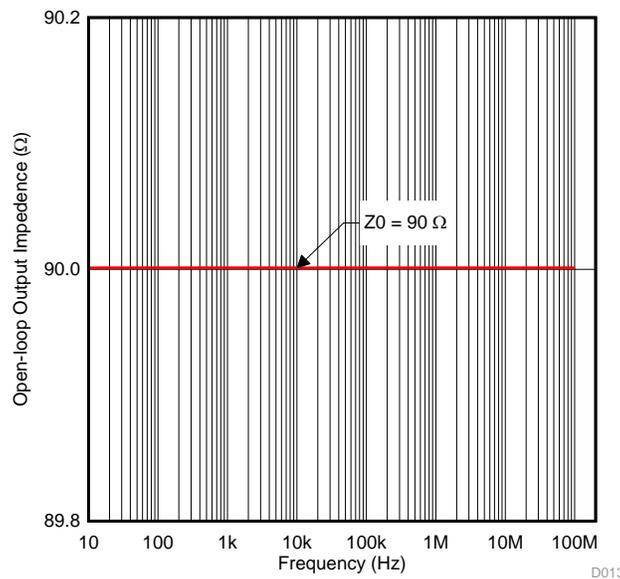
图 17. TINA-TI™ Simulation Result—Output Impedance of OPA320
