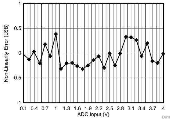
图 29. Measurement Data—ADC Linearity (26 Points)
