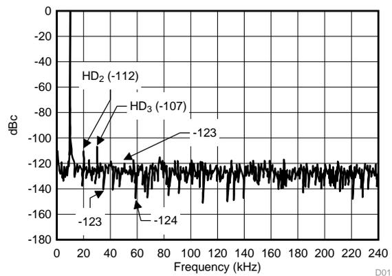
图 30. Measurement Data—FFT of DAQ Block
