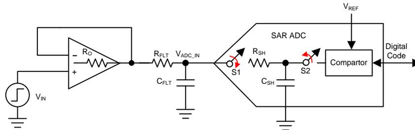
图 11. Simplified Schematic of Single-Ended ADC Input Stage
