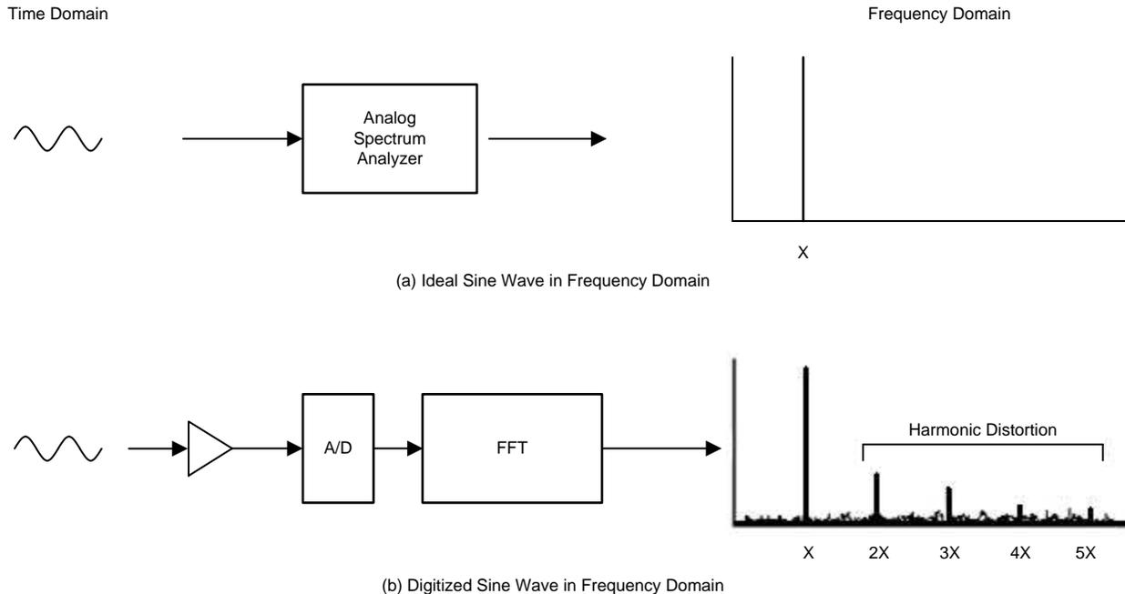
图 7. Comparison of (A) Ideal and (B) Digitized Sine Wave in Frequency Domain
