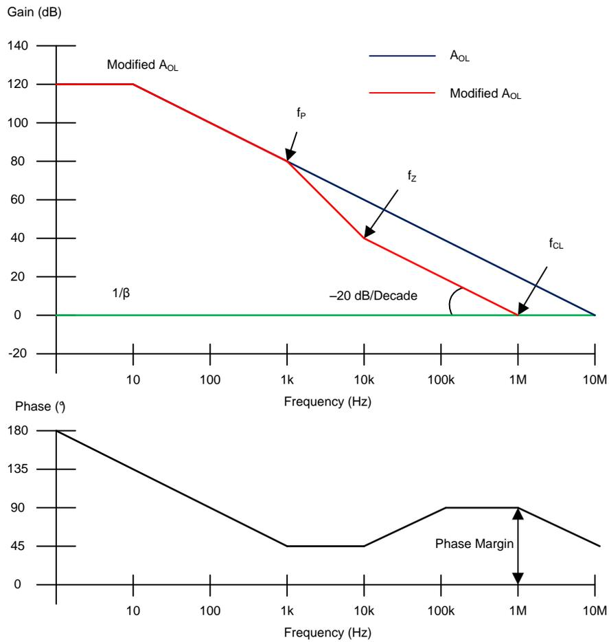
图 12. Analyzing Effect of RC-Filter on Op Amp Stability Using  $A_{OL}$  Response
