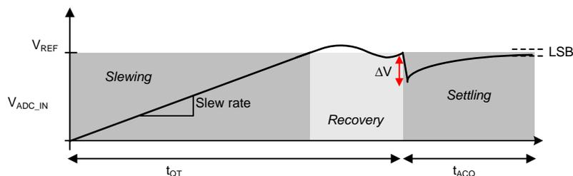
图 10. Typical Input Settling Time Response
