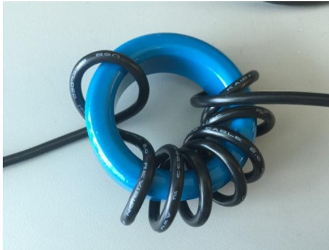
**图 17. USB Cable Around Ferrite Bead**
