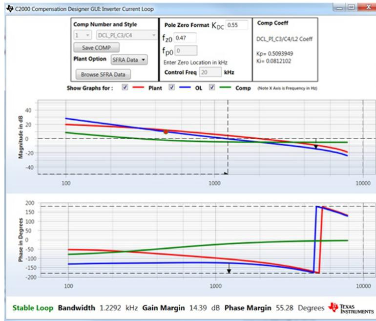
图 30. Compensation Designer With Measured Plant Frequency Response Data
