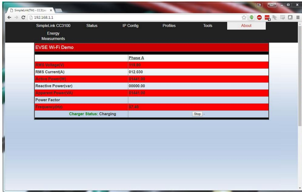
图 33. EVSE Web Page Showing Charging State
