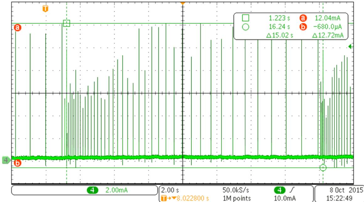
图 29. System Current Showing One Complete Transmit Cycle
