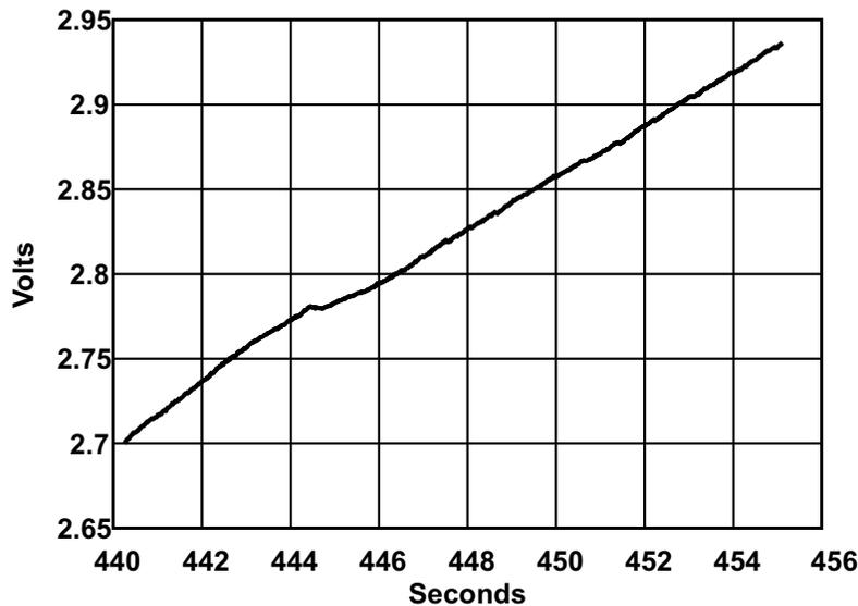
图 31. Voltage Rise Between Transmissions During Capacitor Reservoir Charging With 1000 Lux
