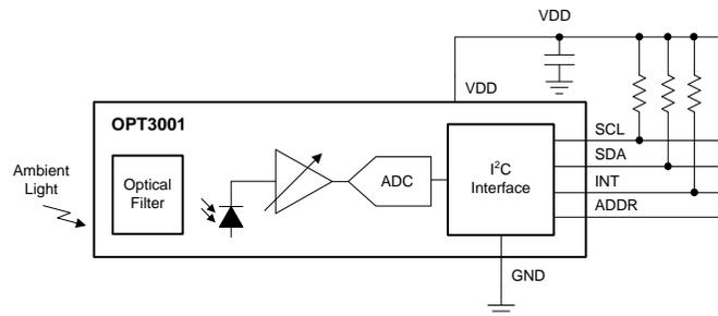
图 6. OPT3001 Functional Block Diagram
