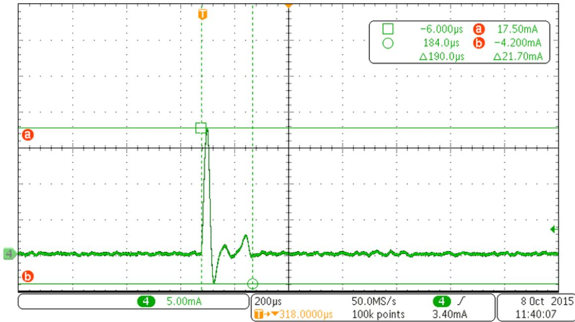
图 30. Current Transient During CC1310 Shutdown
