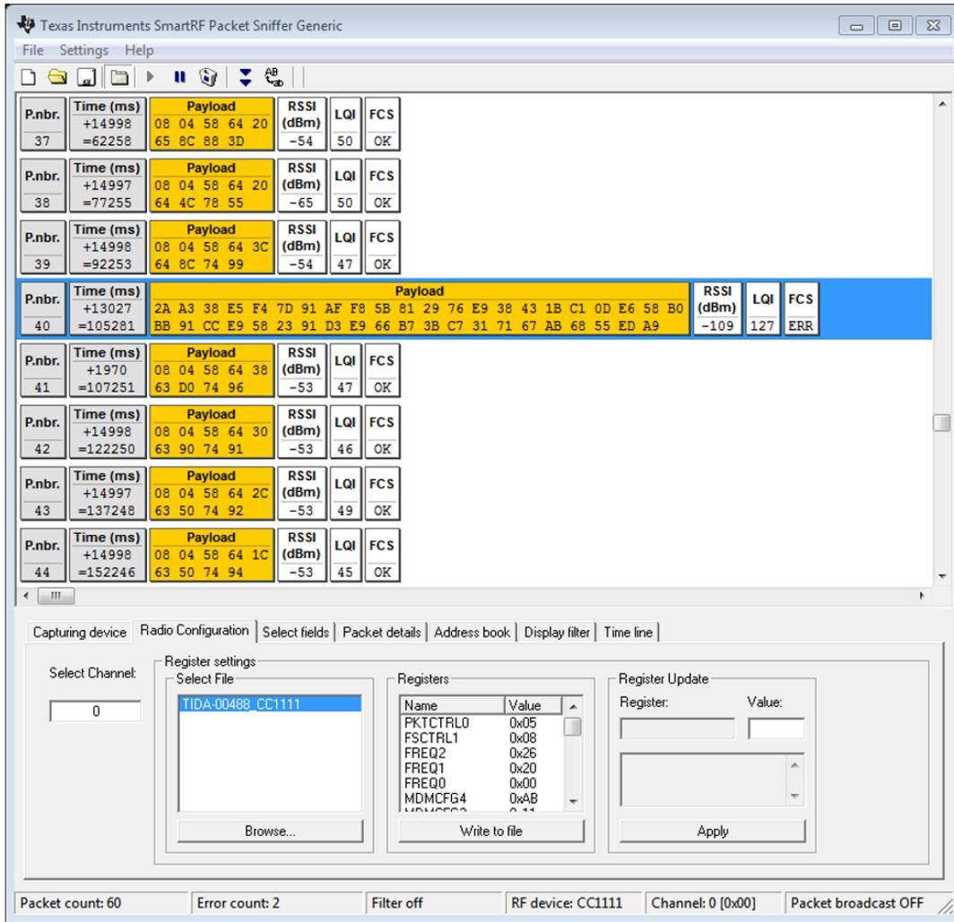
图 16. Unfiltered Radio Data
