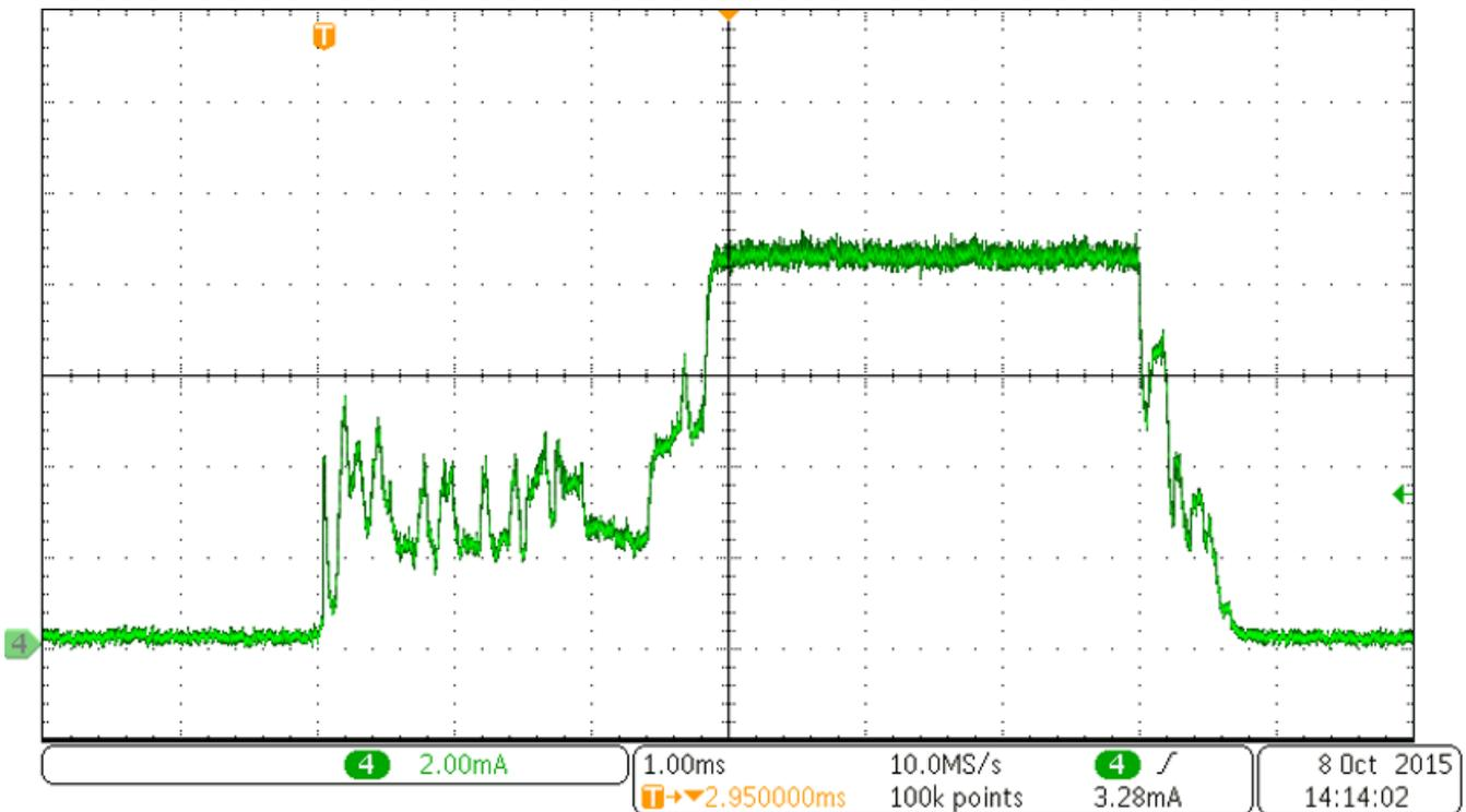
图 28. Light Sensor Data Read and RF Transmission
