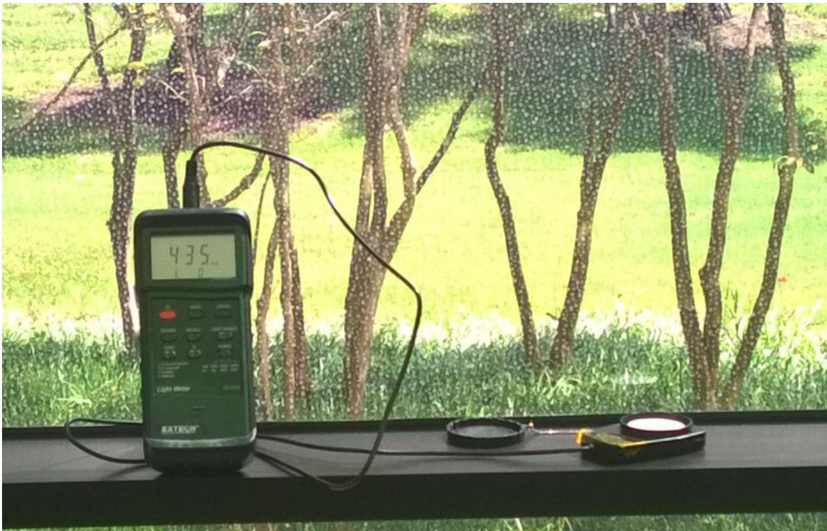
**图 18. Light Meter Measuring Light Level in a Sunny Window**
