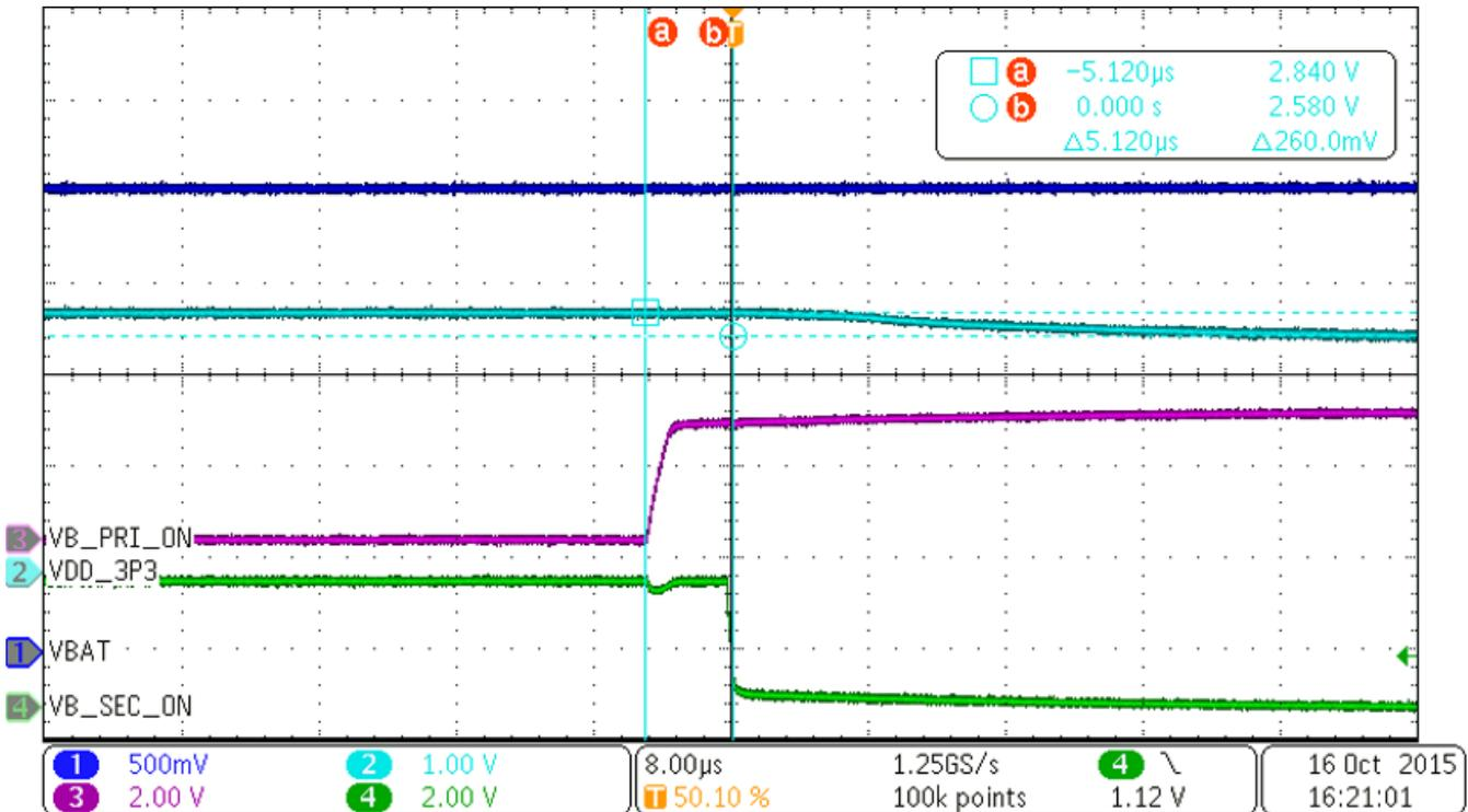
图 19. Power Transition From Primary Cell to the Capacitor Reservoir Charged by the Solar Cells
