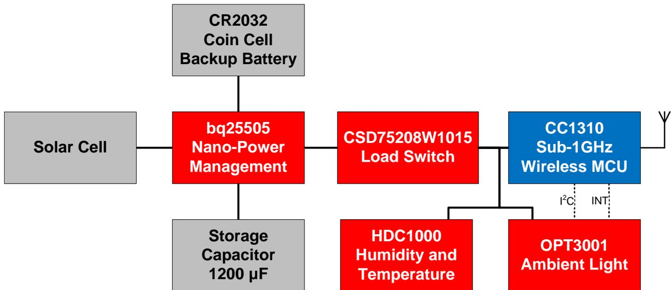
图 2. Energy Harvesting Ambient Light and Environment Sensor Node for Sub-1GHz Networks System Block Diagram
