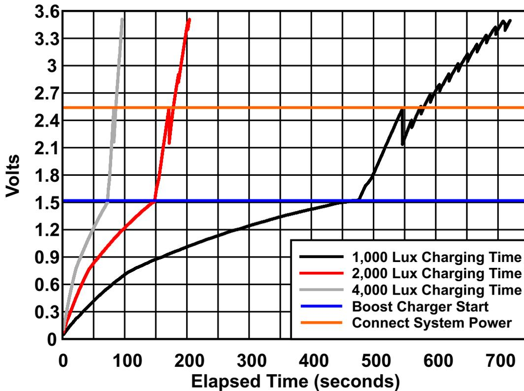
图 25. Voltage versus Time for the Capacitor Reservoir for Three Light Levels
