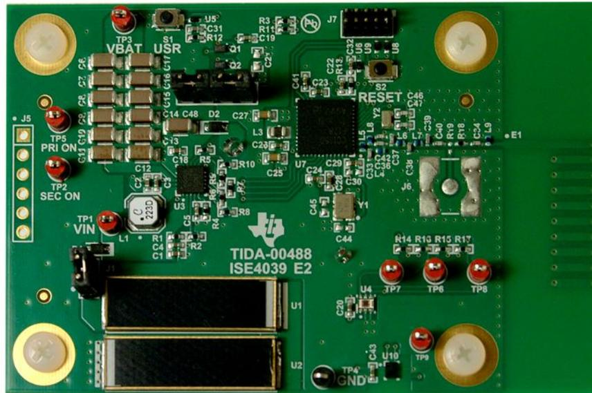
图 11. Energy Harvesting Ambient Light and Environment Sensor Node for Sub-1GHz Networks Reference Design Hardware
