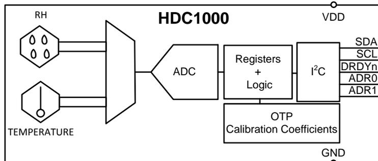
图 7. HDC1000 Functional Block Diagram
