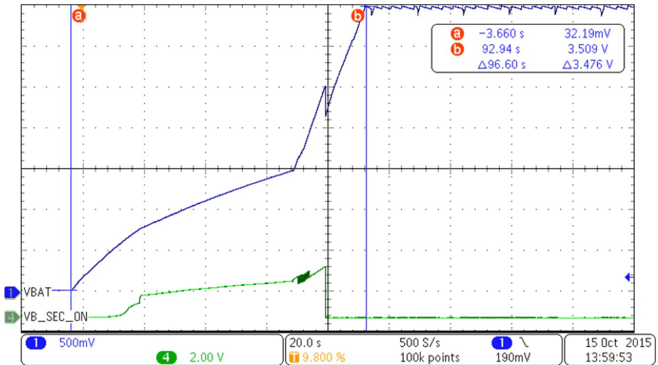
图 24. Capacitor Reservoir Charging Profile With 4,000 Lux Light Level
