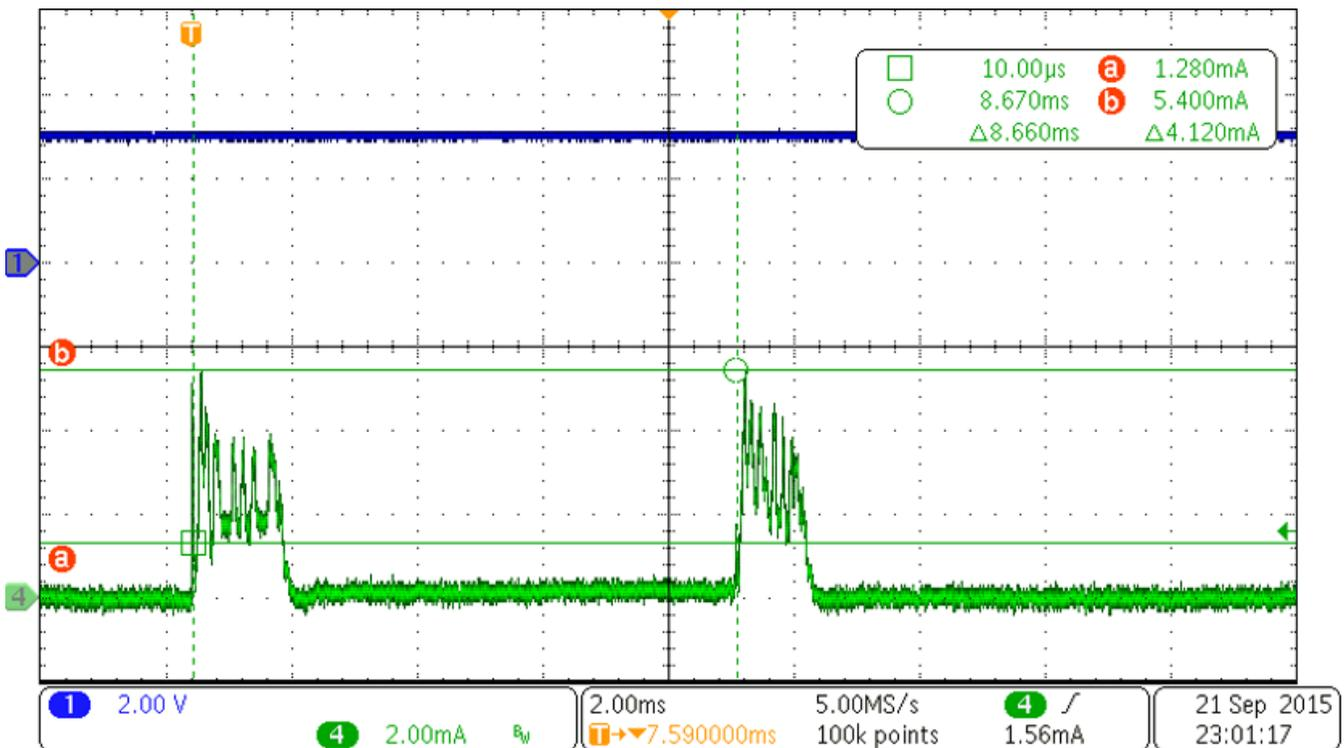
图 26. Current Profile During Conversion Trigger and Temperature-Humidity Sensor Read
