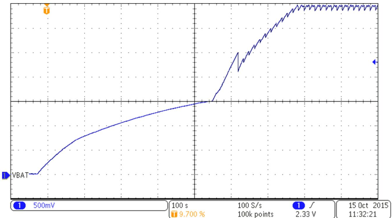
图 22. Capacitor Reservoir Charging Profile With 1,000 Lux Light Level
