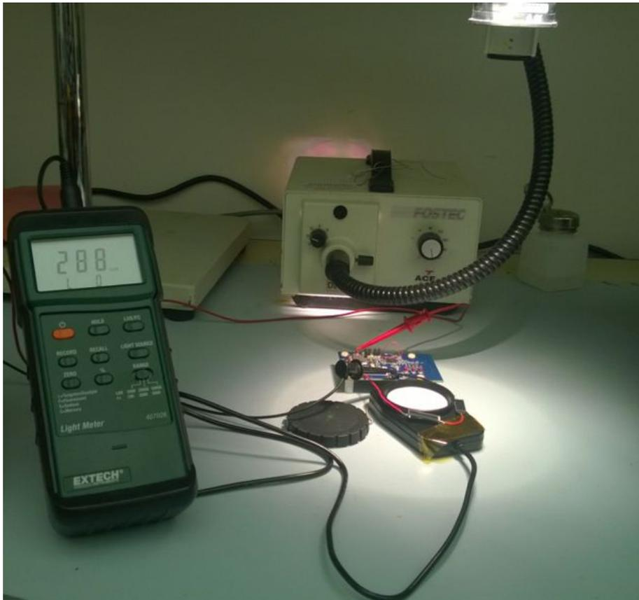
图 21. Light Measurement Setup With Microscope Light at 2880 Lux
