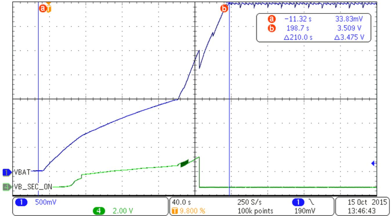
图 23. Capacitor Reservoir Charging Profile With 2,000 Lux Light Level
