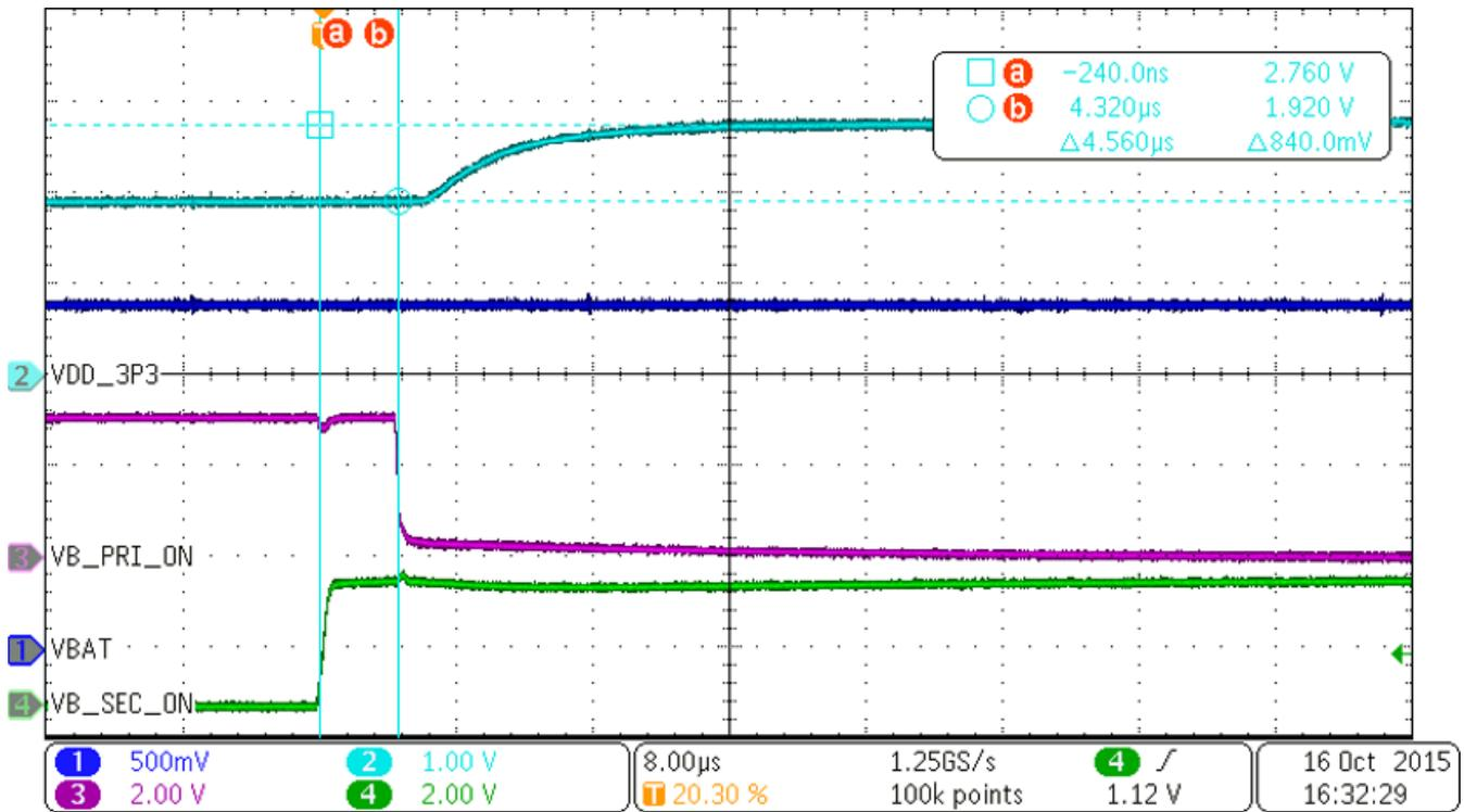
图 20. Power Transition From Primary Cell to the Capacitor Reservoir Charged by the Solar Cells
