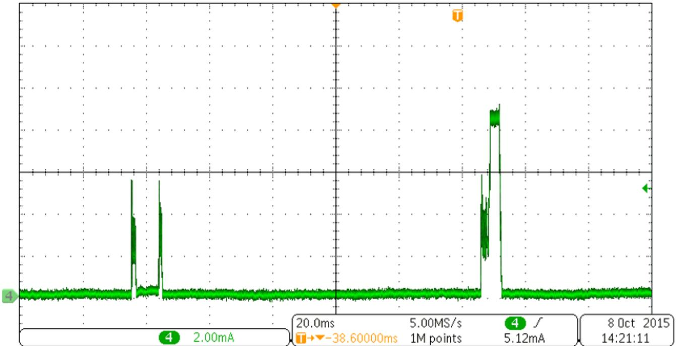
图 27. Current Profile of Sensor Data Conversions, Data Reads, and RF Transmission
