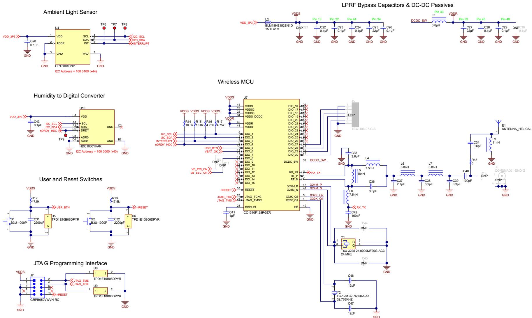
图 33. Bluetooth® and Light Sensing Schematic
