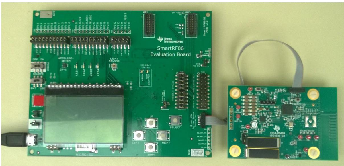
图 12. Connection of SmartRF06 Evaluation Board and TI Designs Hardware for Programming and Debugging
