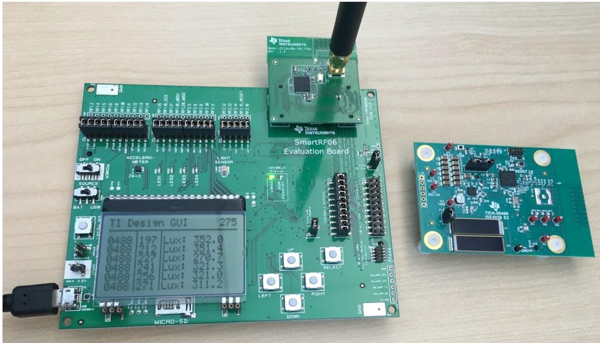
图 13. Sniffer Application Running on the SmartRF06 EVM With the CC13xxEM Radio
