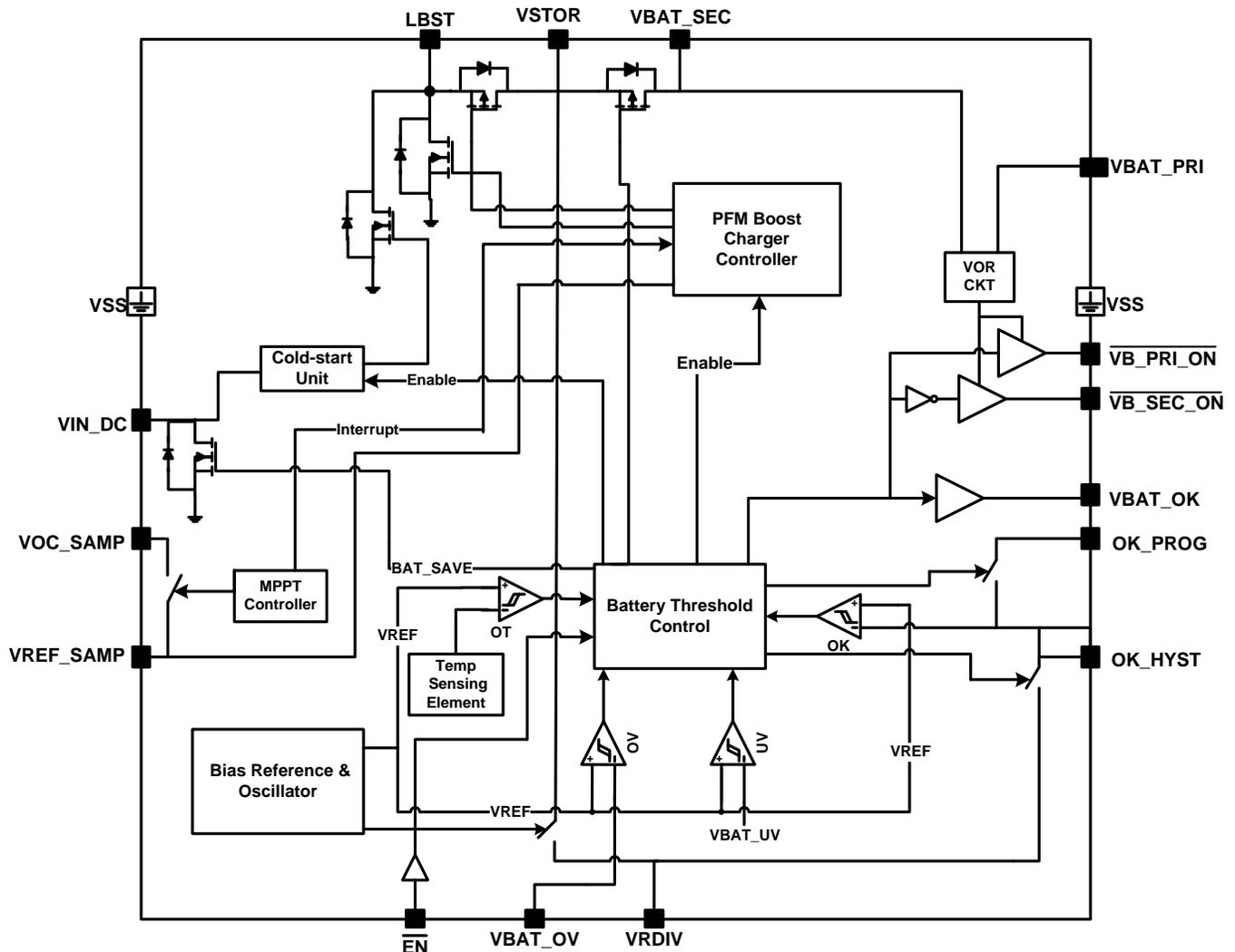
图 3. bq25505 Functional Block Diagram
