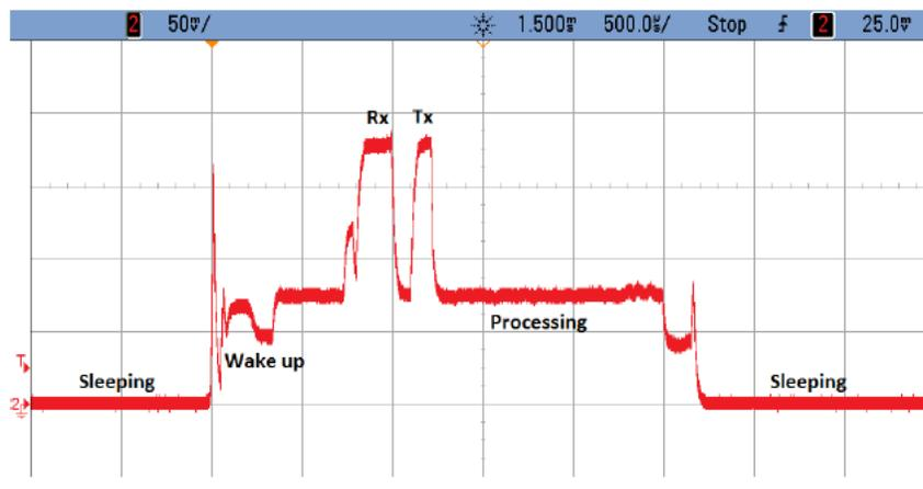
图 7. Current Consumption versus Time During a Single Connection Event
