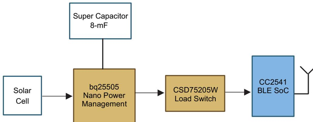
图 2. Bluetooth Low Energy Beacon Subsystem Block Diagram
