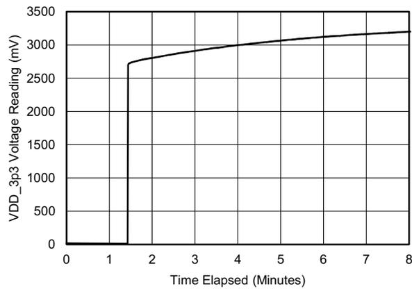
图 24. VDD\_3p3 After Load Switch as Controlled by bq25505
