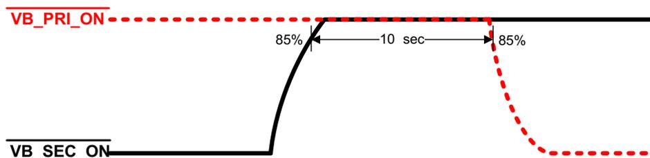
图 6. Break-Before-Make Operation of VB\_PRI\_ON and VB\_SEC\_ON
