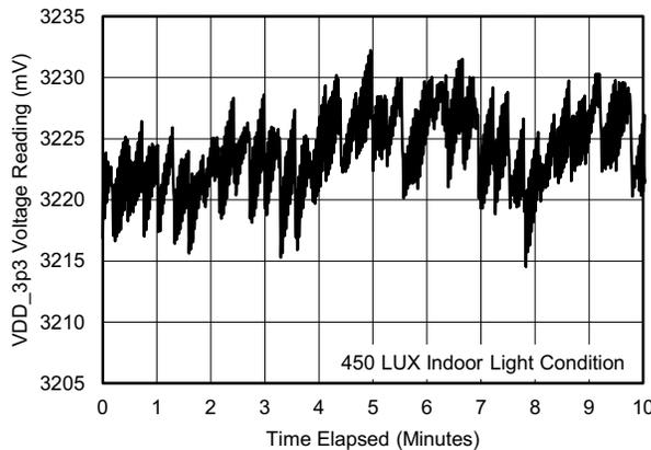
图 19. Voltage VDD\_3p3 Measured During BLE Beacon Transmissions (Functional Mode)
