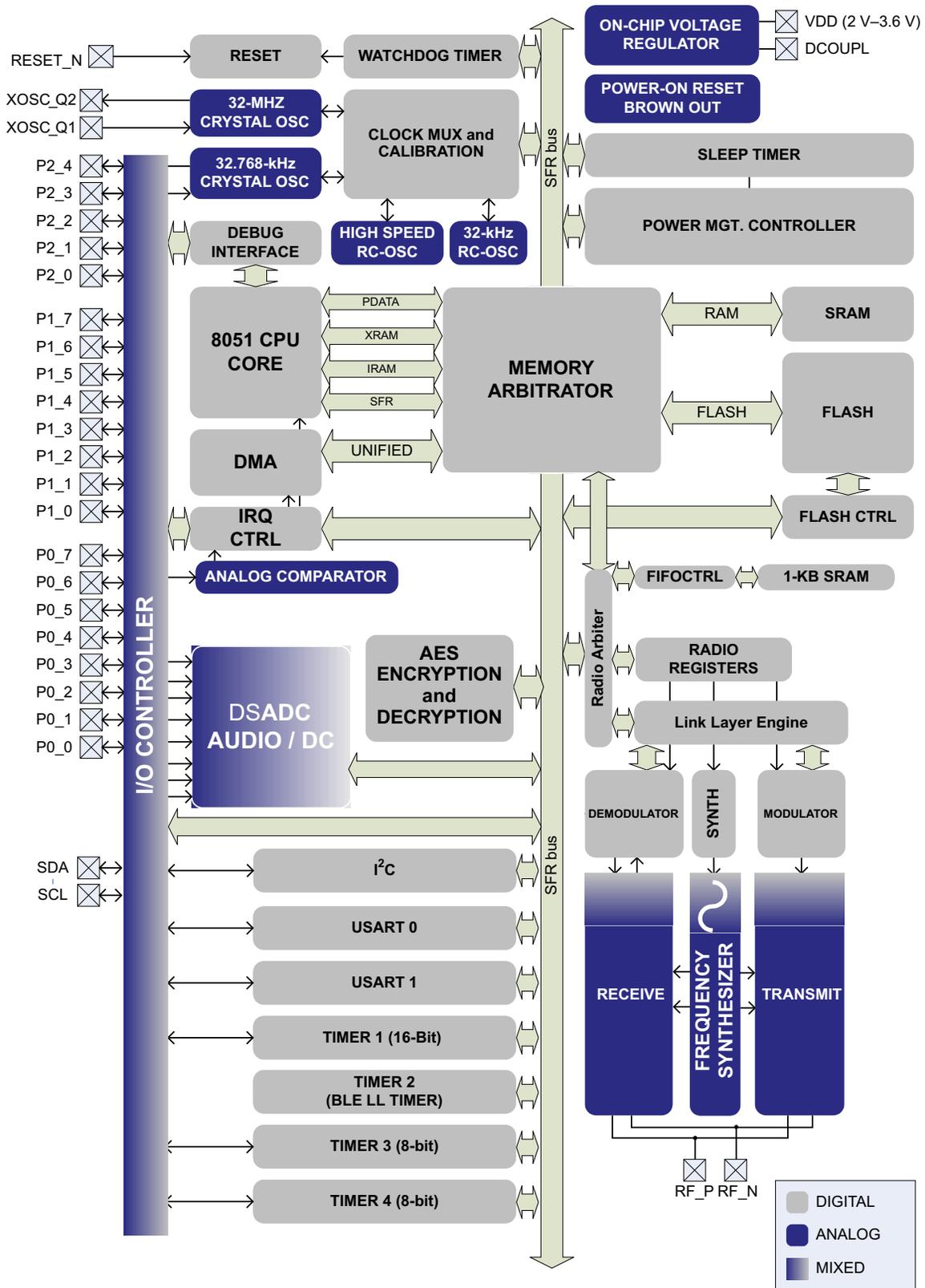
图 4. CC2541 Functional Block Diagram
