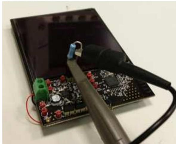
图 13. Current Probe Measurement for Dynamic Power Measurement
