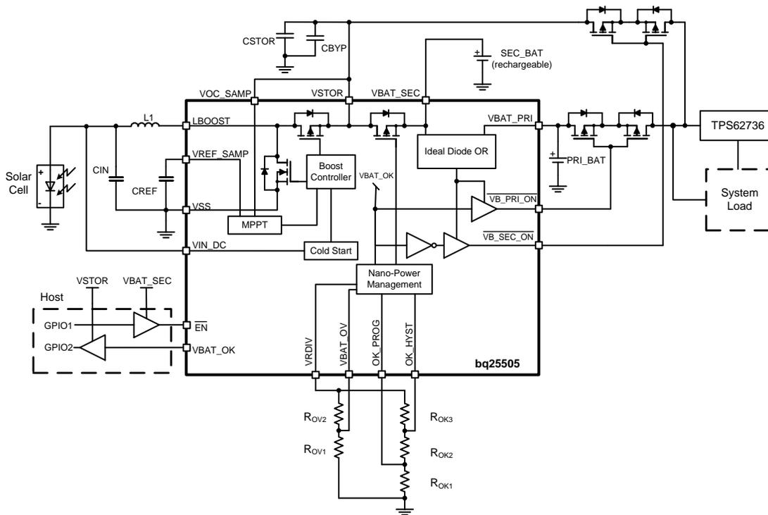
图 3. bq25505 Functional Block Diagram
