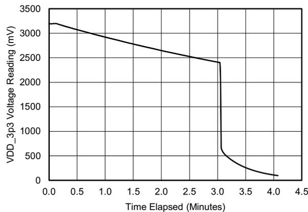
图 26. VDD\_3p3 After Load Switch as Controlled by bq25505
