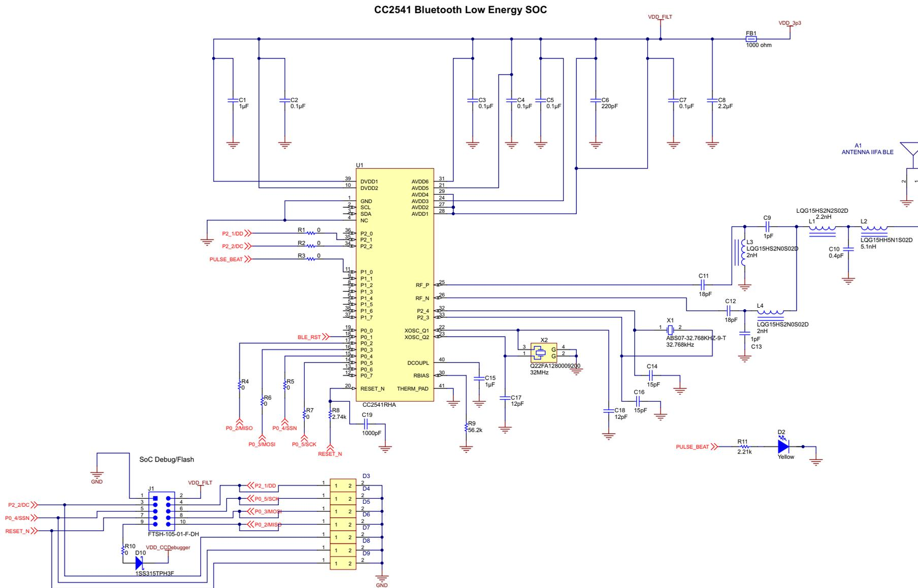
图 28. CC2541 Bluetooth Low Energy SOC Schematic
