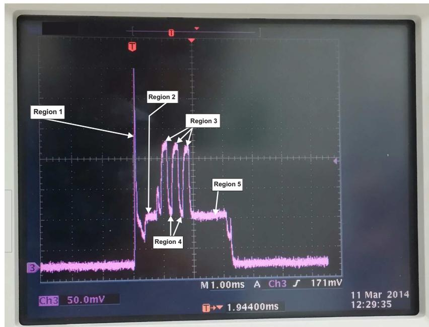
图 14. Power Drawn During Beacon Transmission
