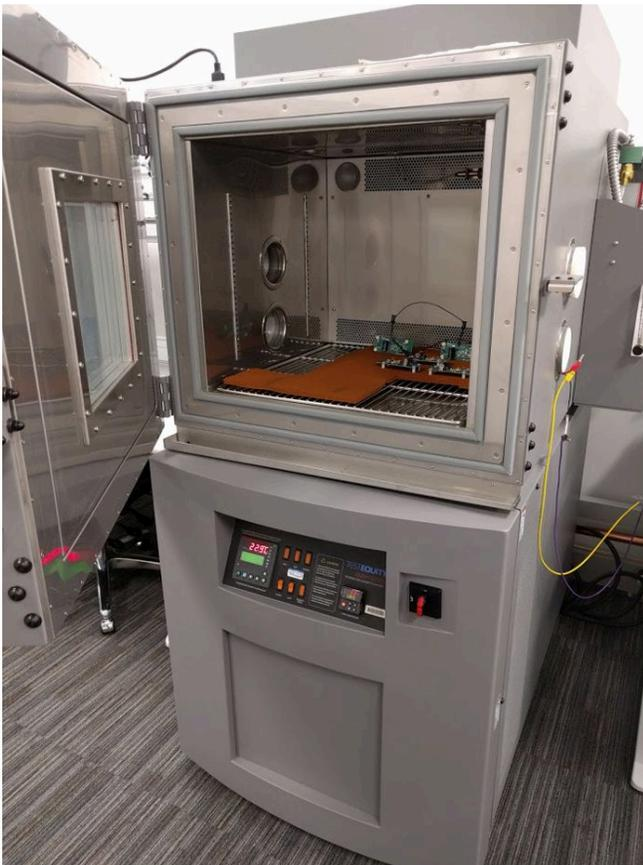
图 26. Temperature and Humidity Test Setup
