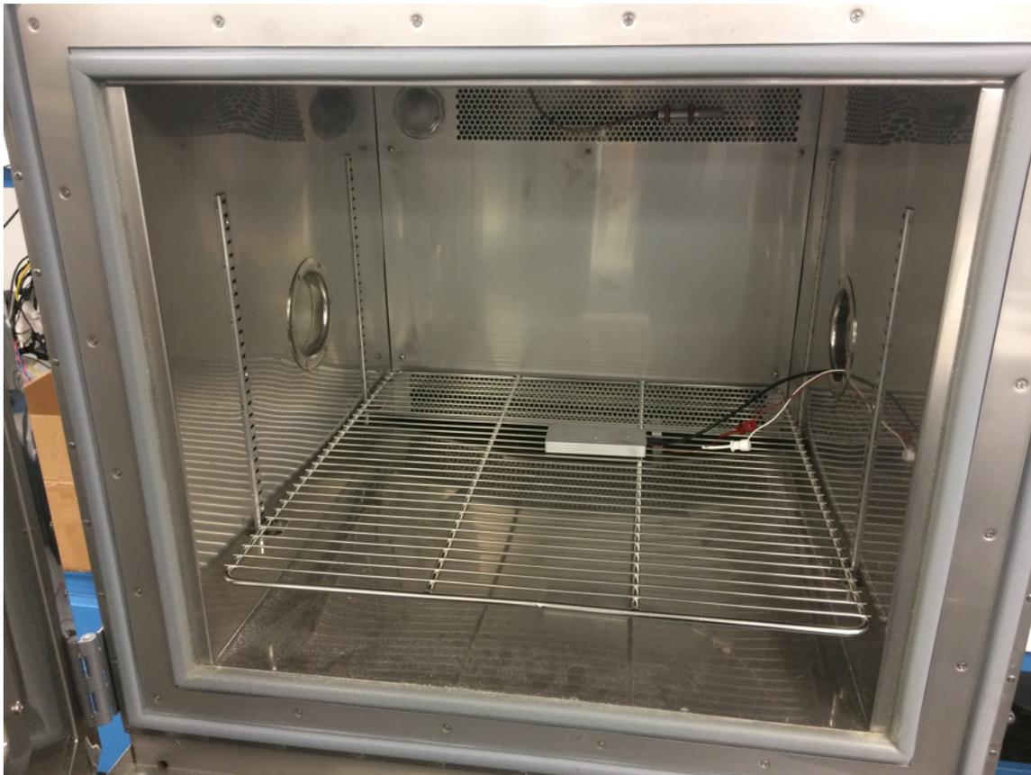
**图 43. Temperature and Relative Humidity Test Setup**
