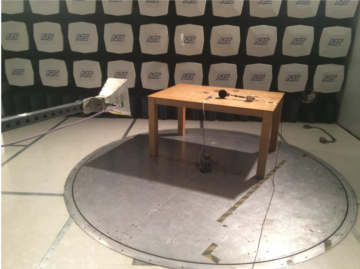
图 55. IEC 61000-4-3 Radiated Immunity Test Setup
