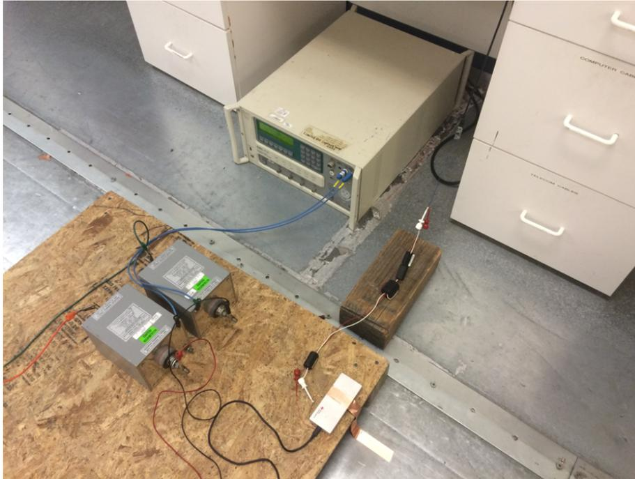
图 74. IEC 61000-4-5 Surge Test Setup
