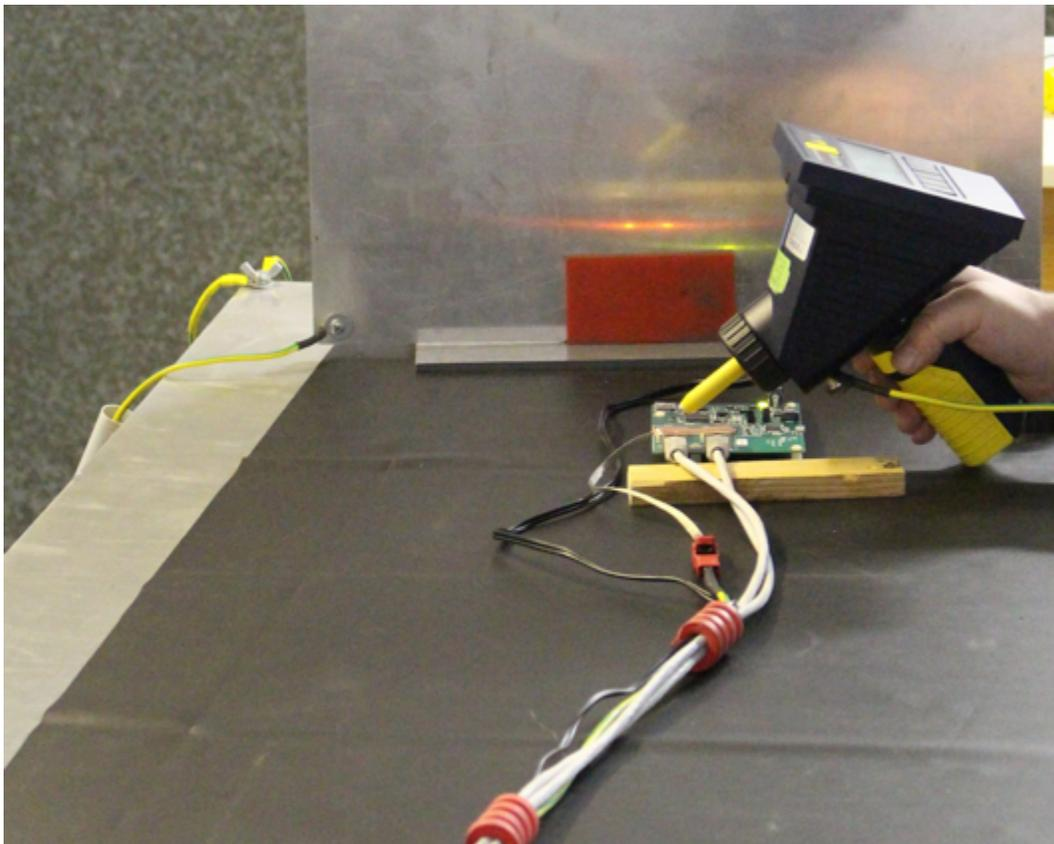
图 62. IEC61000-4-2 Test Setup for TIDA-00204 (Picture of 6-kV CD)
