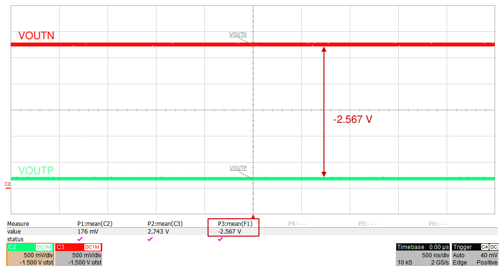
图 6-5. Typical Fail-Safe Output of the AMC3330
