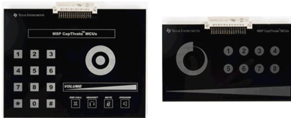
Figure 7-6. CAPTIVATE-PHONE and CAPTIVATE-BSWP Panels
