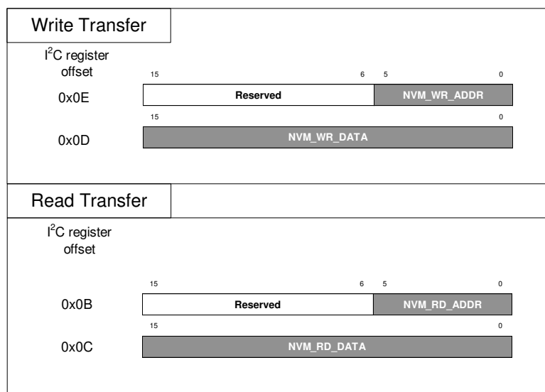
图 8-12. EEPROM Direct Access Using I 2 C
