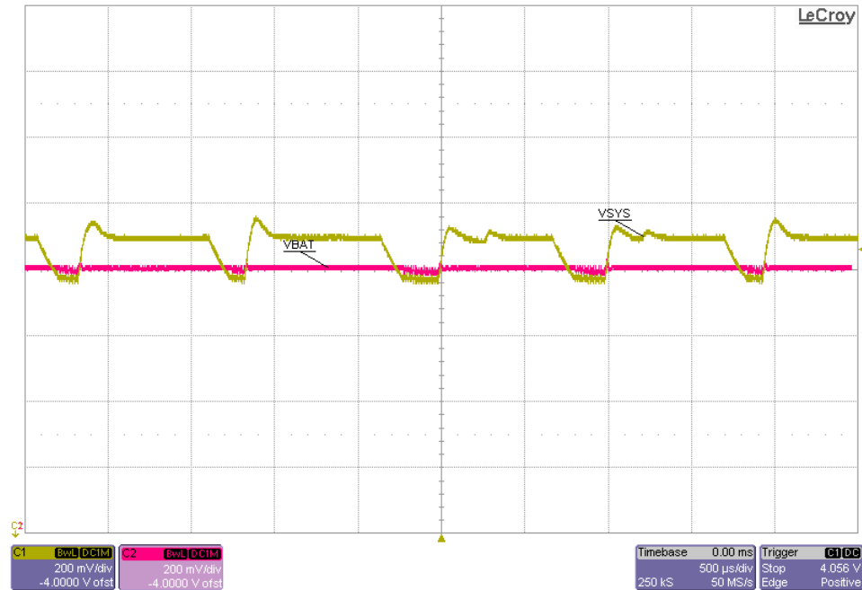
图 8-7. V(SYS) When Reverse Boost Prevention Circuit is Active
