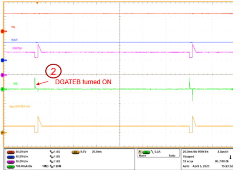
Figure 16. DGATE 交错开通放大图 1
