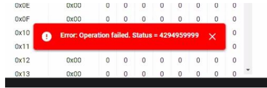
Figure 6. I2C2 未连接时软件报错信息
