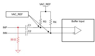
If the input amplitude or Vpp is greater than datasheet specification a  $50\Omega$  resistor to ground is used to meet the input requirements. This re-biasing is true for both differential (using INP and INN) and single ended input waveforms(using just INP).R3 and R4 are usually  $50\Omega$ .
