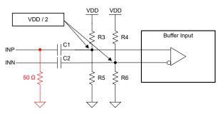
If the input amplitude or Vpp is greater than datasheet specification a  $50\Omega$  resistor to ground is used to meet the input requirements. This is usually not required in this case because bias point is set around VDD/2 and there is usually enough room for the input swing between GND and VDD for absolute maximum specification. This re-biasing is true for both differential (using INP and INN) and single ended input waveforms(using just INP).
