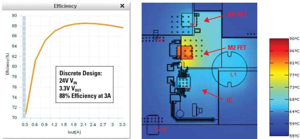
**Figure 6. WEBENCH Simulation Output for a Discrete Design**
