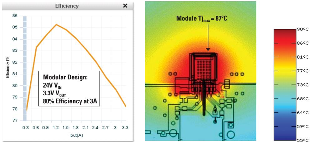
Figure 7. WEBENCH Simulation Output for a Modular Design
