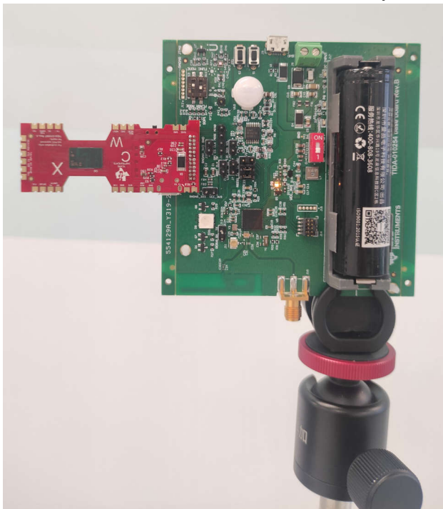
Figure 3-12. Design Module With TIDA-010254 Base Board on a Tripod
