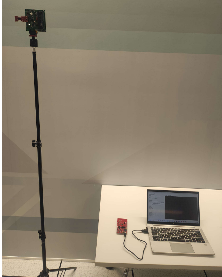
Figure 3-14. Bluetooth® LE Demonstration Position Setup
