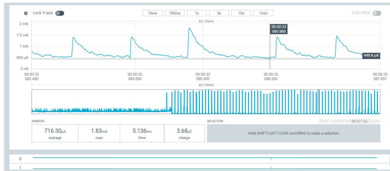
Figure 3-20. Module Minimum Current Waveframe
