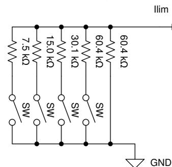
With this methodology, four switches can select 16 current levels. Both eFuses support different levels. The eFuse for the next node has steps of 300 mA and a maximum current of 4.8 A. The eFuse for the load connected to the node has steps of 200 mA and a maximum current of 3.2 A. Table 2 shows the relationship between the current levels and the switch settings for the application power eFuse. Table 3 shows the same information for the next node eFuse.
