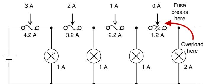
Electronic fuses (eFuses) are the ideal devices to fulfill this requirement so that all nodes can be built identical and configured ad hoc. Figure 8 shows such a configuration as it is implemented in this design. Each node can then be protected with a current level according to the sum of its own maximum current and all currents of the next nodes.
