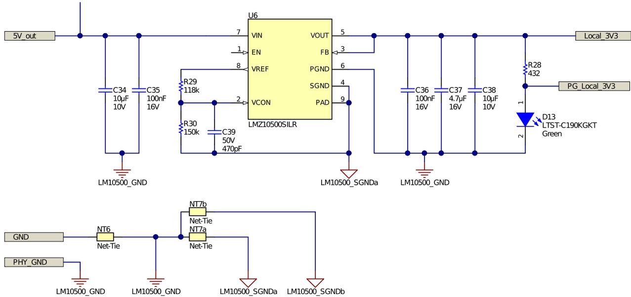
Net-tie NT6 connects the PHY analog ground AGND with the digital ground GND and the local LMZ10500 PHY power supply ground. This eases layout design because the position of the net-tie, and therefore the connection between AGND and GND, can be determined exactly. There is no need to cut the ground polygon to create the analog ground island.
