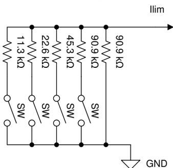
Figure 10. Resistor Setting for 4.8 A (Maximum)
