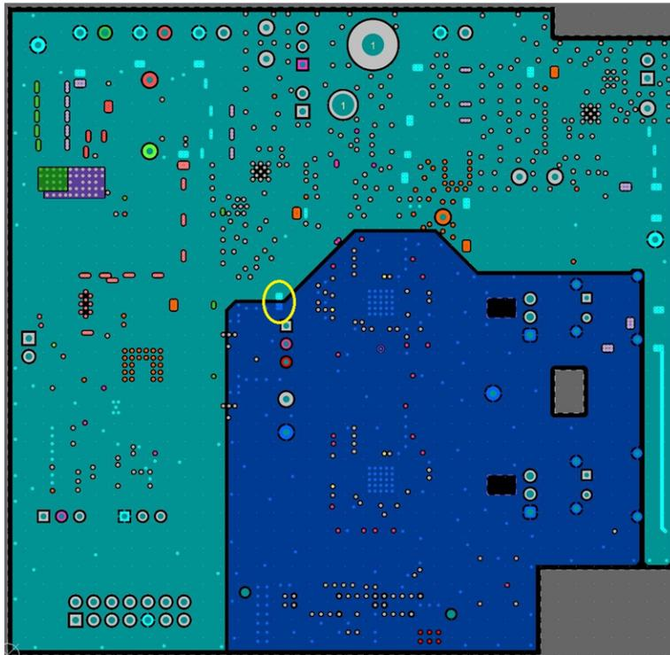
These ties are used on every building block so that the local components have their own ground which is then connected to the global ground where applicable. Noise from current loops in the switch mode power supplies is then kept local and doesn't travel across the board. [Figure 24](#) shows how this is handled in the schematics.
