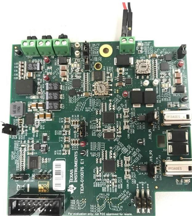
Figure 19. Jumpers, Connectors, and Test Points
