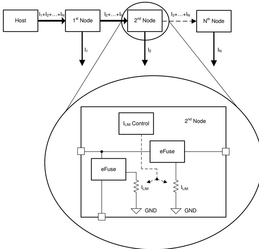
By adding an additional programmable eFuse for each node's power extraction port, it is possible to isolate a fault to a single location. This keeps the system up and running also in case of an overload condition at any place.
