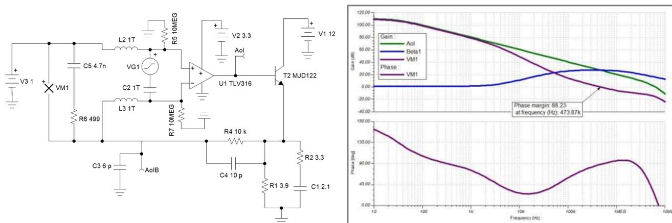
Figure 2-12. TINA-TI™ Stability Analysis of EC Mirror Driver With Compensation
