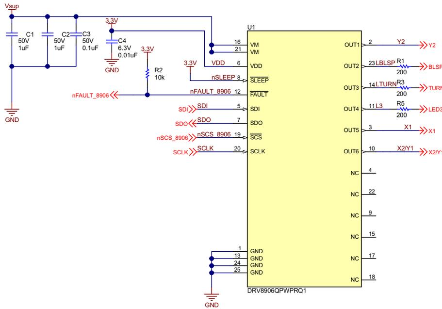
Figure 2-7. DRV8906-Q1 Configuration Schematic
