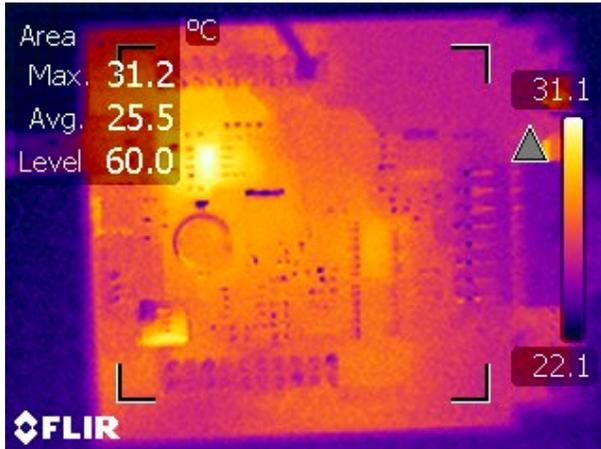
Figure 3-8. Reference Thermal Image of PCB
