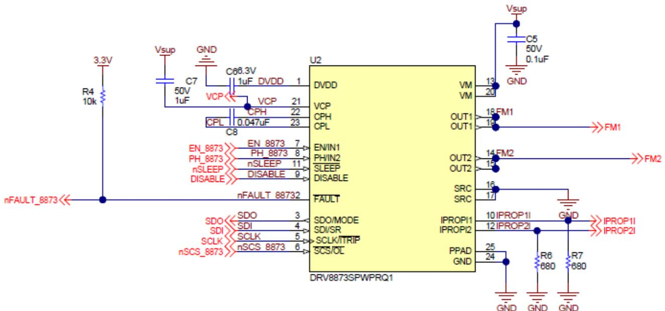
Figure 2-8. DRV8873-Q1 Configuration Schematic
