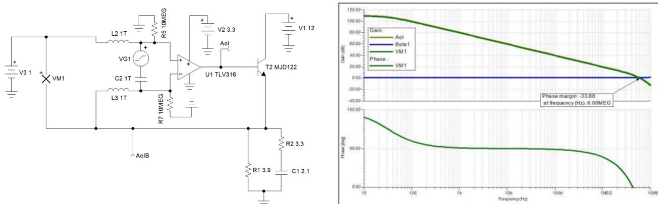
Figure 2-11. TINA-TI™ Stability Analysis of EC Mirror Driver Without Compensation
