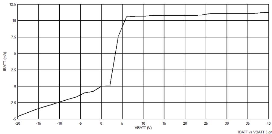
Figure 3-7. Input Voltage vs Input Current Graph
