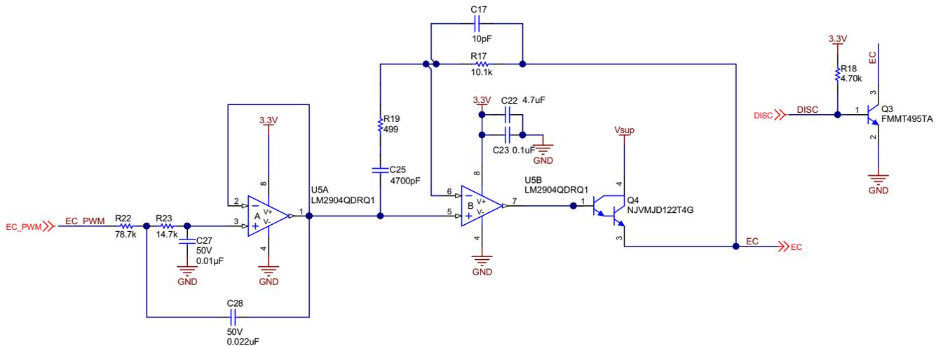
**Figure 2-10. Electrochromic Mirror Driver Circuit**
