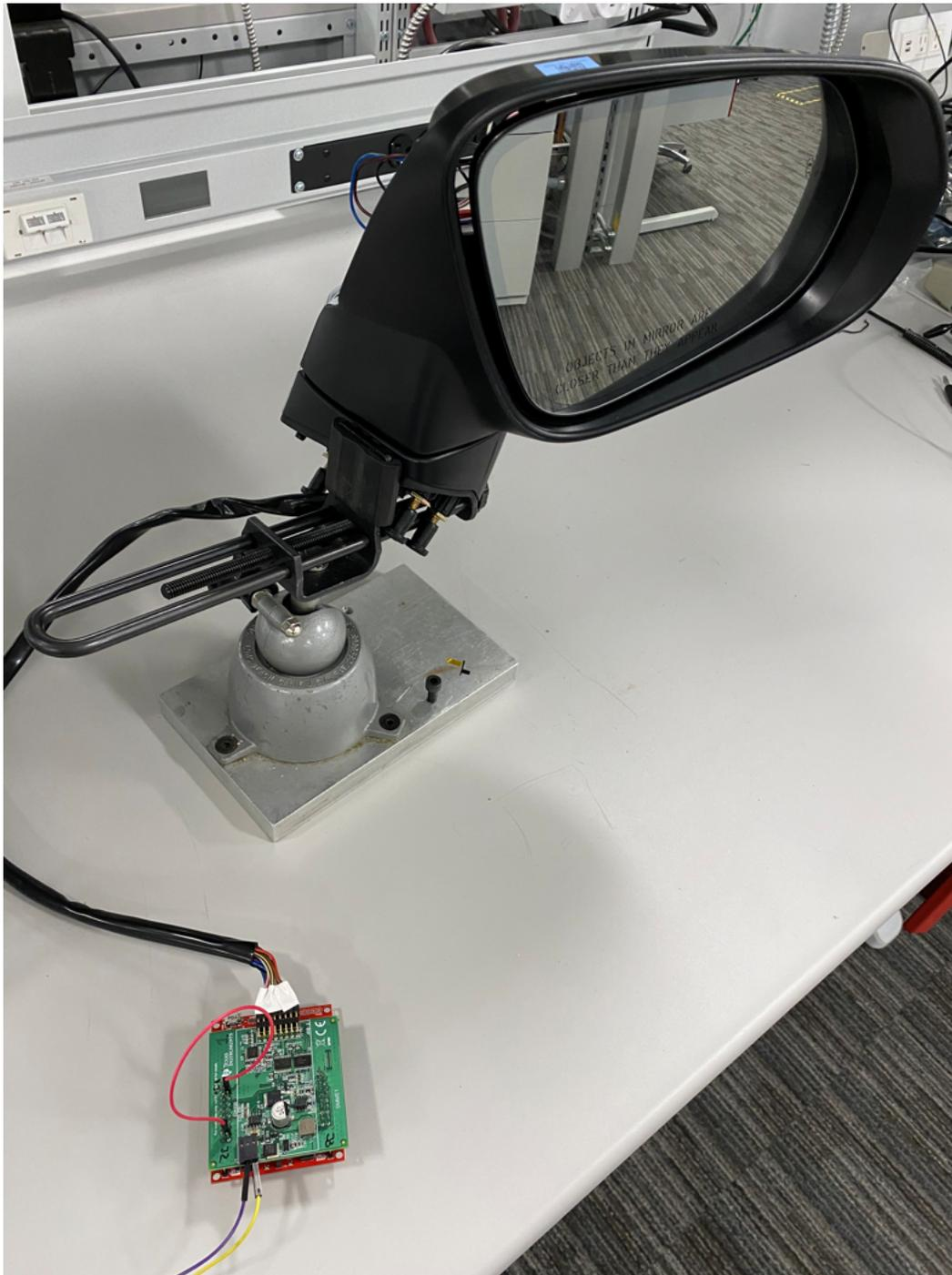
**Figure 3-5. TIDA-020027 Test Set-up**
