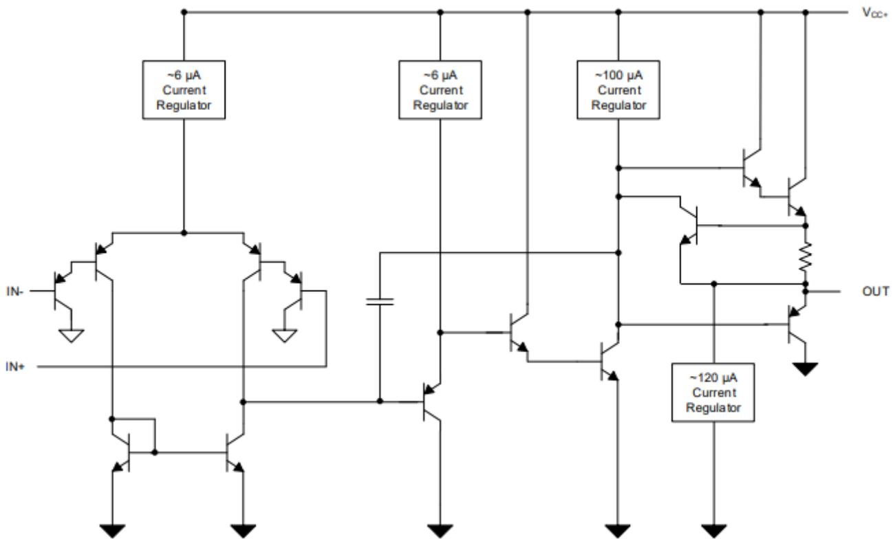
Figure 2-5. LM2904B-Q1 Block Diagram
