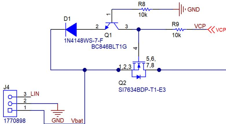
Figure 3-6. Reverse Battery Protection Circuit
