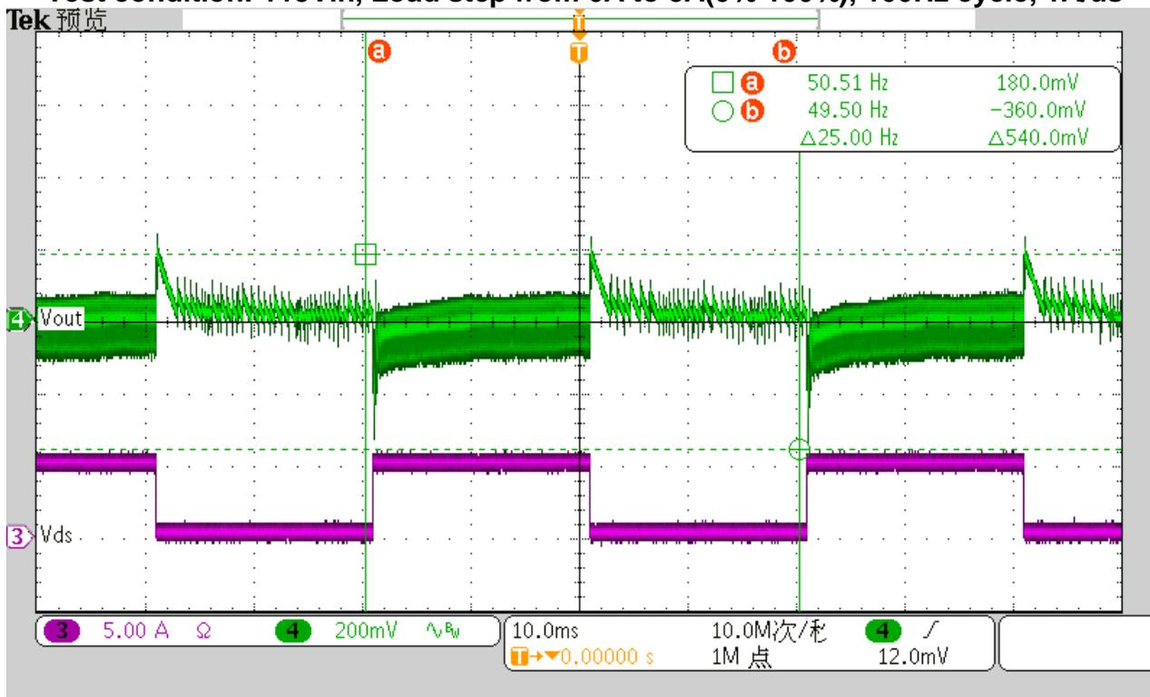
Test condition: 230Vin, Load step from 0A to 5A(0%-100%), 100Hz cycle, 1A/us
