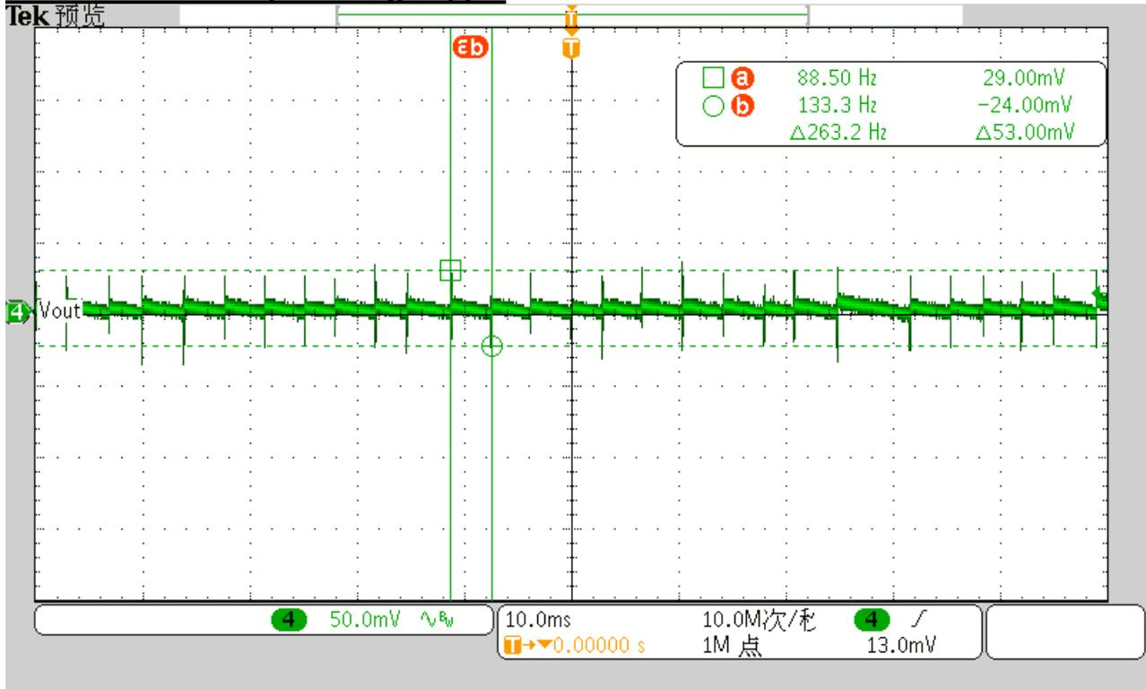
**230Vin no load output voltage ripple**
