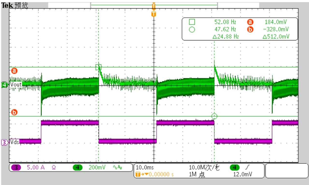
Test condition: 115Vin, Load step from 0A to 5A(0%-100%), 100Hz cycle, 1A/us
