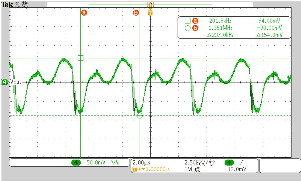
**115Vin full load output voltage ripple**
