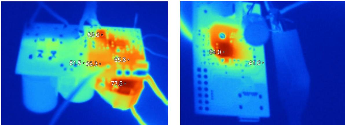
115Vac Input, output is 9V/5A load (30 minutes) without fan cooling
