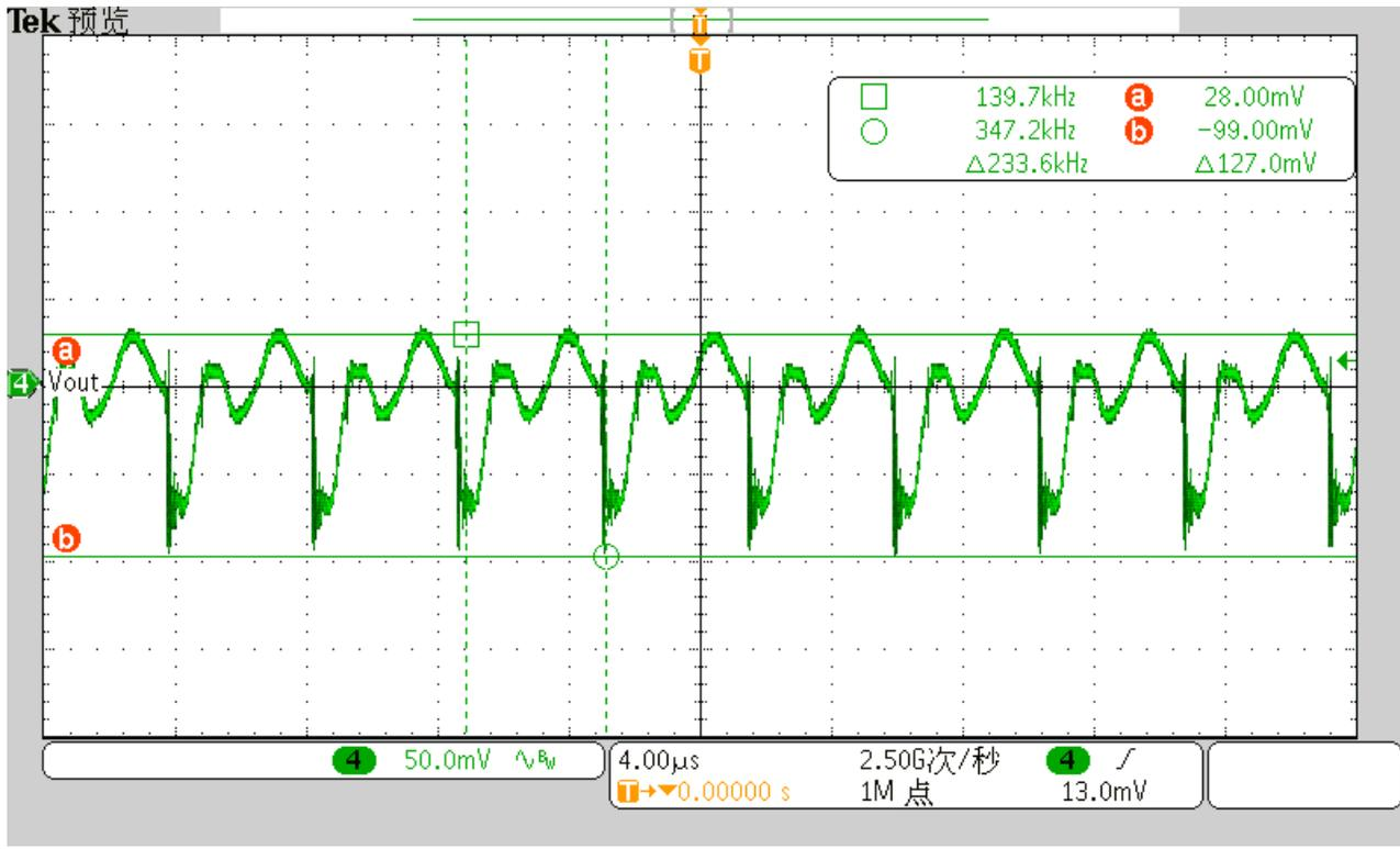
**230Vin full load output voltage ripple**
