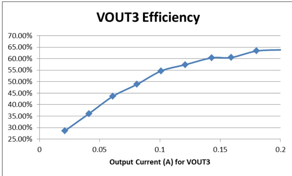
The below plot is an efficiency plot showing the efficiency of the entire system. The three outputs are all loaded simultaneous. The currents are at 20%, 40%, 60%, 80%, and 100% of their full loads.
