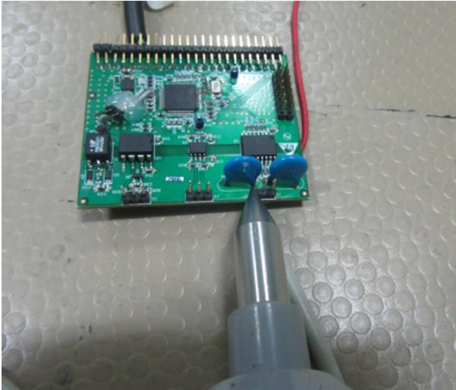
Figure 45. ESD Test Setup for Contact Discharge
