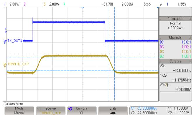
Figure 27. Fall Time of Terminated Output of ISO3082
