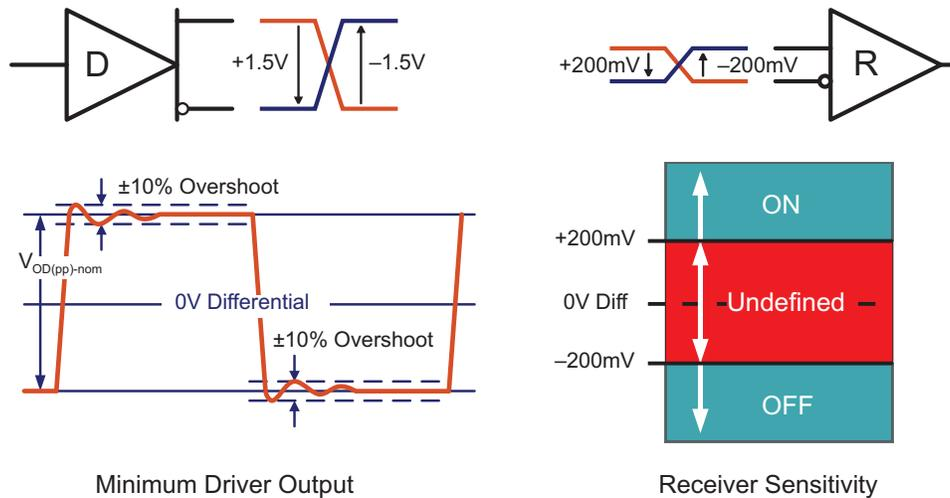
Figure 3. RS-485 Specified Bus Signal Levels
