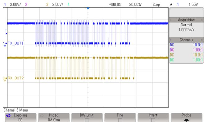
Figure 29. CAN Single Data Packet Communication
