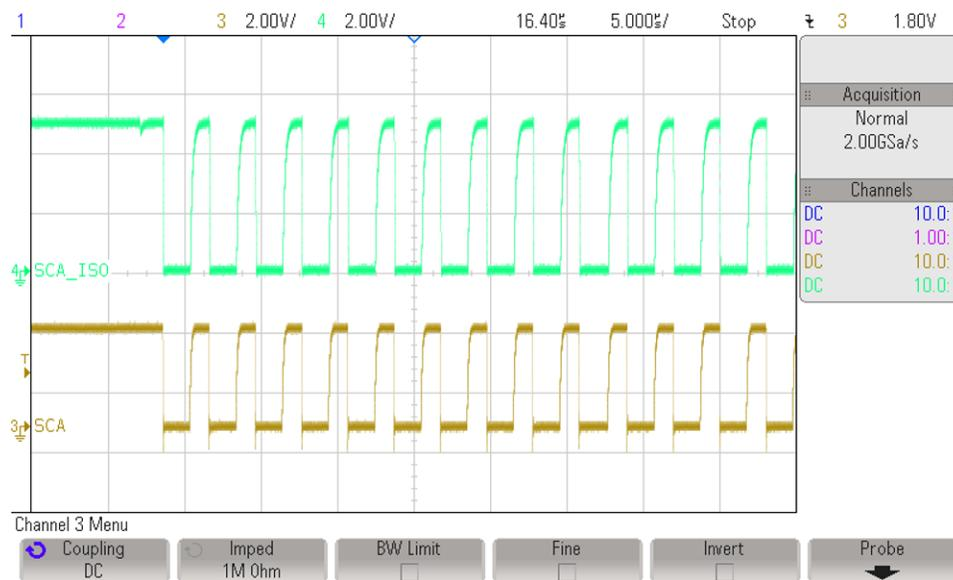
Figure 41. I2C Clock Waveform at the Input and Output of ISO1541
