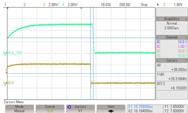
Figure 43. Falling Edge Propagation Delay of ISO1541
