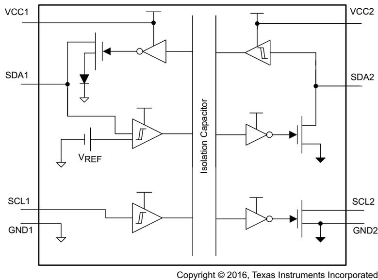
**Figure 7. ISO1541 Functional Block Diagram**
