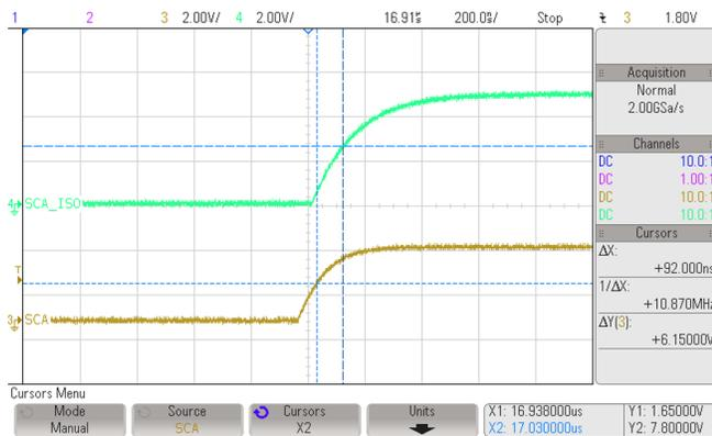
Figure 42. Rising Edge Propagation Delay of ISO1541
