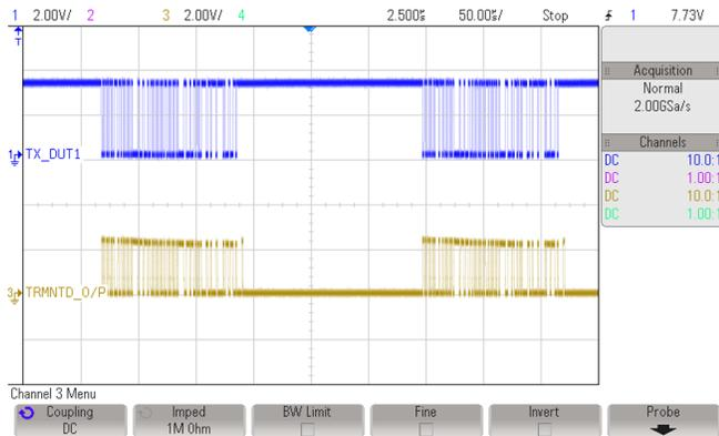
**Figure 32. ISO1050 Input and Terminated Output Waveform (Multiple Data Packets)**
