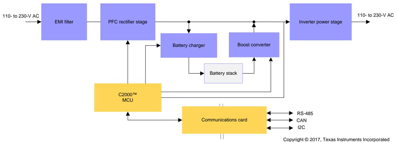
**Figure 1. System Block Diagram of Online UPS System**
