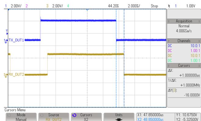
Figure 21. RS-485 Falling Edge Transmission Delay
