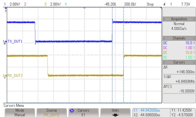
Figure 31. CAN Rising Edge Transmission Delay
