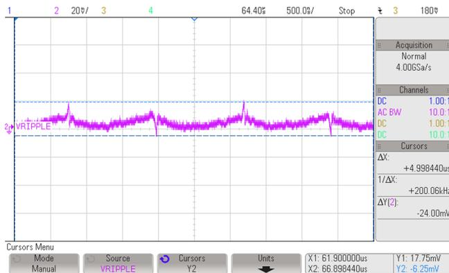
**Figure 48. Output Ripple at 1-W Load**
