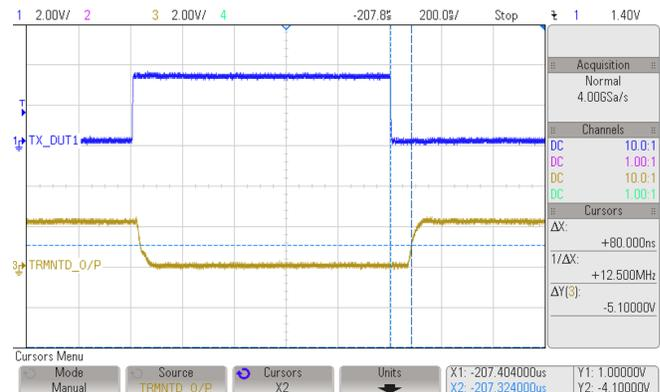
**Figure 35. Falling Edge Propagation Delay of ISO1050**
