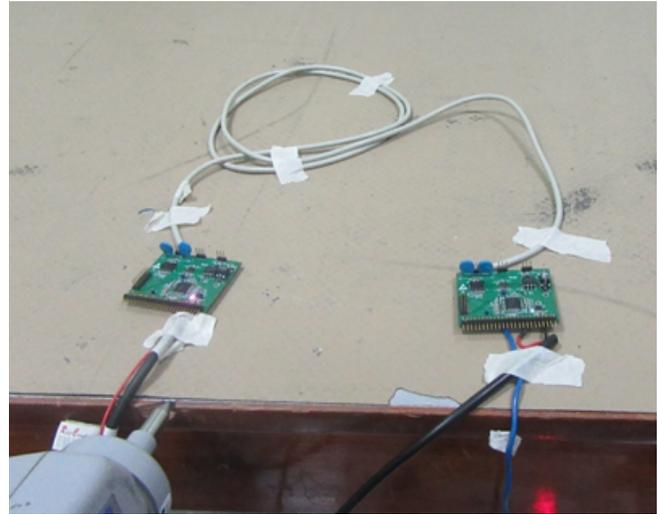
Figure 46. ESD Test Setup for Indirect Discharge by HCP
