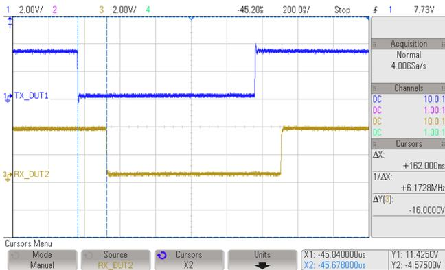
Figure 30. CAN Falling Edge Transmission Delay
