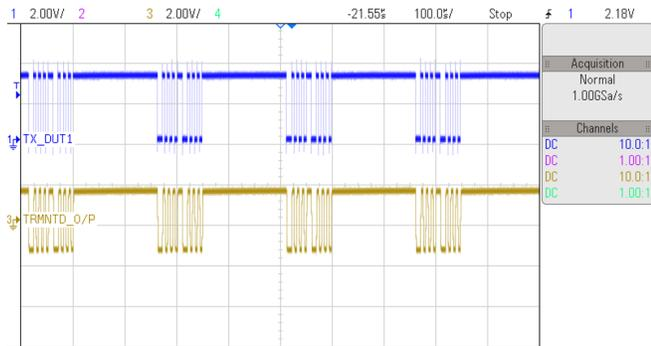
**Figure 22. ISO3082 Input and Terminated Output Waveform (Multiple Data Packets)**
