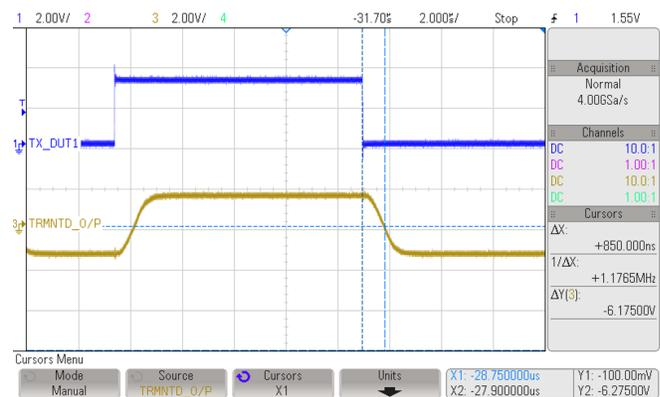
**Figure 25. Falling Edge Propagation Delay of ISO3082**
