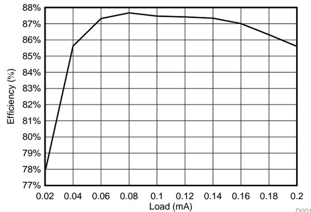
**Figure 49. Efficiency of Auxiliary Power Supply**
