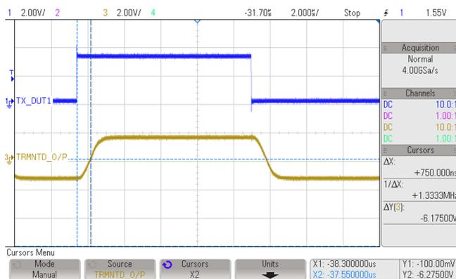
**Figure 24. Rising Edge Propagation Delay of ISO3082**
