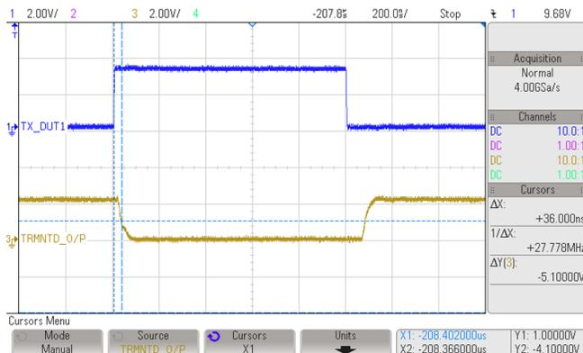
**Figure 34. Rising Edge Propagation Delay of ISO1050**
