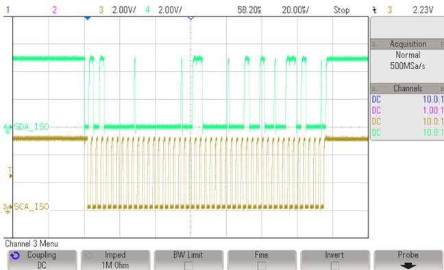
Figure 38. I2C Output Clock and Data
