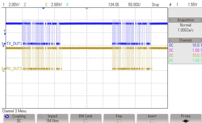
Figure 28. CAN Multiple Data Packet Communication
