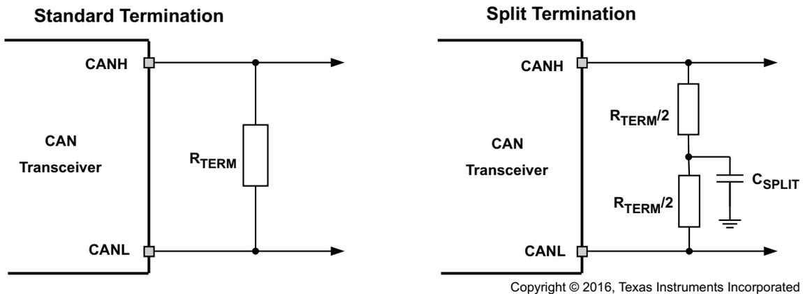
Figure 11. CAN Bus Termination Concepts
