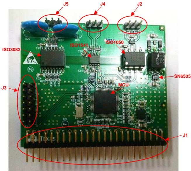
Figure 14. TIDA-01281 Front-Side Board Picture With Major Components
