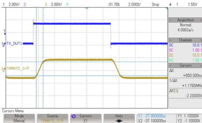
Figure 26. Rise Time of Terminated Output of ISO3082
