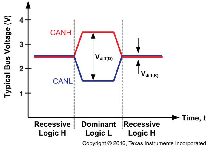
Figure 10. CAN Bus States (Physical Bit Representation)
