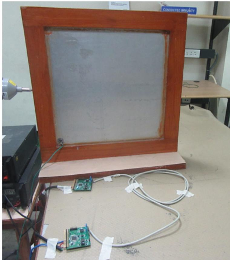
Figure 47. ESD Test Setup for Indirect Discharge by VCP
