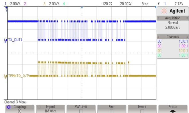
**Figure 33. ISO1050 Input and Terminated Output Waveform (Single Data Packet)**
