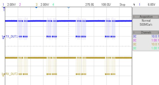
Figure 18. RS-485 Multiple Data Packet Communication
