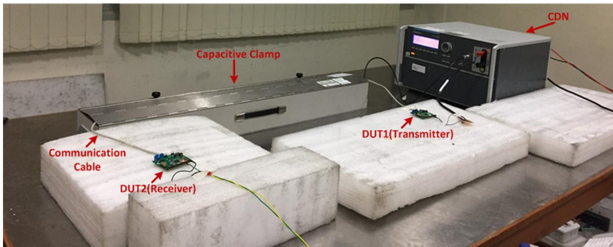
Figure 44. EFT Test Setup
