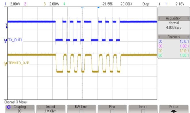
**Figure 23. ISO3082 Input and Terminated Output Waveform (Single Data Packet)**
