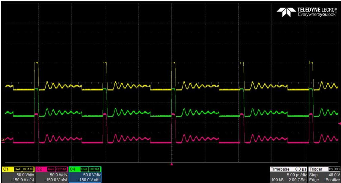
The photo below shows the FET switching voltage at TP4 (Red), the voltage at D2-cathode (Green) and D100-cathode (Yellow) for an input voltage of 15V and a 2mA load. (50V/DIV, 5uS/DIV)
