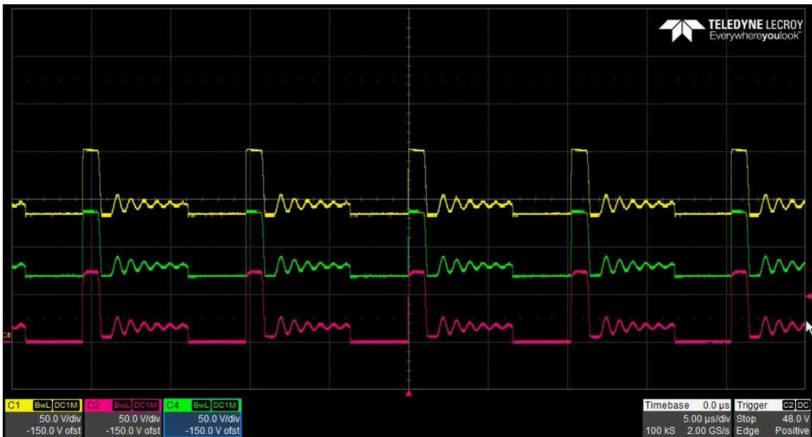
The photo below shows the FET switching voltage at TP4 (Red), the voltage at D2-cathode (Green) and D100-cathode (Yellow) for an input voltage of 9V and a 2mA load. (50V/DIV, 5uS/DIV)
