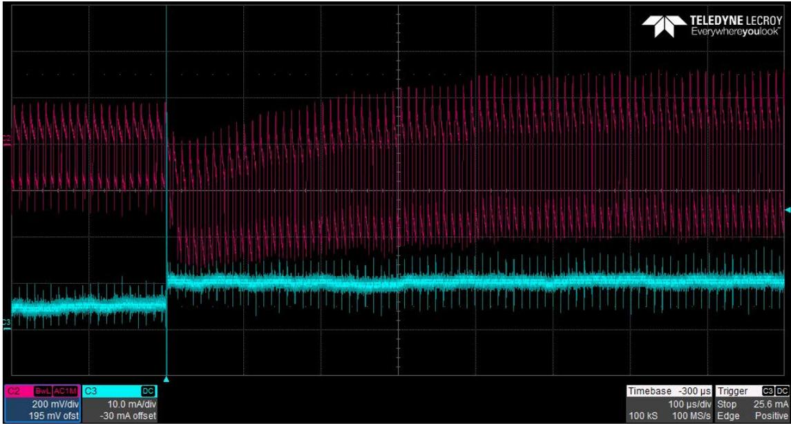
The photo below shows the 200V output voltage (ac coupled) when the load current is stepped between 10mA and 5mA.  $V_{in} = 12V$ .
