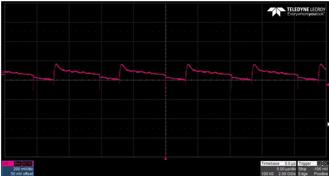
The 200V output ripple voltage (AC coupled) is shown in the figure below. The image was taken with the output loaded to 2mA. The input voltage is set to 15V. (200mV/DIV, 5uS/DIV)
