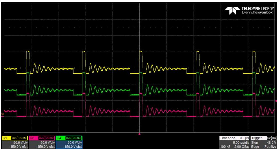
The photo below shows the FET switching voltage at TP4 (Red), the voltage at D2-cathode (Green) and D100-cathode (Yellow) for an input voltage of 15V and a 0mA load. (50V/DIV, 5uS/DIV)
