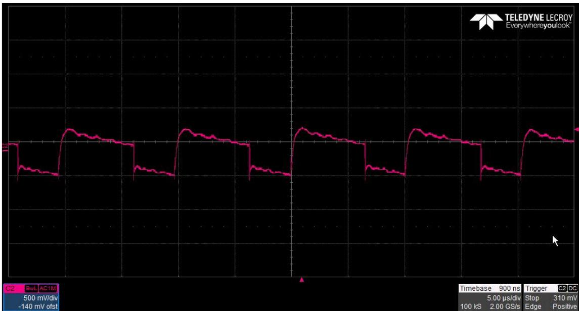
The 200V output ripple voltage (AC coupled) is shown in the figure below. The image was taken with the output loaded to 2mA. The input voltage is set to 9V. (200mV/DIV, 5uS/DIV)
