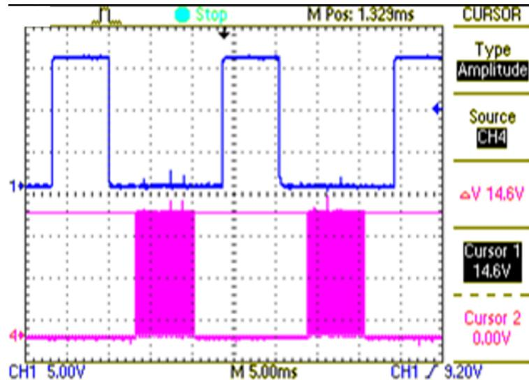
Figure 35. High-Side and Low-Side PWM Input to UCC27714
