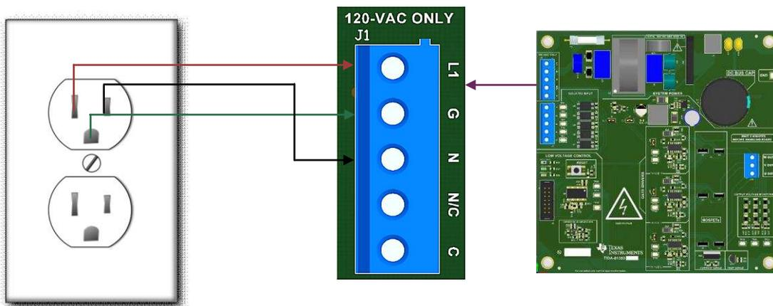
**Figure 24. 120-V AC Power Outlet Board Connection Example**
