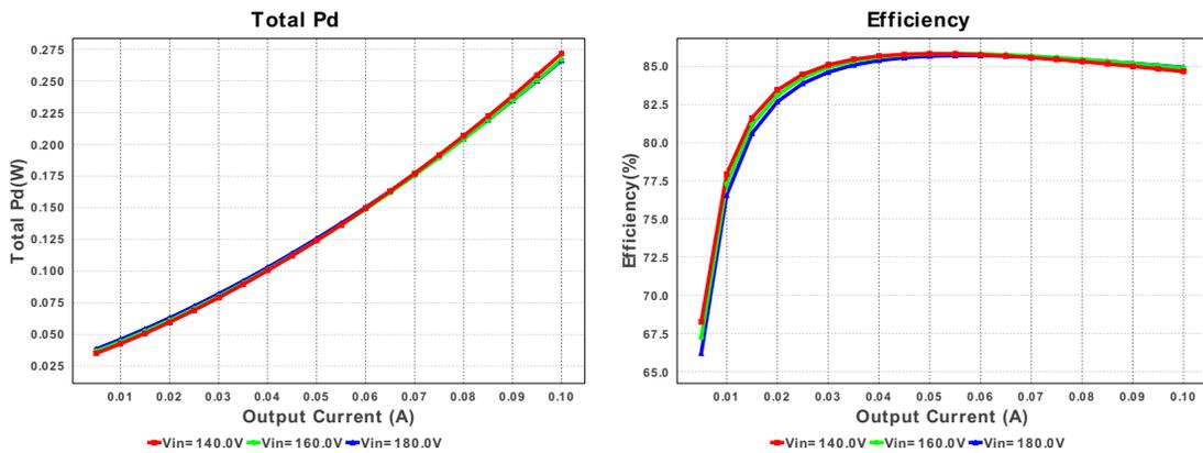
Figure 10. Buck Converter Simulation Output (Power Dissipation and Efficiency)
