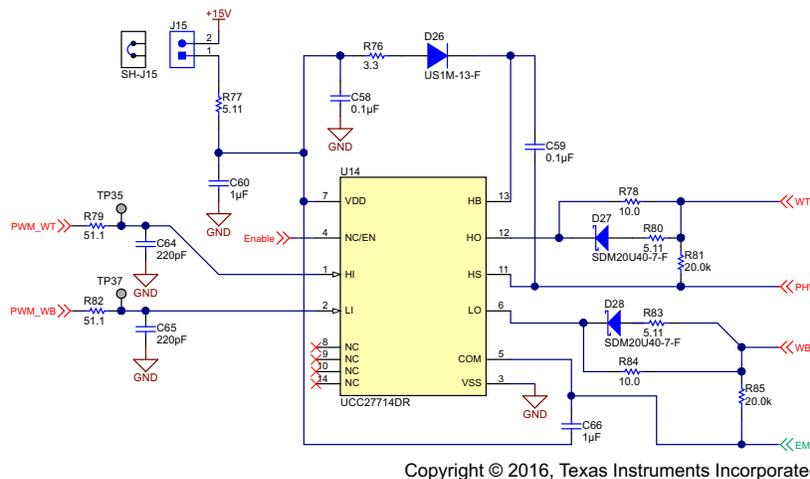
Figure 13. TIDA-01353 Application of UCC27714 Half-Bridge Gate Driver
