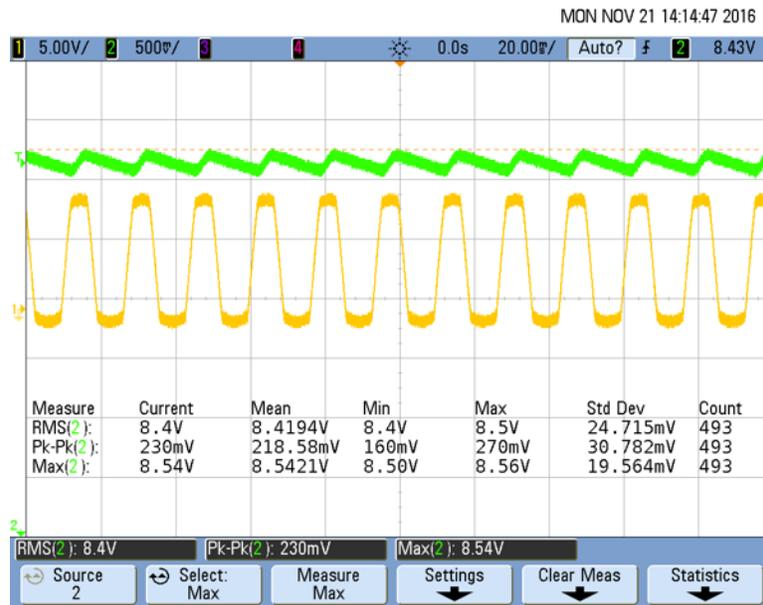
Figure 39. 10 Vp-p Input and DC\_Link Voltage Output
