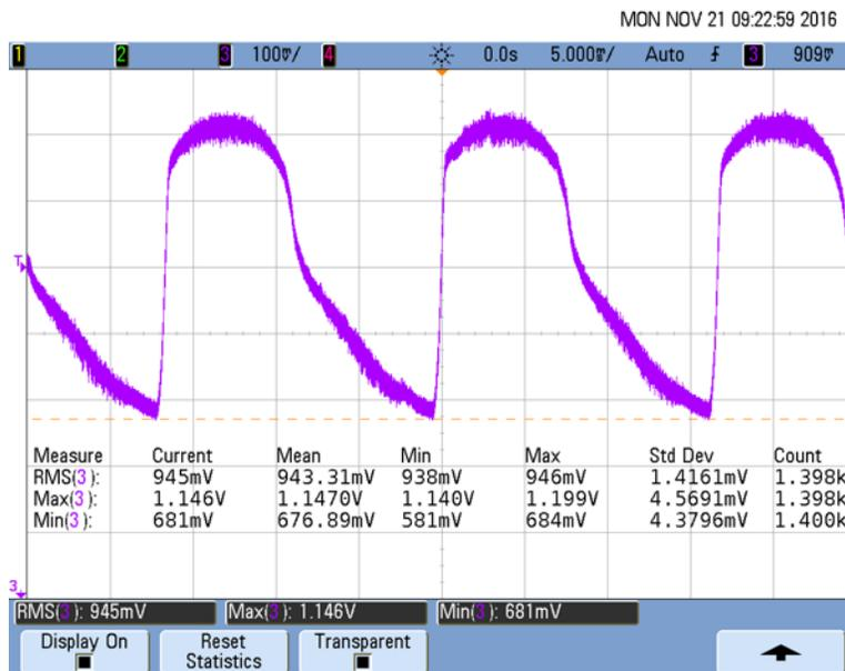
Figure 42. MCU Speed Setting Input From Optocoupler
