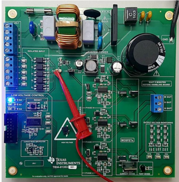
**Figure 27. 3.3-V Connection for MSP430F5132 JTAG Programming**
