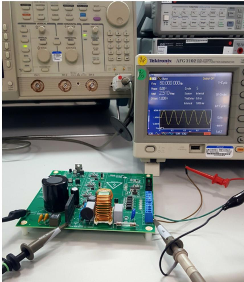
**Figure 38. Main Power Supply Testing Setup**
