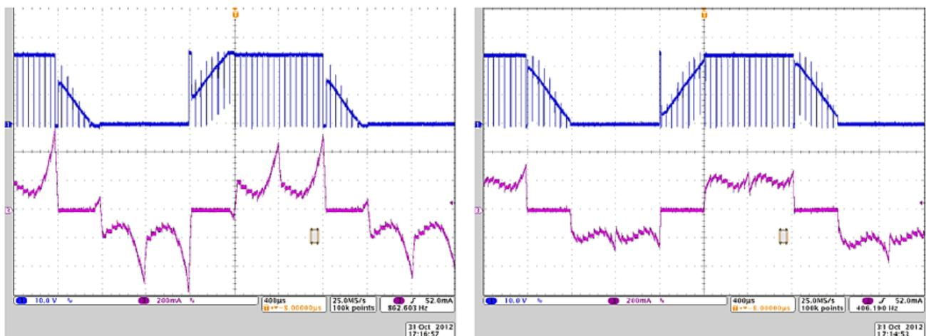
Figure 30. High versus Optimized Flux Threshold Waveforms
