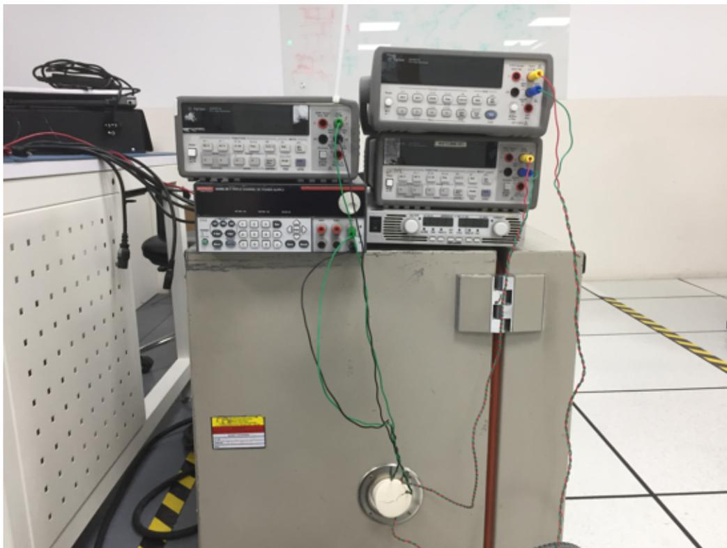
**Figure 9. Test Setup for Testing Across Temperature Range**
