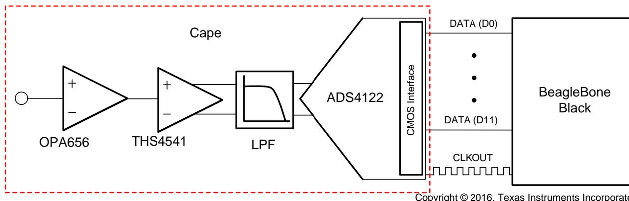
**Figure 1. TIDA-00942 Block Diagram**
