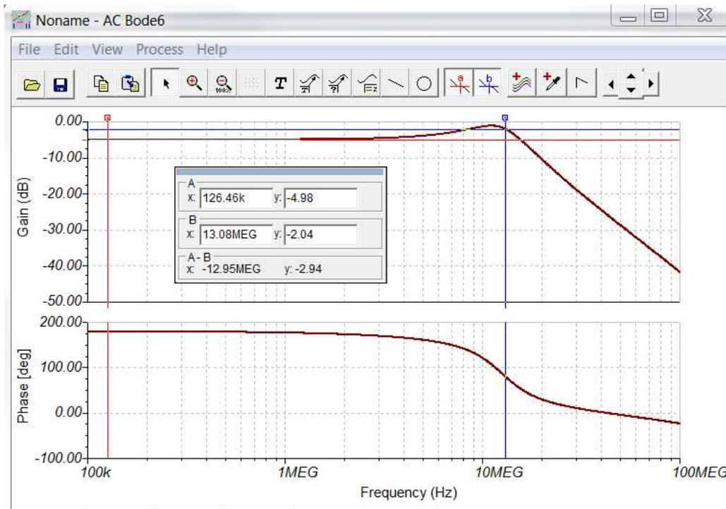
Figure 5. Frequency Response of FDA (THS4541) and MFB Low-pass Filter
