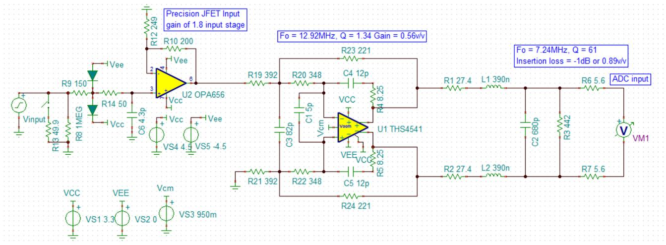
Figure 4. Input Circuit With OPA656, THS4541, and Low-pass Filter
