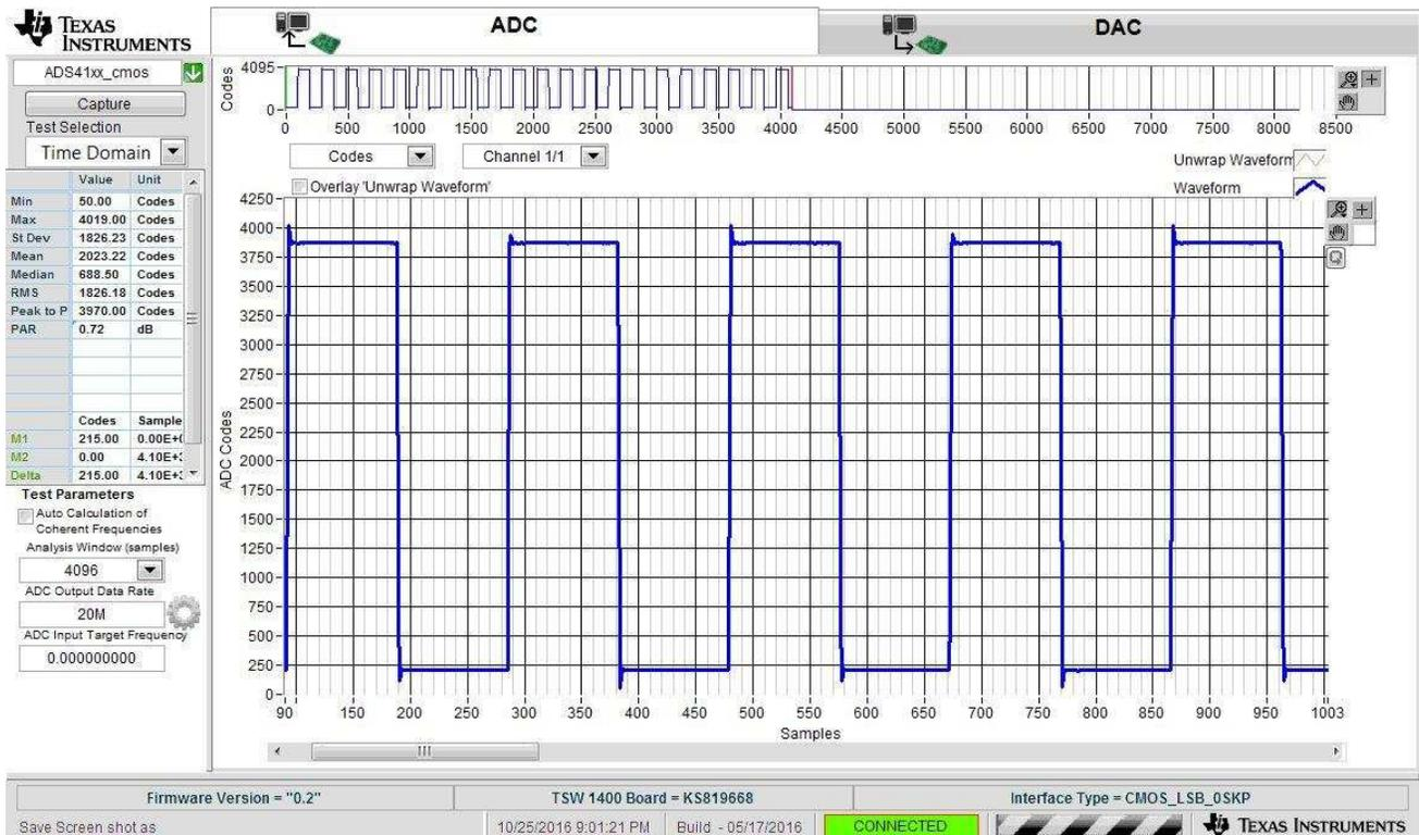
Figure 9. 100-KHz Square Wave Input
