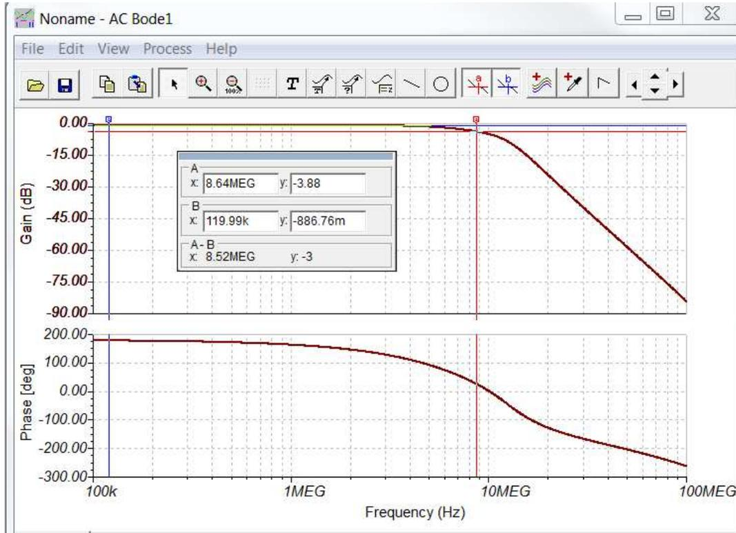
Figure 6. Frequency Response of Input Circuit
