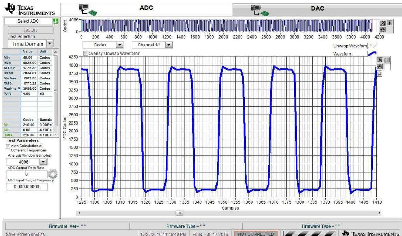
Figure 10. 1-MHz Square Wave Input
