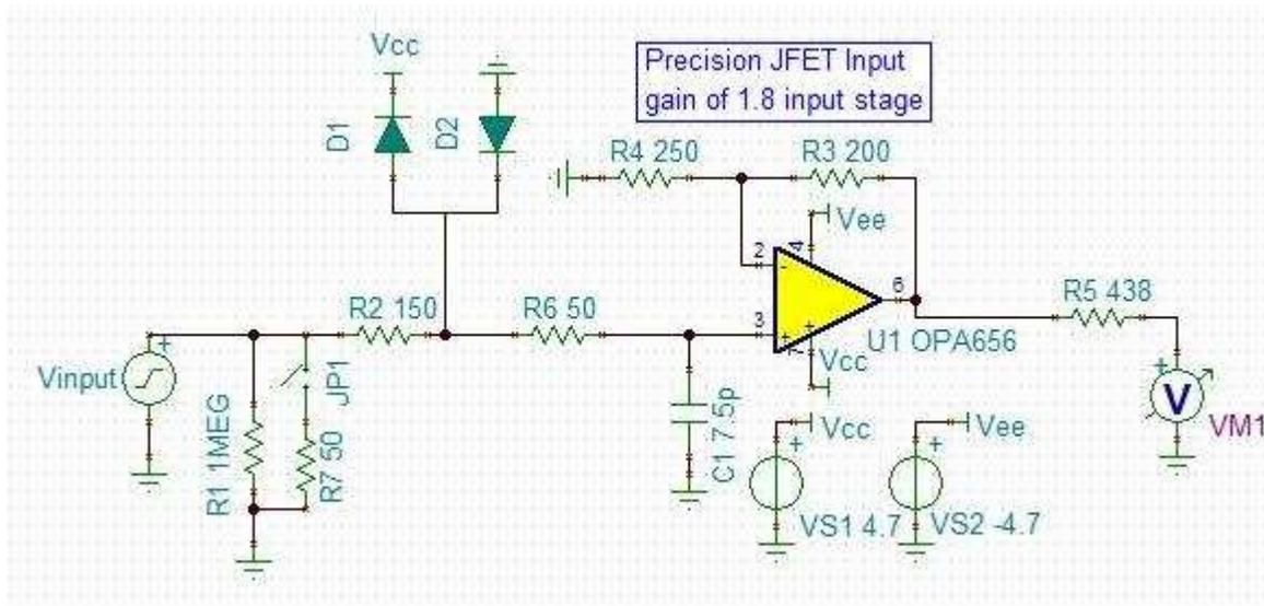
Figure 2. Circuit for Input Buffer Stage (OPA656)
