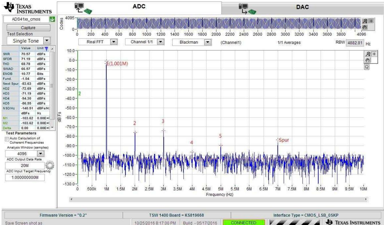
Figure 8. FFT 1-MHz -1-dBFS Input Signal
