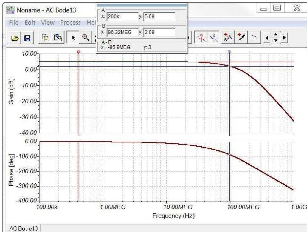
**Figure 3. Frequency Response of Input Buffer Stage (OPA656)**
