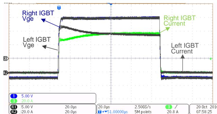
Figure 26. Current Sharing During One PWM Pulse
