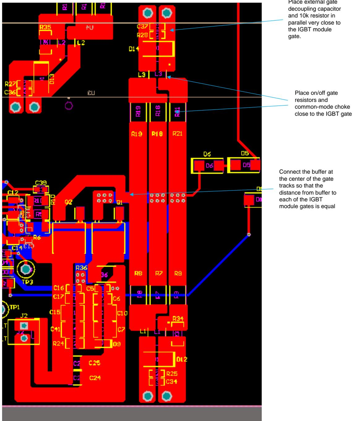
**Figure 31. Connection of Buffer to Gate Track**
