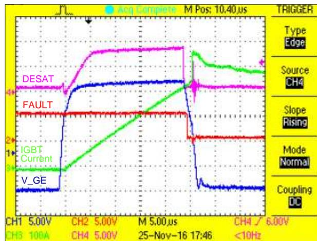
**Figure 29. IGBT DESAT Waveform Showing Fault Signal**
