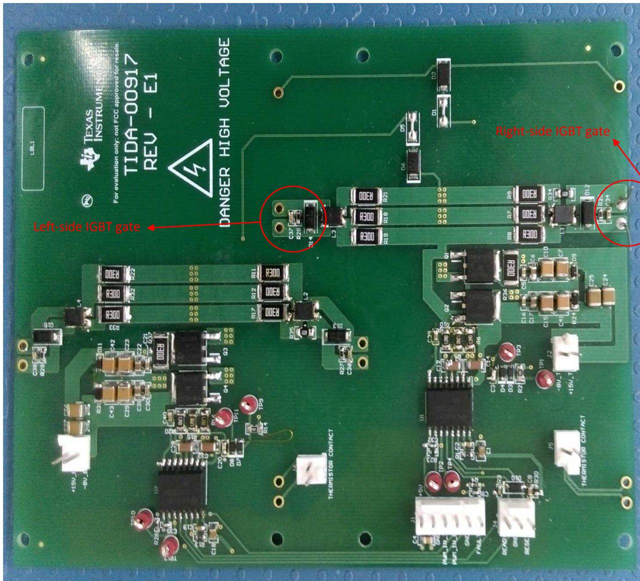
**Figure 18. Left and Right IGBT Modules**
