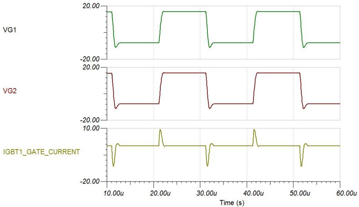
Figure 8. Simulation Results for Gate Current of IGBT
