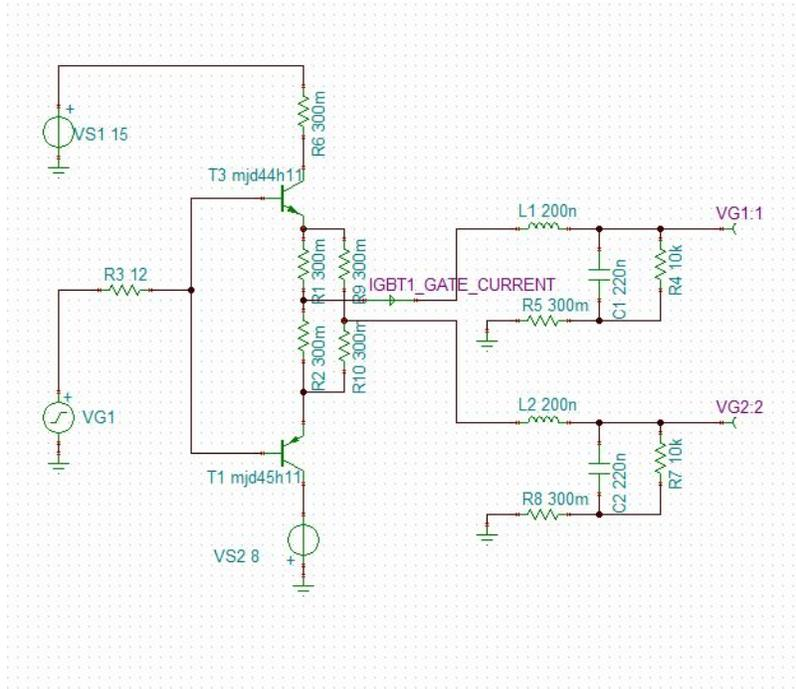
Figure 7. Schematic for Calculating Gate Current of IGBT
