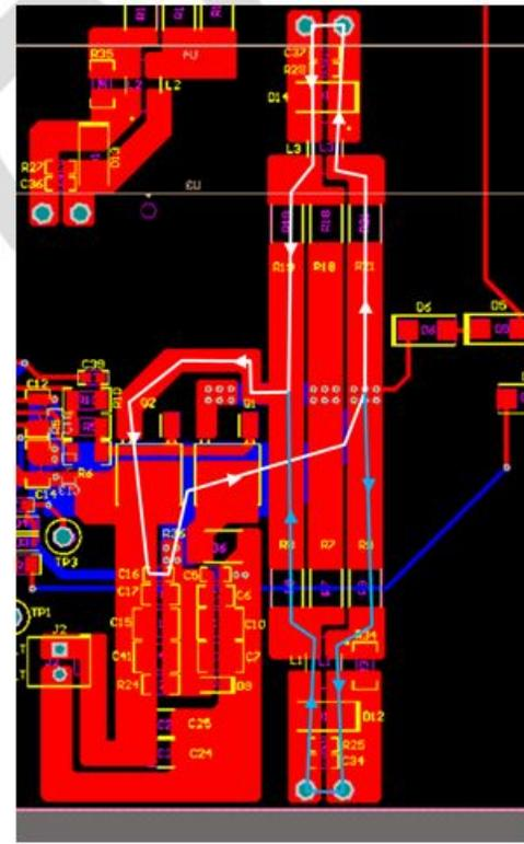
Figure 34. IGBT Gate Turnoff Current Path
