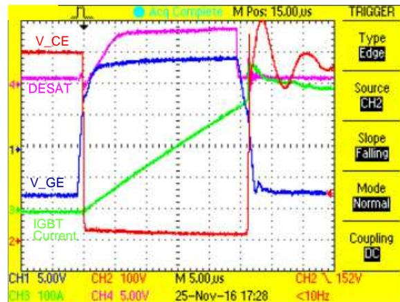
**Figure 28. IGBT DESAT Waveform Showing  $V_{CE}$**
