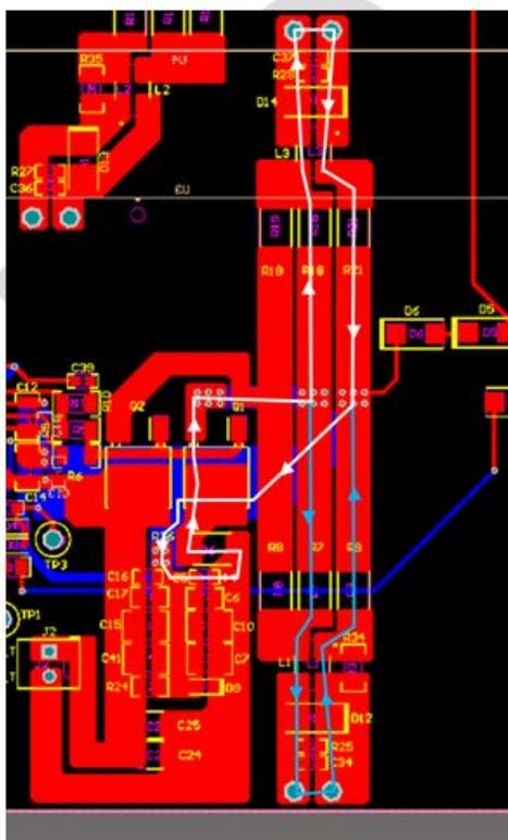
Figure 33. IGBT Gate Turnon Current Path
