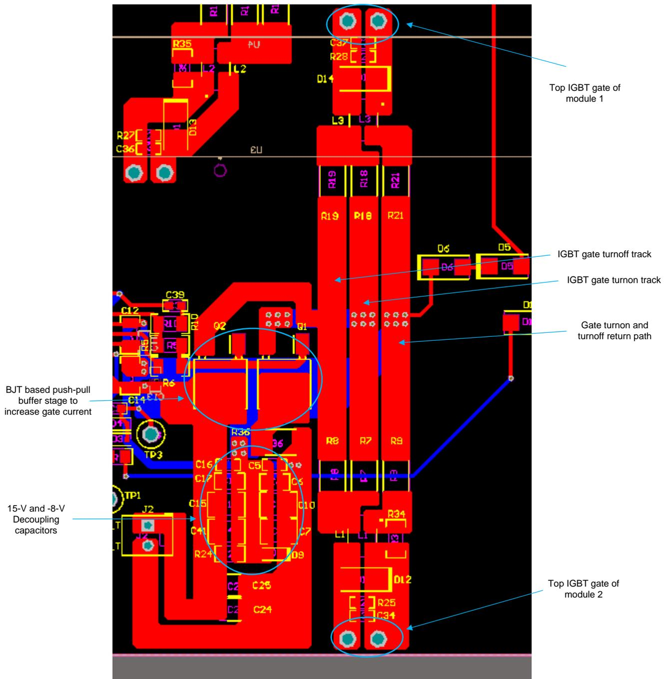
**Figure 30. Current Buffer Stage Interface to IGBT Gate**
