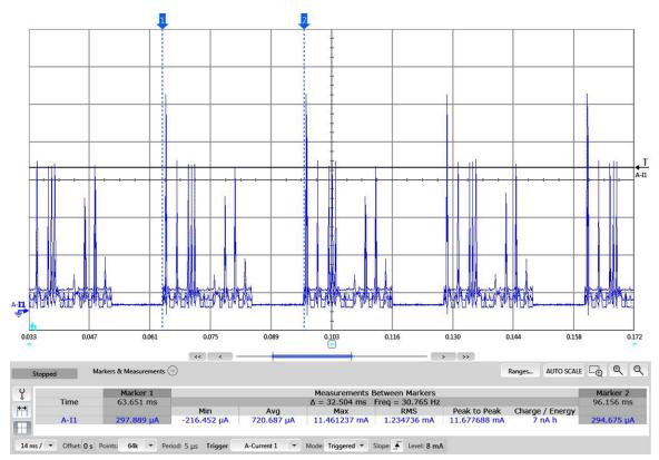
Figure 13. Current Consumption Timing With UART and LPM0 Sleep
