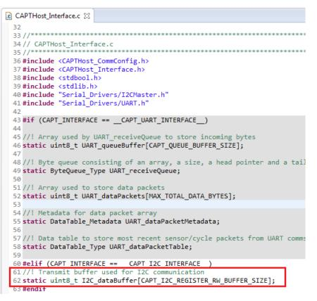
Figure 8. I2C\_dataBuffer Array in CAPTHost\_Interface.c
