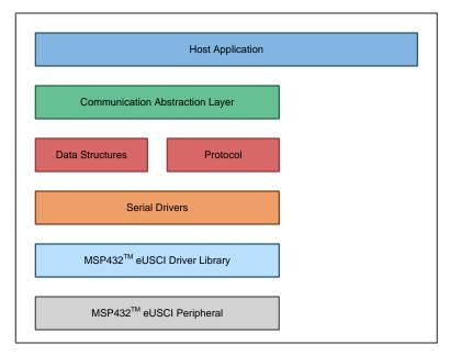
Figure 5. MSP432<sup>™</sup> Host Application and Communications Module Organization
