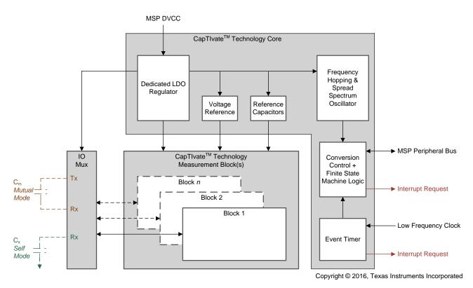
Figure 3. CapTlvate<sup>™</sup> Technology Block Diagram
