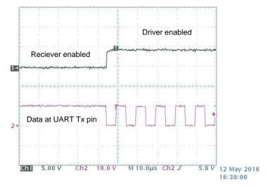
Figure 8. Enable Signal for 200 kbps
