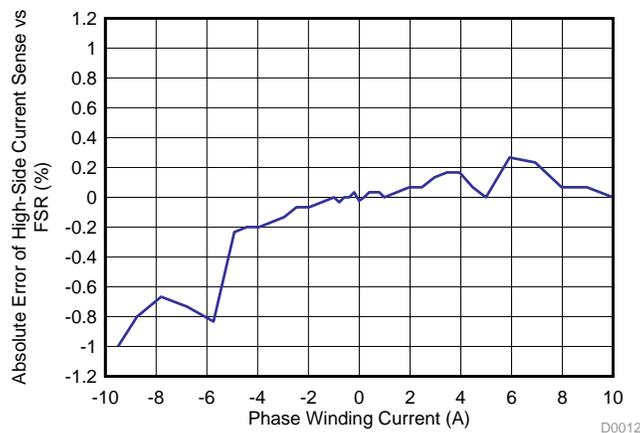
Figure 39. Absolute Error versus FSR ( $-15$  to 15 A) in % of SM72295 Current Sense Amplifier Output
