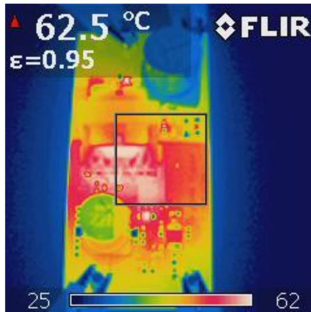
IR thermal image taken at steady state at 400mA load and VIN = 9.0V for two minutes with no airflow (4 Layer board, 1 Oz copper layer)
