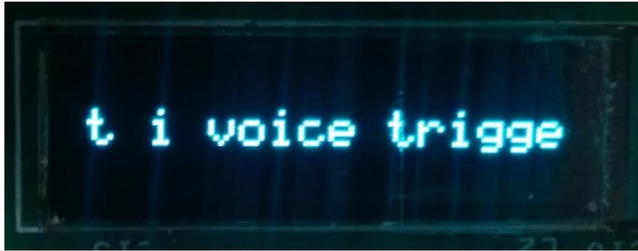
**Figure 8. OLED on C5535 eZdsp After the Keyword Phrase is Recognized**
