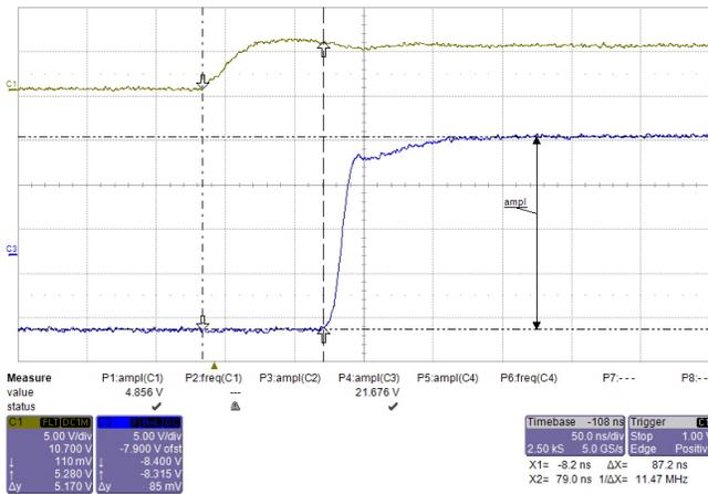
Figure 69. PWM Turnon Delay Between SN74LVC125A-Q1 and BJT
