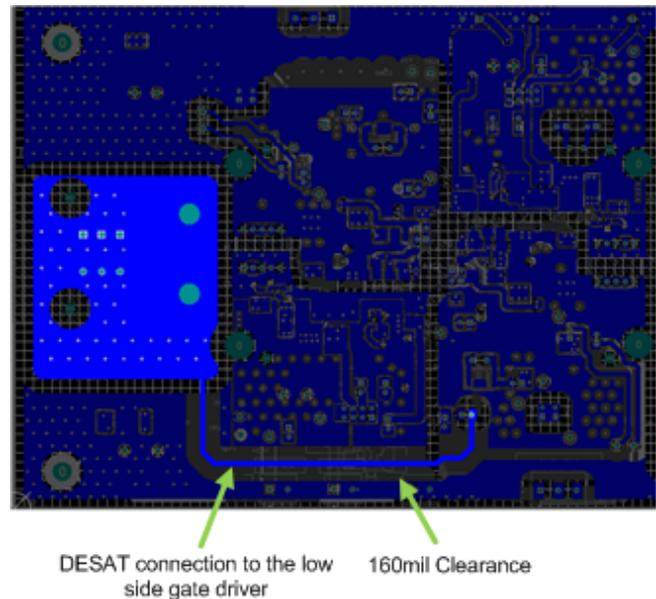
**Figure 108. PCB Trace From DESAT to Low-Side Driver**
