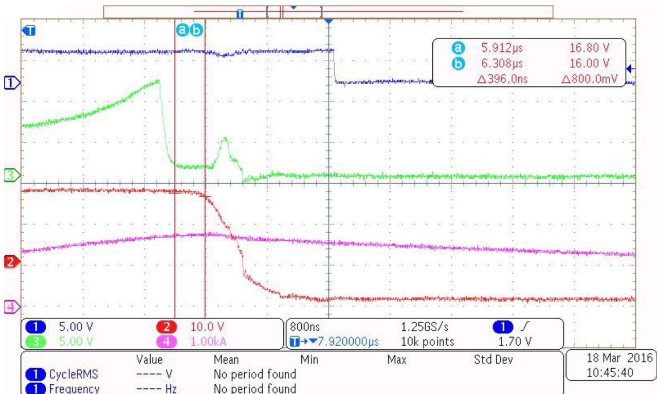
Figure 95. DESAT Protection Response Time
