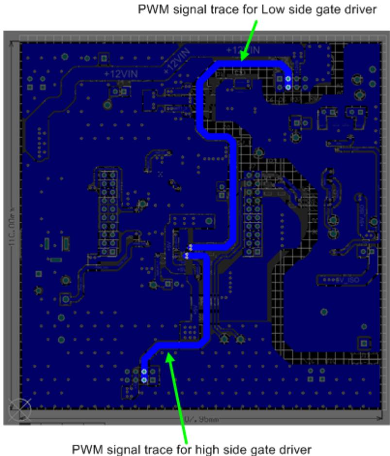
**Figure 118. PCB Traces From PWM Signals to IGBT Gate Drivers**
