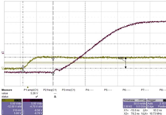
Figure 71. PWM Rise Slope With 22-Ω Base Resistor
