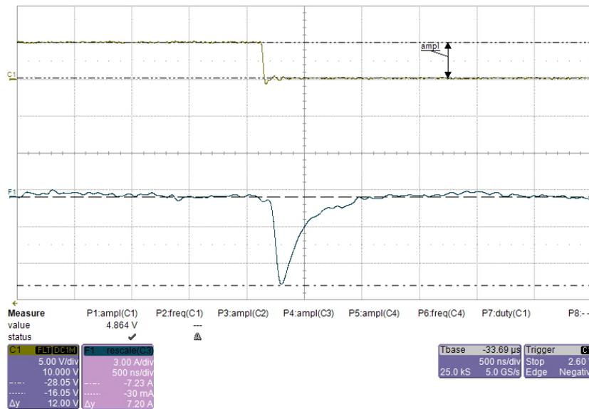
Figure 84. Sink Current of BJT Current Boost Under 100-nF Load (7.20-A Peak)
