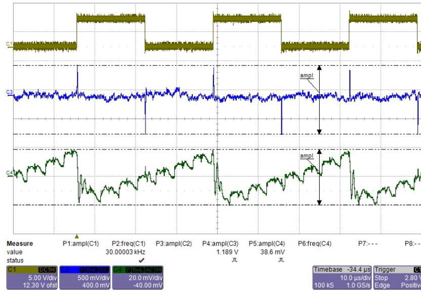
Figure 47. +15-V Output Ripple With BJT Current Boost
