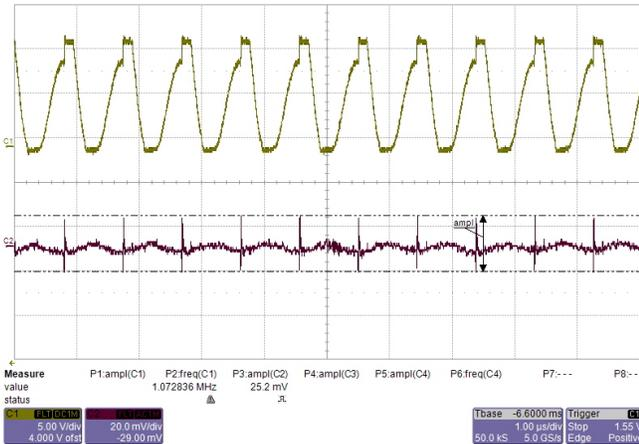
Figure 51. +5-V Output Ripple With No Load
