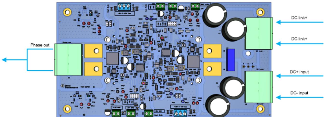
Figure 31. Power Connectors for DC Link
