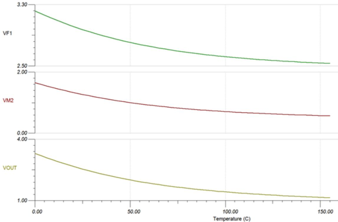
**Figure 22. Simulated Results of NTC AFE Circuit**
