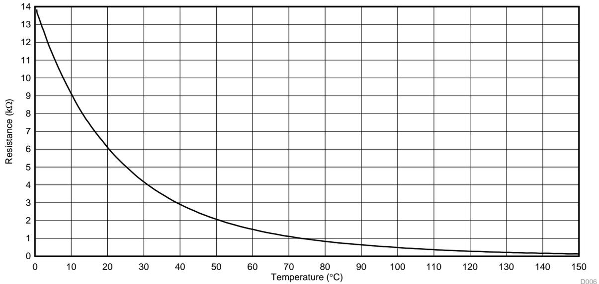
**Figure 63. Calculated Temperature-Resistance Characteristic of NTC Thermistor**
