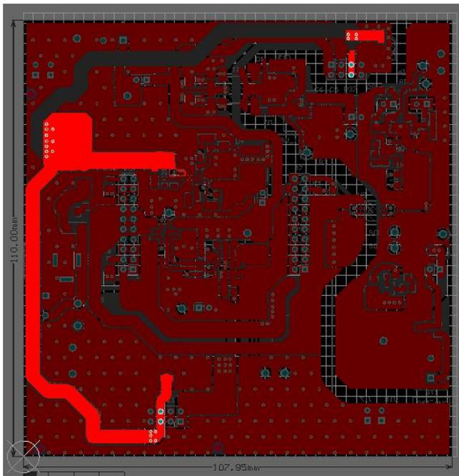
Figure 114. 12-V Power Rail on Top Layer
