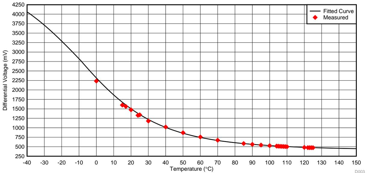
Figure 62. Comparison Between Measured and Calculated Differential Voltages at ADC Input
