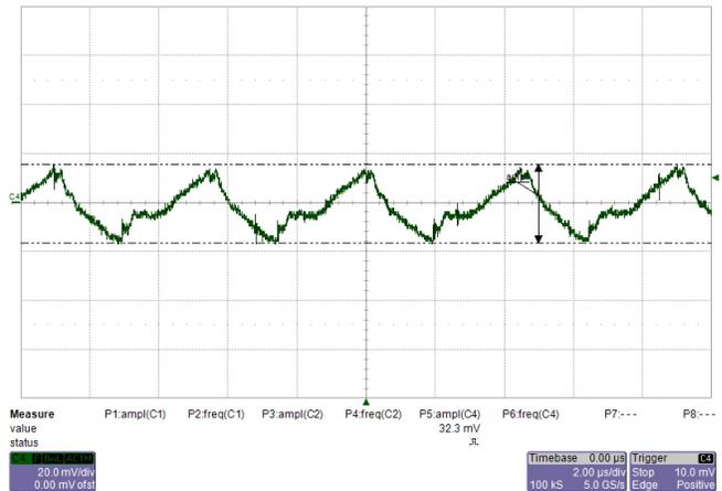
Figure 43. -9-V Rail Output Ripple With Full Load
