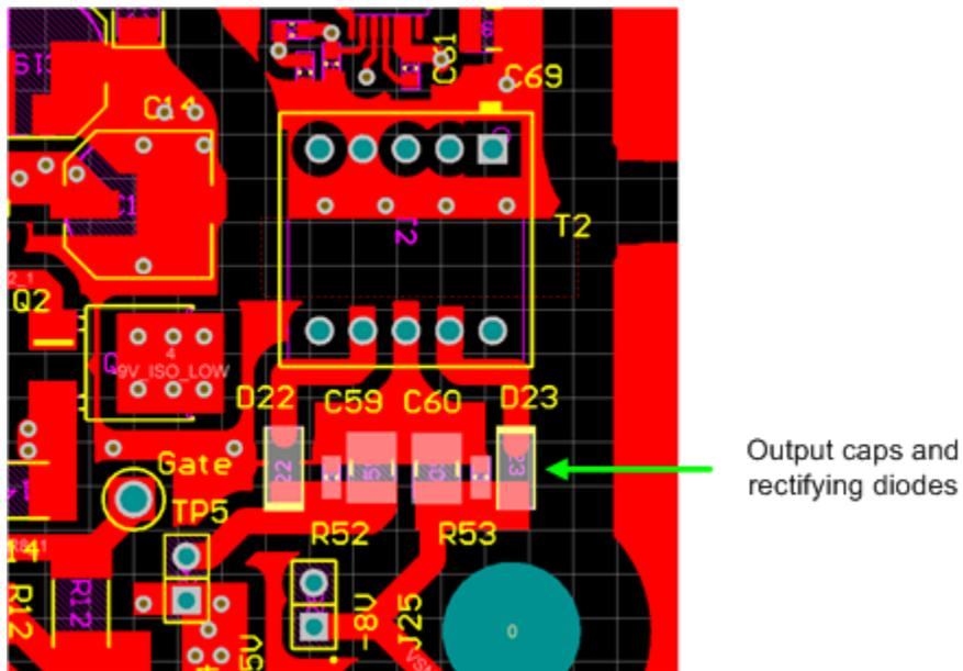
Figure 110. Placement of Transformer Secondary Components
