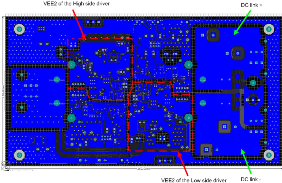
**Figure 106. Fourth Layer of Gate Driver Board**
