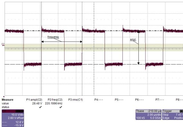
Figure 38. Voltage Waveforms at LM5160-Q1 Switch Node With No Load
