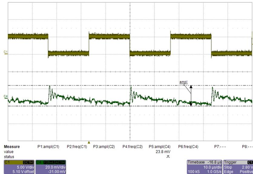
Figure 45. -9-V Output Ripple at Transition of 5-A Source Current
