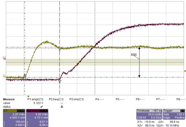
Figure 72. PWM Rise Slope With 3.3-Ω Base Resistor
