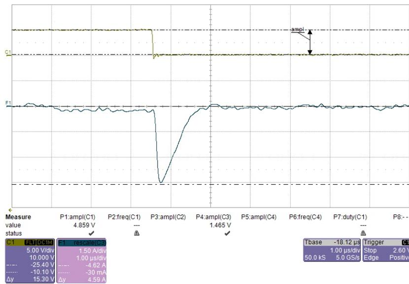
Figure 81. Sink Current of ISO5852S Under 100-nF Load (4.59-A Peak)
