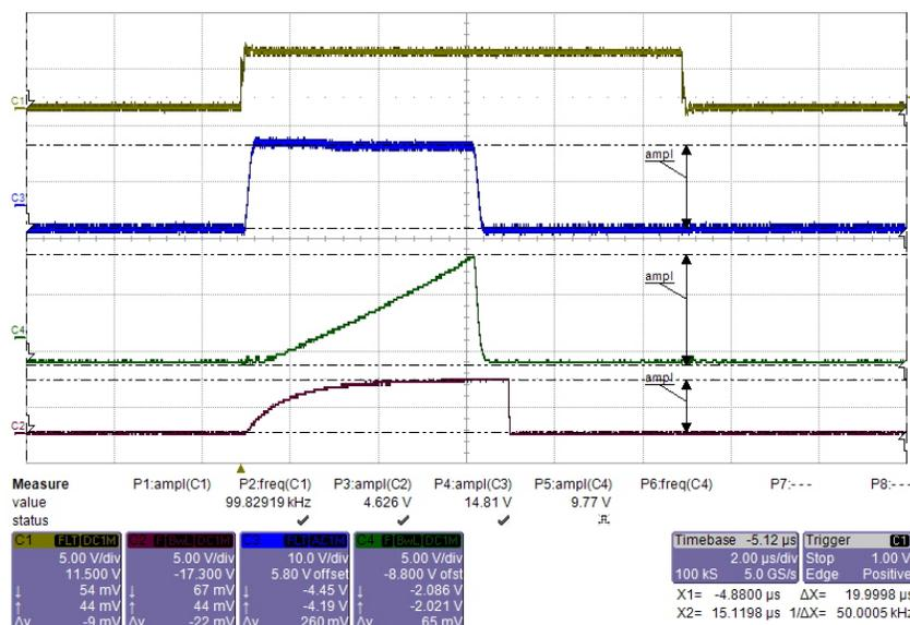
Figure 89. DESAT Protection — RST Pin Toggled With 50 kHz
