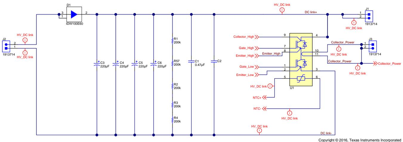
Figure 13. Schematic of Power Stage
