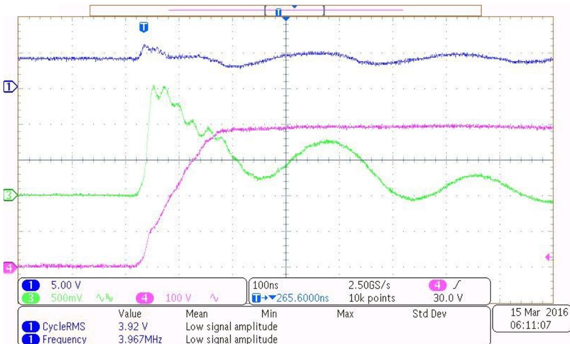
Figure 87. Active Miller Clamp Enabled
