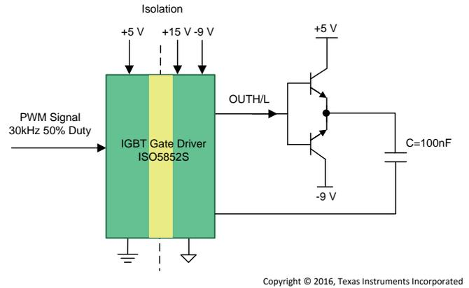
Figure 76. Test Circuit of BJT Current Boost
