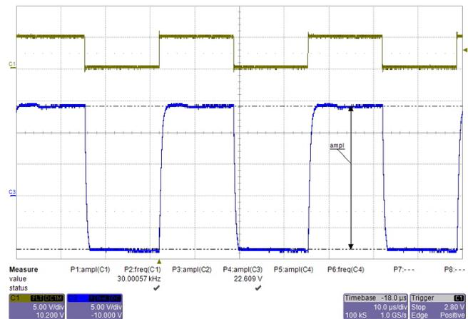
Figure 78. PWM Signal of Gate Driver With BJT Current Boost
