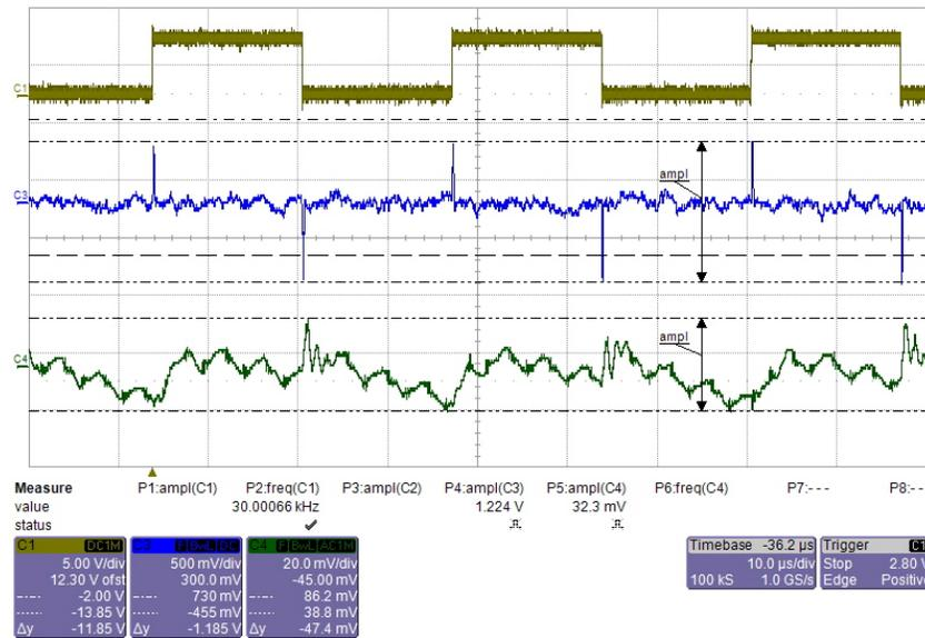
Figure 48. -9-V Output Ripple With BJT Current Boost
