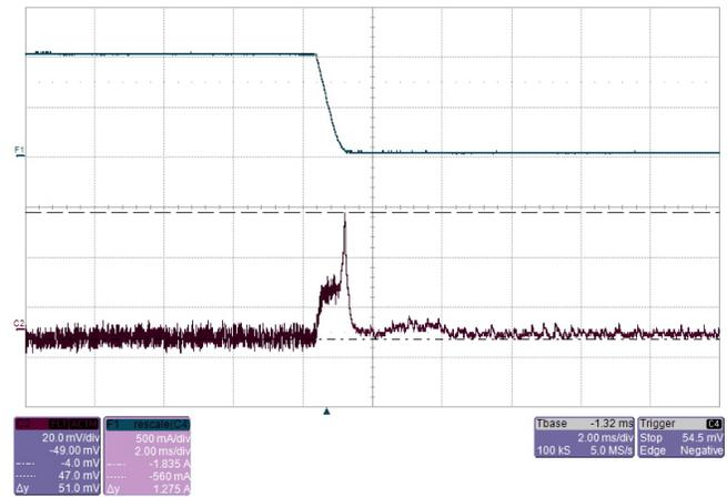
Figure 54. +5-V Load Dump During Load Step-Down
