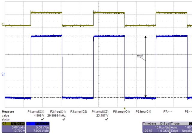
Figure 67. PWM Signals at Output of ISO5852S Gate Driver
