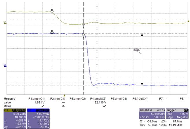
Figure 70. PWM Turnoff Delay Between SN74LVC125A-Q1 and BJT
