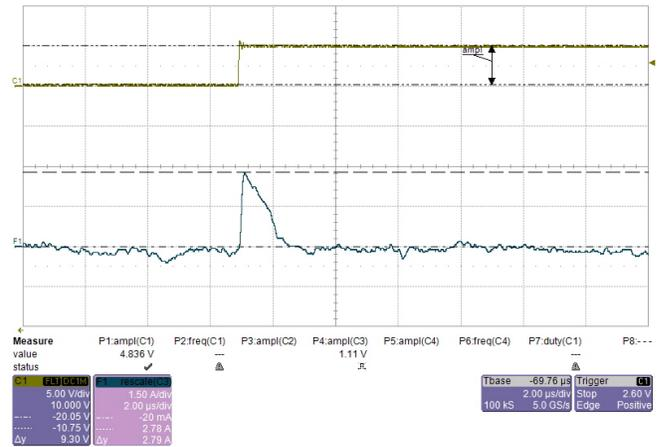
Figure 80. Source Current of ISO5852S Under 100-nF Load (2.79-A Peak)
