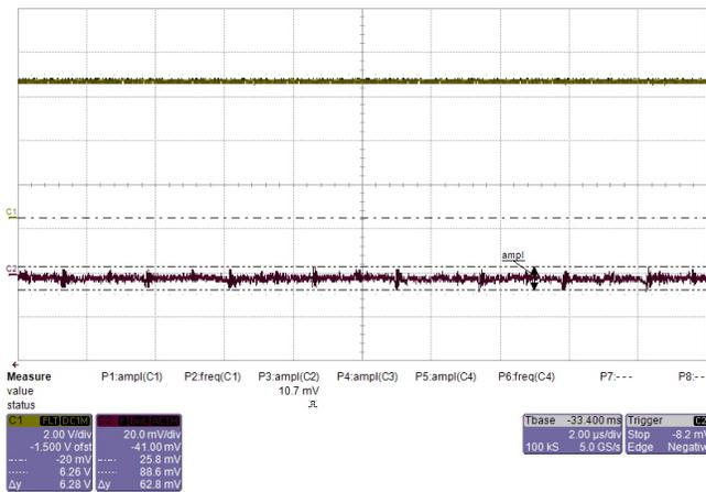
Figure 56. Output Ripple of Secondary Side of Transformer at No Load
