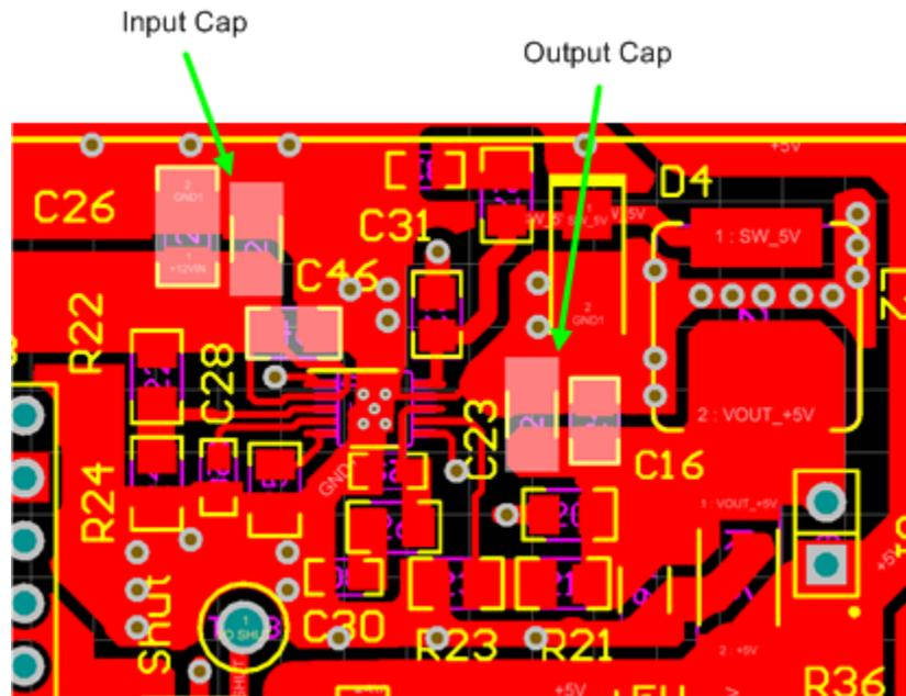
Figure 119. Placement of Input and Output Capacitors
