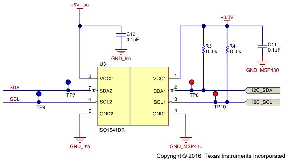
**Figure 23. I<sup>2</sup>C Isolation Schematic**
