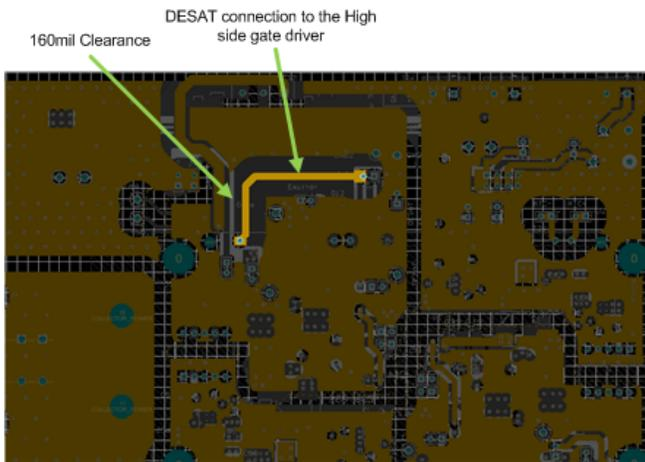
**Figure 107. PCB Trade From DESAT to High-Side Driver**
