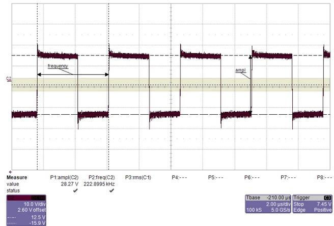
Figure 39. Voltage Waveforms at LM5160-Q1 Switch Node With Full Load
