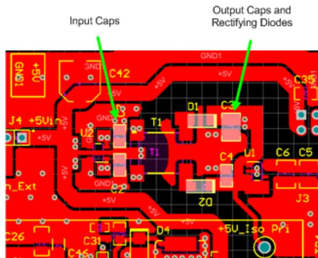
Figure 120. Placement of Input Capacitors and Output Components
