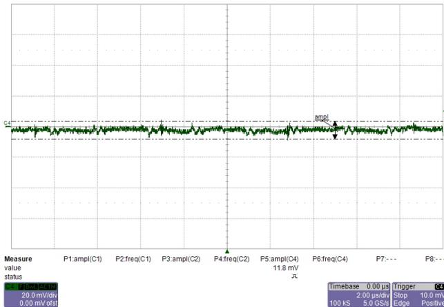
Figure 42. -9-V Rail Output Ripple With No Load
