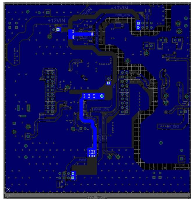
Figure 117. 5-V Power Rail on Bottom Layer
