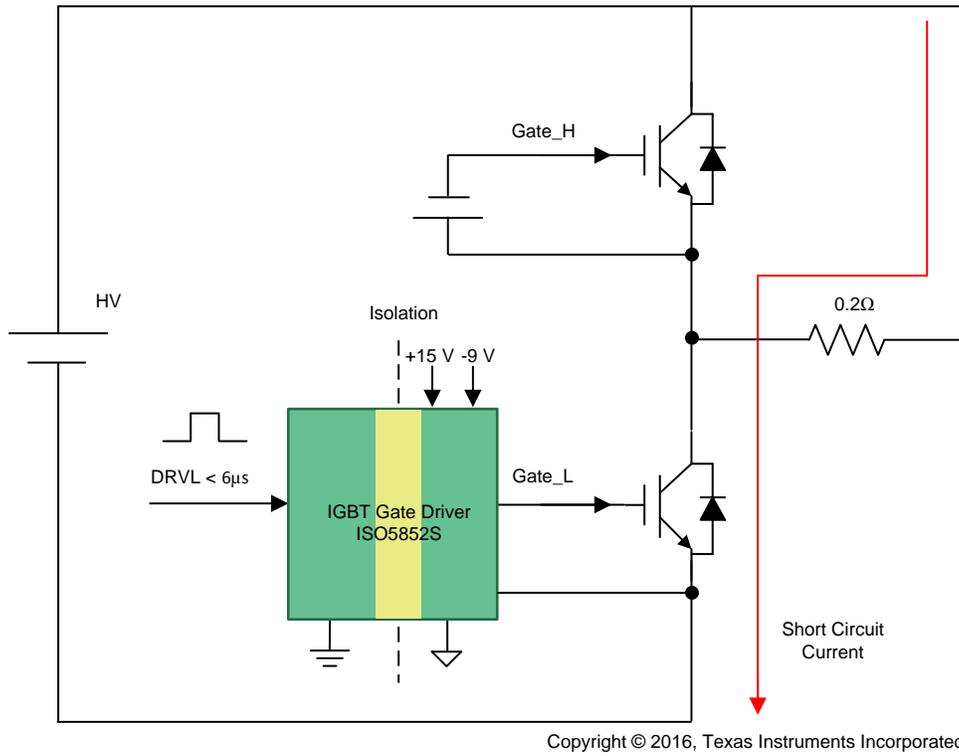
**Figure 93. Test Circuit for Driver Desaturation Protection**
