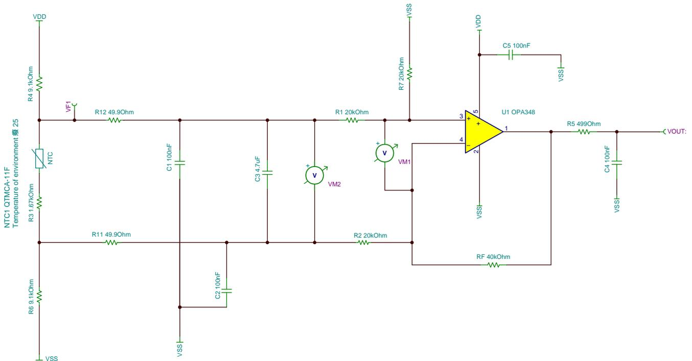
Figure 21. NTC Signal Conditioning AFE Simulation Circuit
