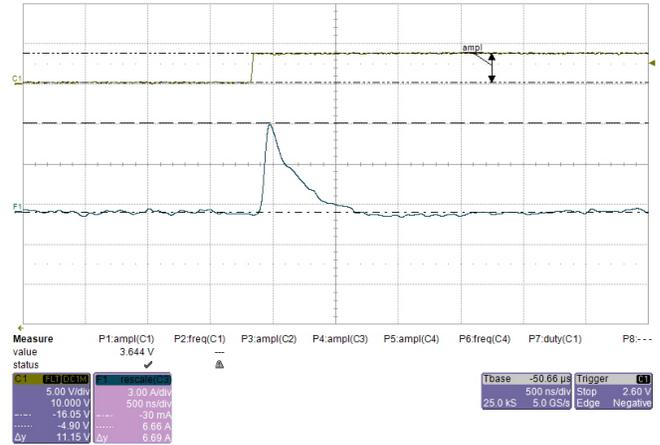
Figure 83. Source Current of BJT Current Boost Under 100-nF Load (6.69-A Peak)
