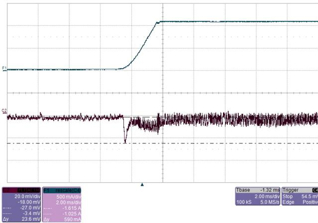
Figure 53. +5-V Load Dump During Load Step-Up
