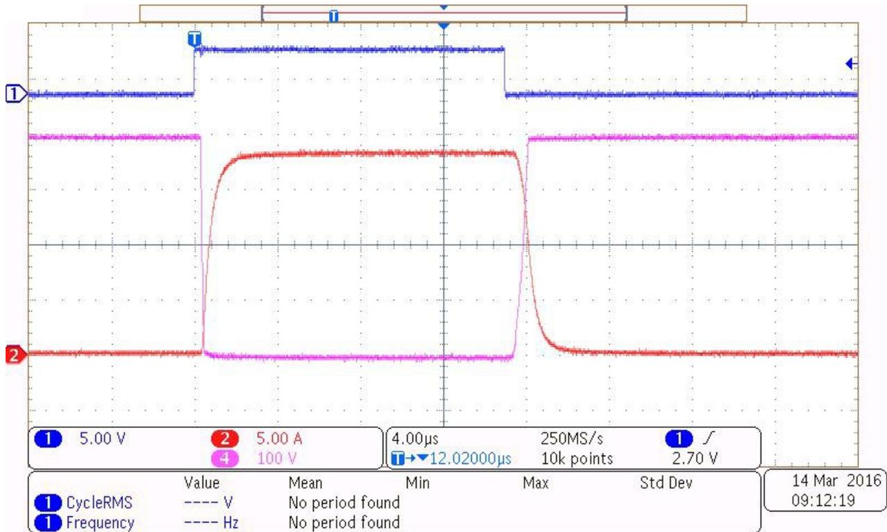
Figure 98. IGBT Switching Waveforms
