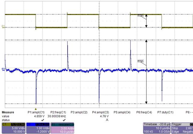
Figure 82. Sink and Source Current With BJT Current Boost Under 100-nF Load
