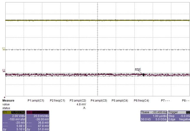
Figure 58. Output Ripple of LDO at No Load
