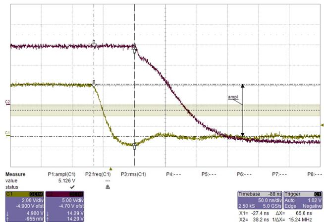
Figure 74. PWM Fall Slope With 3.3-Ω Base Resistor
