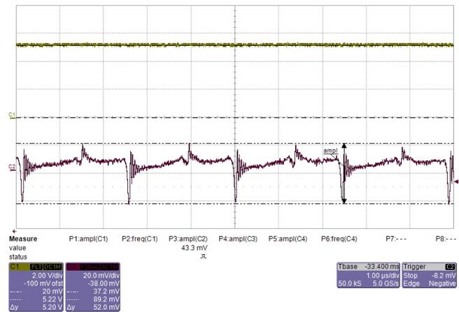
Figure 57. Output Ripple of Secondary Side of Transformer at Full Load
