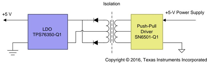
Figure 55. Diagram of Push-Pull Isolated Power Supply
