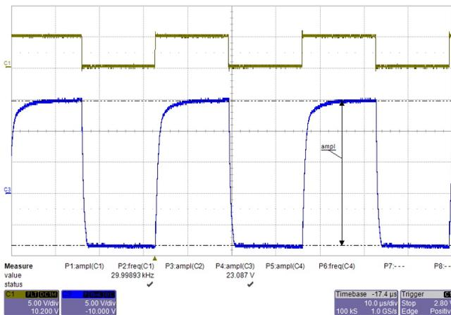
Figure 77. PWM Signal of Gate Driver Without BJT Current Boost
