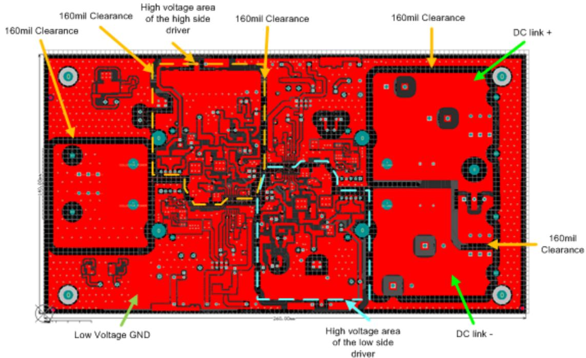
**Figure 103. Top Layer of Gate Driver Board**
