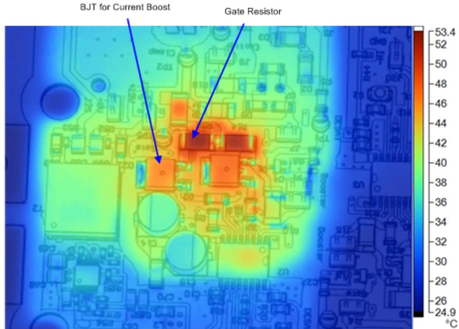
Figure 101. Thermal Image of Gate Driver Board at 100-nF Load for 30 Minutes
