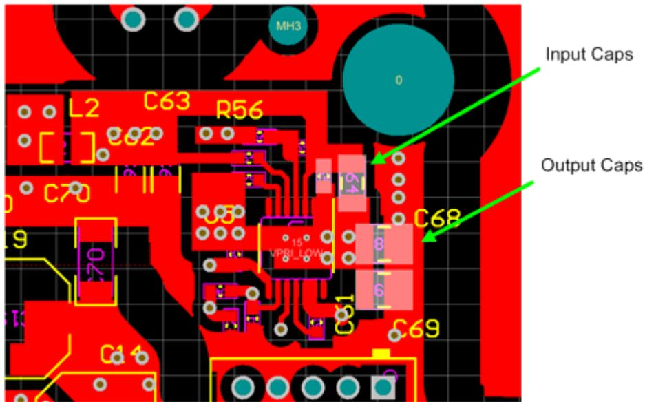
Figure 109. Placement of Input and Output Capacitors in Fly-Buck™ Converter
