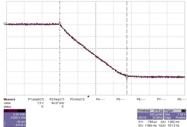
Figure 37. -9-V Rail During Startup
