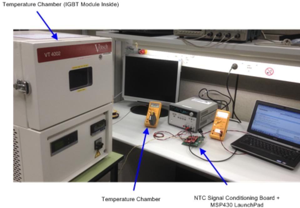
Figure 61. Test Setup for NTC Signal Conditioning Board
