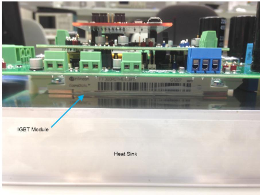
Figure 30. Placement of IGBT Module
