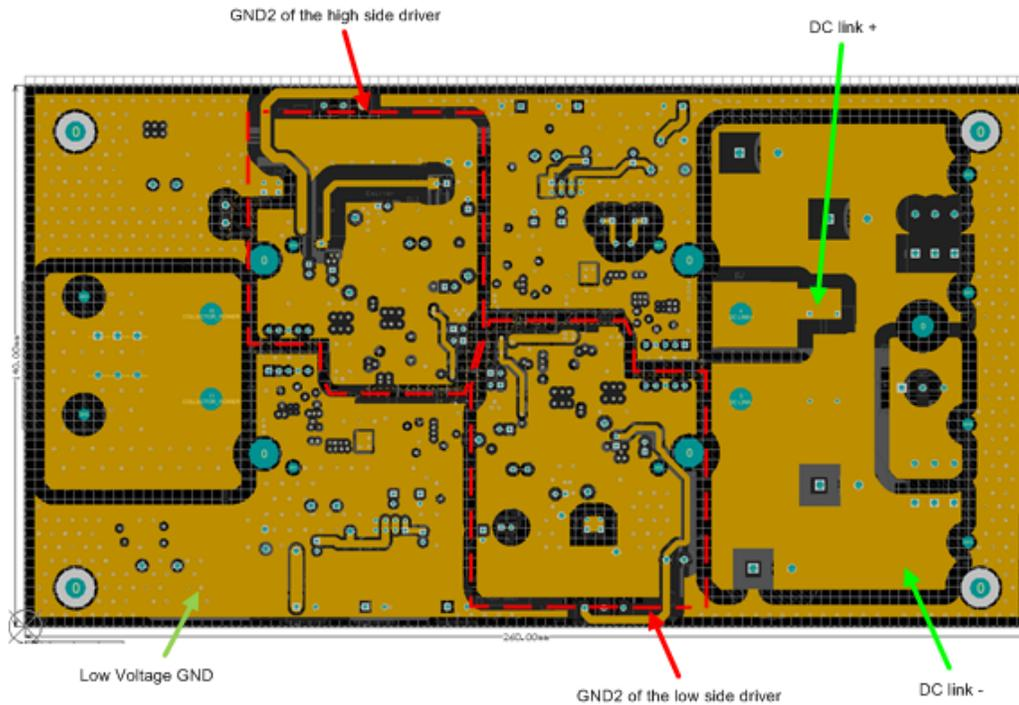
Figure 104. Second Layer of Gate Driver Board
