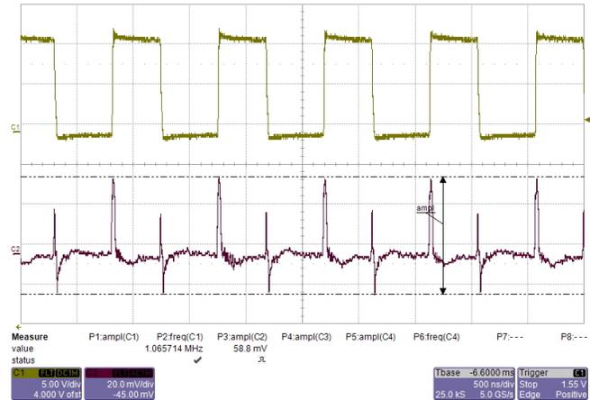
Figure 52. +5-V Output Ripple With Full Load (1 A)
