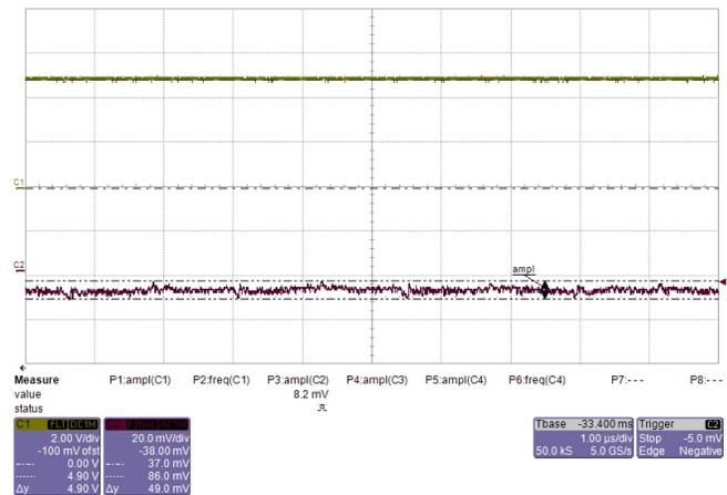
Figure 59. Output Ripple of LDO at Full Load
