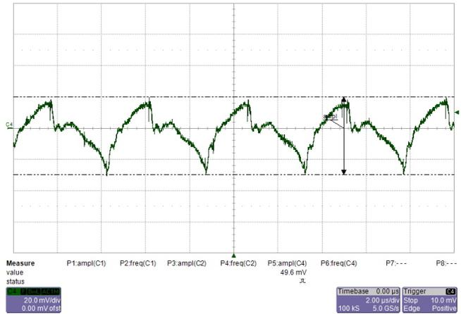
Figure 41. +15-V Rail Output Ripple With Full Load
