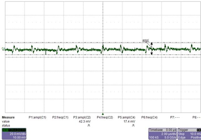
Figure 40. +15-V Rail Output Ripple With No Load
