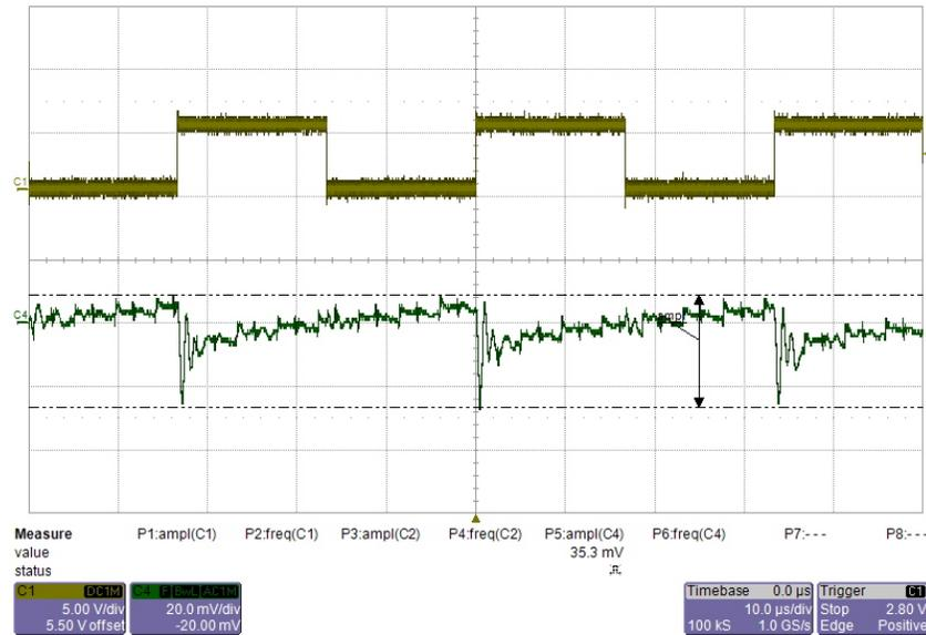
Figure 44. +15-V Output Ripple at Transition of 2.5-A Source Current
