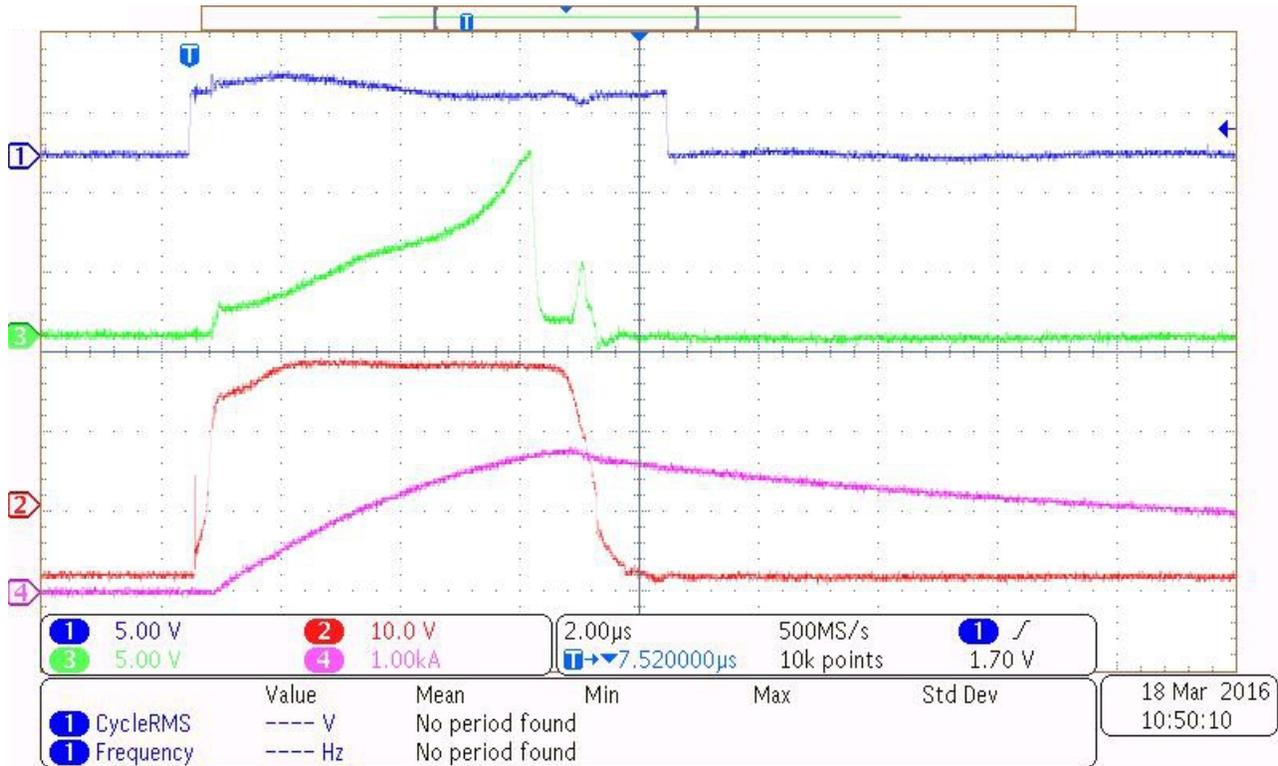
Figure 94. DESAT Protection Test With BJT Push-Pull Current Boost
