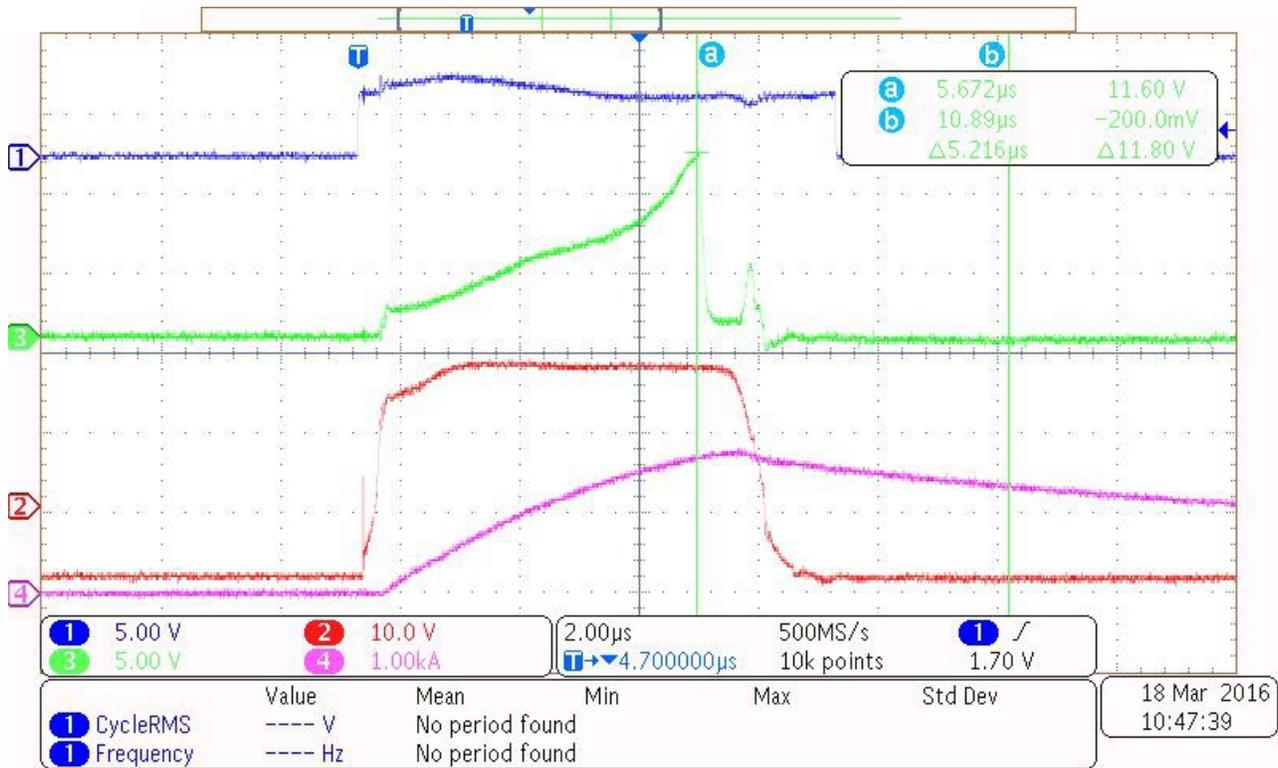
Figure 96. DESAT Detection Threshold
