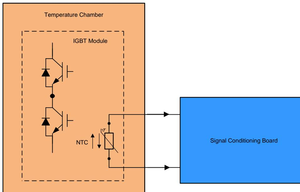
Figure 60. Test Circuit for NTC Signal Conditioning Board
