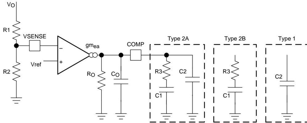
Figure 16. Different Types of Frequency Compensation
