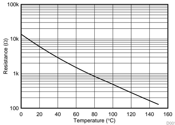
**Figure 1. Resistance – Temperature Characteristic of NTC Inside Infineon Module**
