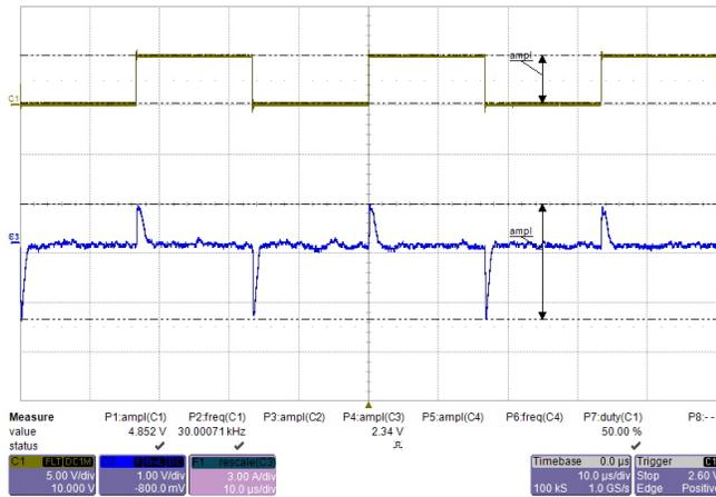
Figure 79. Sink and Source Currents of ISO5852S Under 100-nF Load
