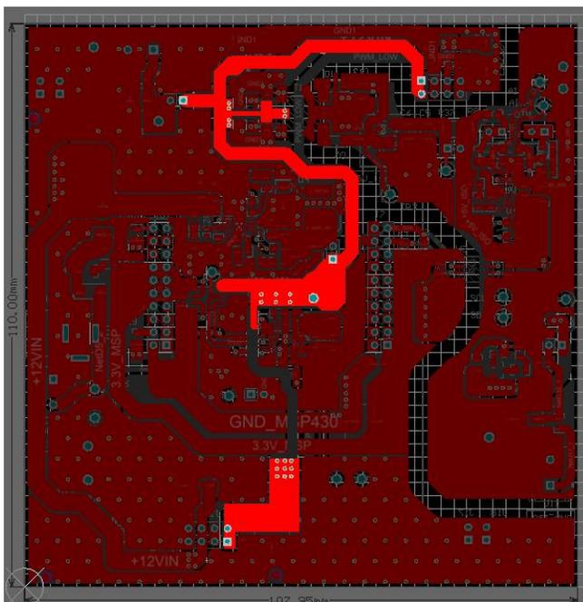
Figure 116. 5-V Power Rail on Top Layer
