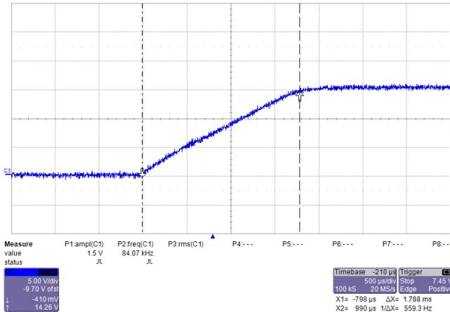
Figure 36. +15-V Rail During Startup
