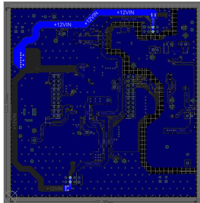
Figure 115. 12-V Power Rail on Bottom Layer
