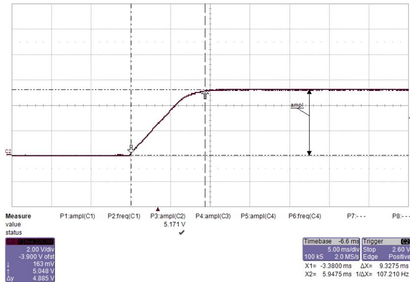
Figure 50. Startup Waveform of Step-Down Converter
