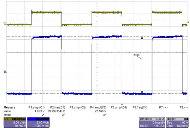
Figure 68. PWM Signals at Output of BJT Current Boost
