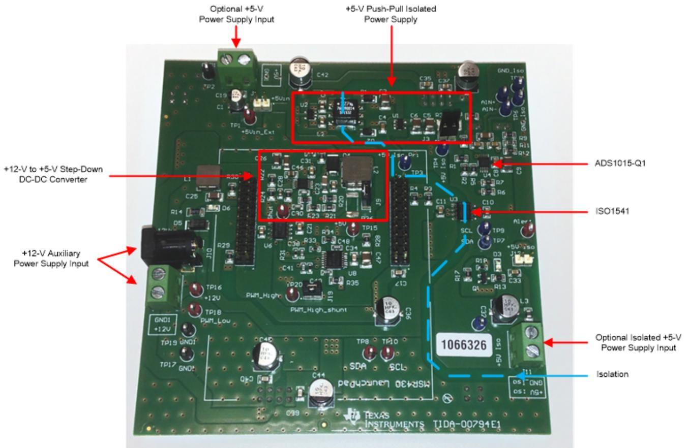
Figure 29. PCB of NTC Signal-Conditioning Board
