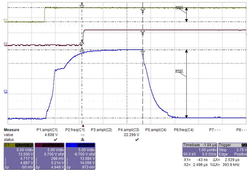
Figure 66. High Temperature Shutdown Propagation Delay
