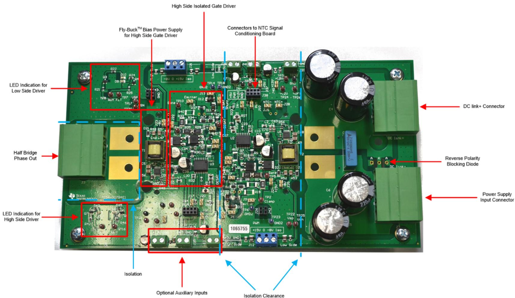
Figure 28. PCB of IGBT Gate Driver Board
