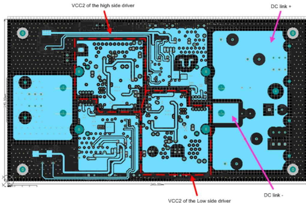
Figure 105. Third Layer of Gate Driver Board
