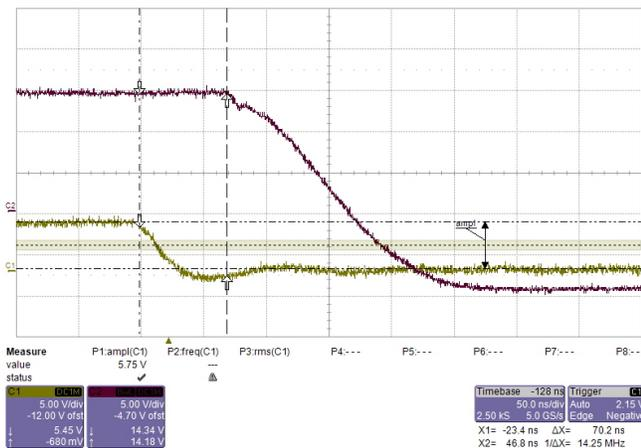
Figure 73. PWM Fall Slope With 22-Ω Base Resistor
