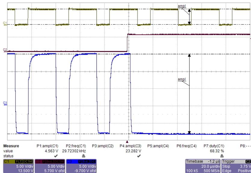
Figure 65. High Temperature Shutdown Response
