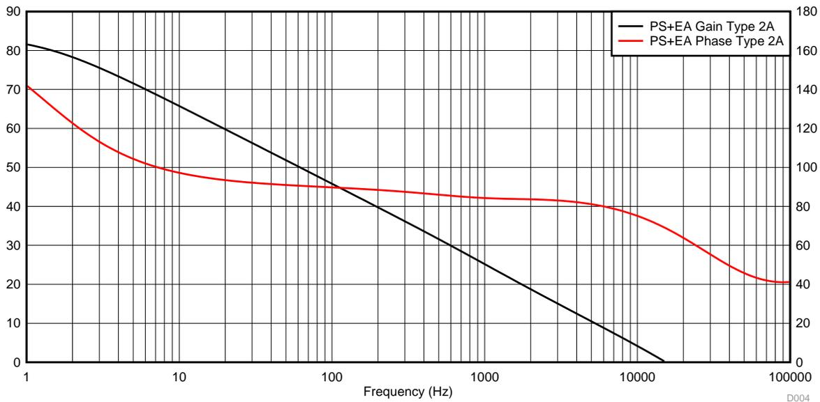
Figure 17. Achieved Gain and Phase Margin of 12-V to 5-V Step-Down DC-DC Converter
