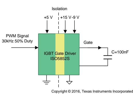
Figure 75. Test Circuit of ISO5852S
