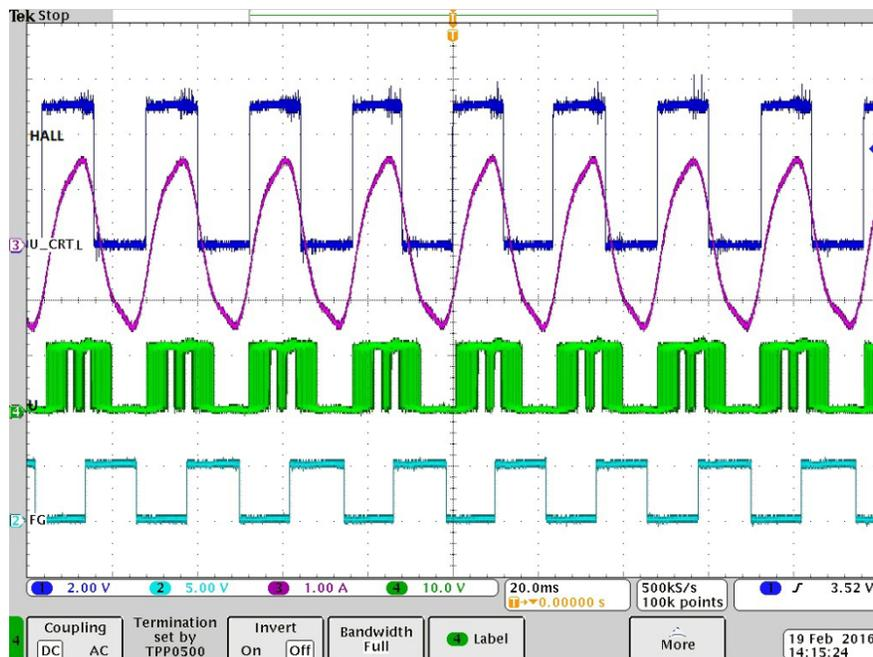
Figure 8. DRV10970 Driving Motor With Three-Hall Mode
