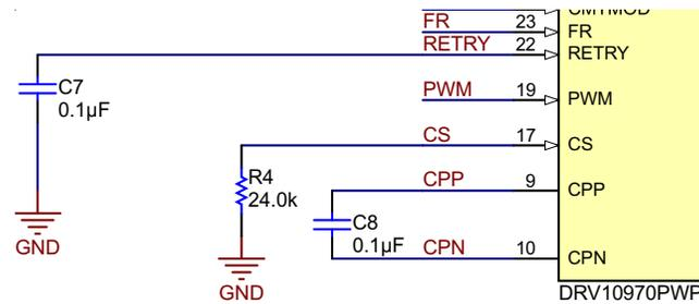
**Figure 4. Current Sense and Retry Circuit**
