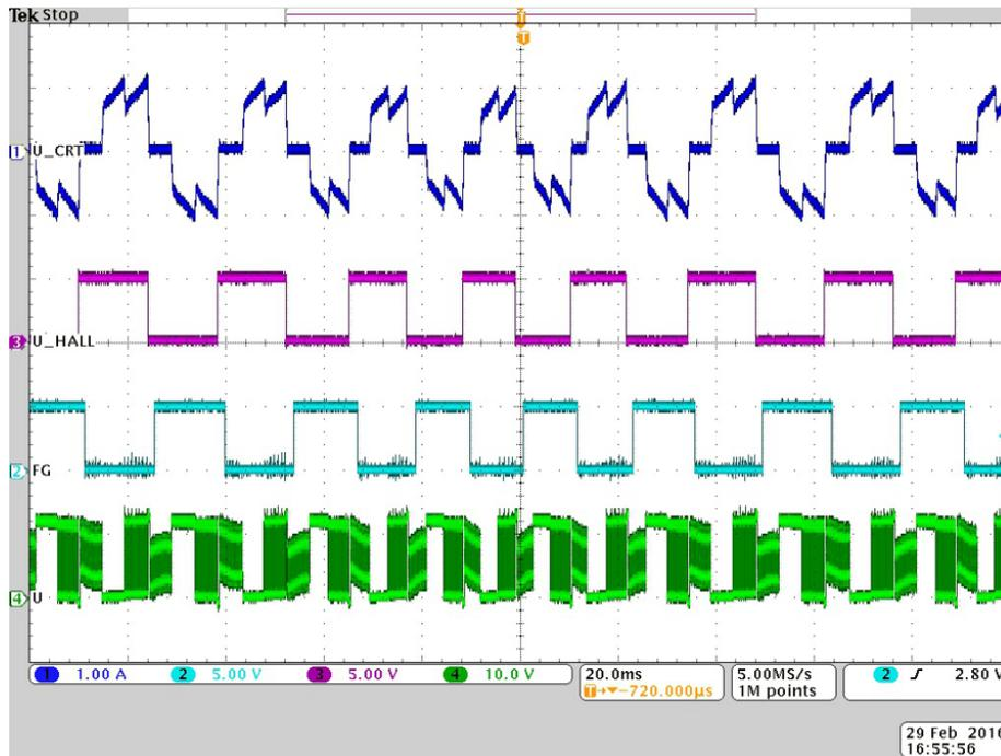
Figure 9. DRV10970 Driving With Trapezoidal Mode
