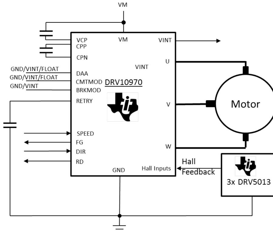
Figure 6. TIDA-00919 Block Diagram
