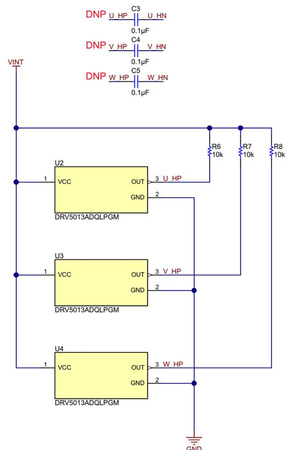
Figure 2. Hall Sensor Connections
