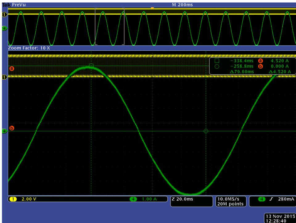
Figure 19. Motor #2 Peak 4.5A(RMS3.2A) at 1/64 micro-stepping
