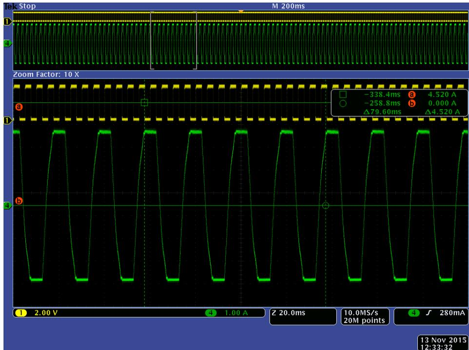
Figure 13. Motor #2 Peak 4.5A(RMS3.2A) at Full step
