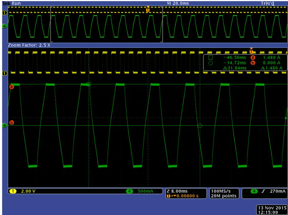
Figure 4. Motor #1 Peak 2A(RMS1.43A) at Full step
