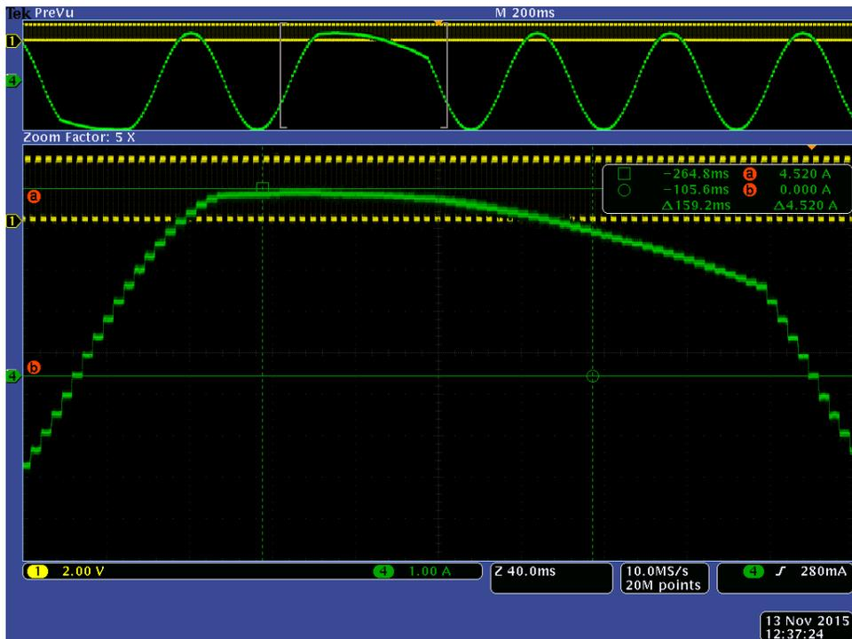
Figure 23. Motor #2 online change from 1/16 to 1/128 micro-stepping
