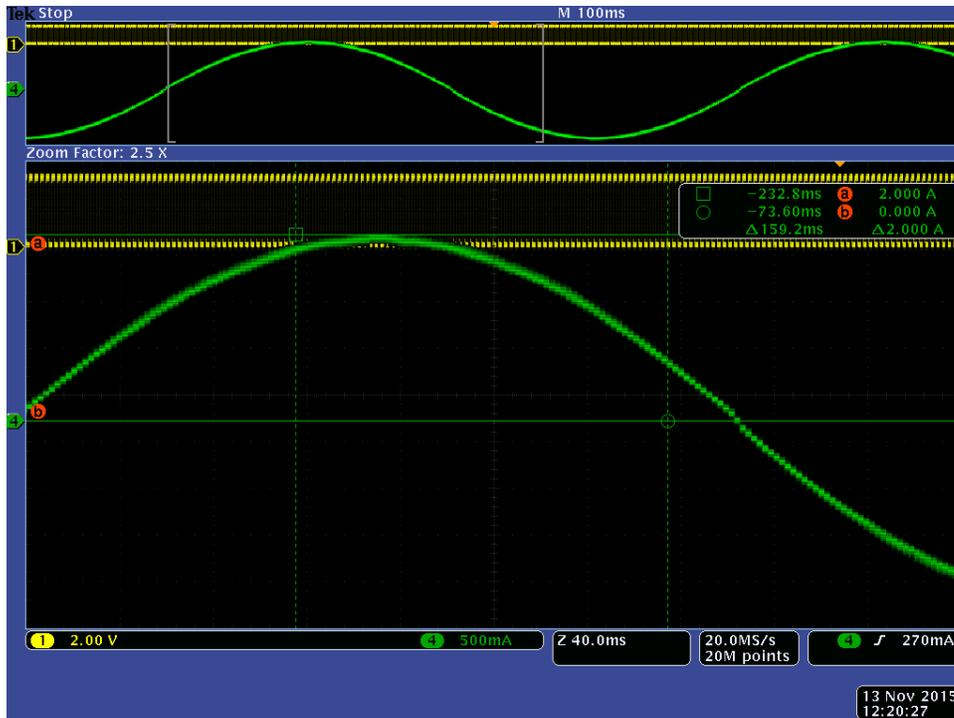
Figure 10. Motor #1 Peak 2A(RMS1.43A) at 1/64 micro-stepping
