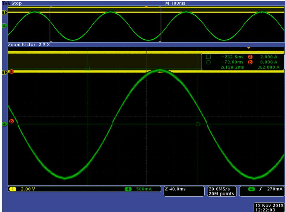
Figure 12. Motor #1 Peak 2A(RMS1.43A) at 1/256 micro-stepping
