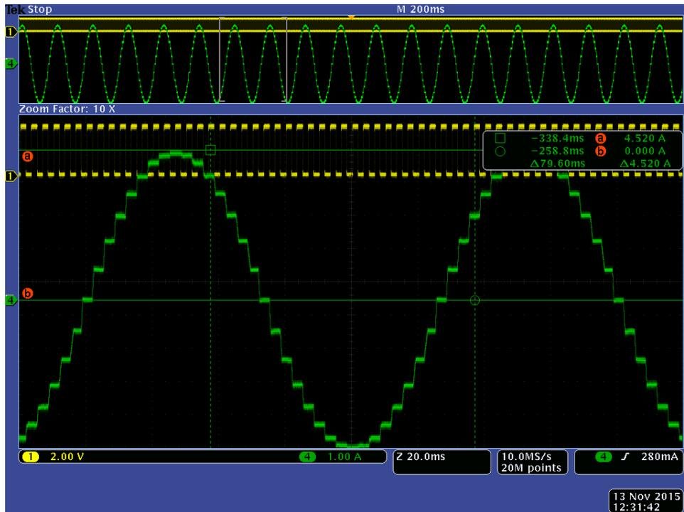
Figure 16. Motor #2 Peak 4.5A(RMS3.2A) at 1/8 micro-stepping
