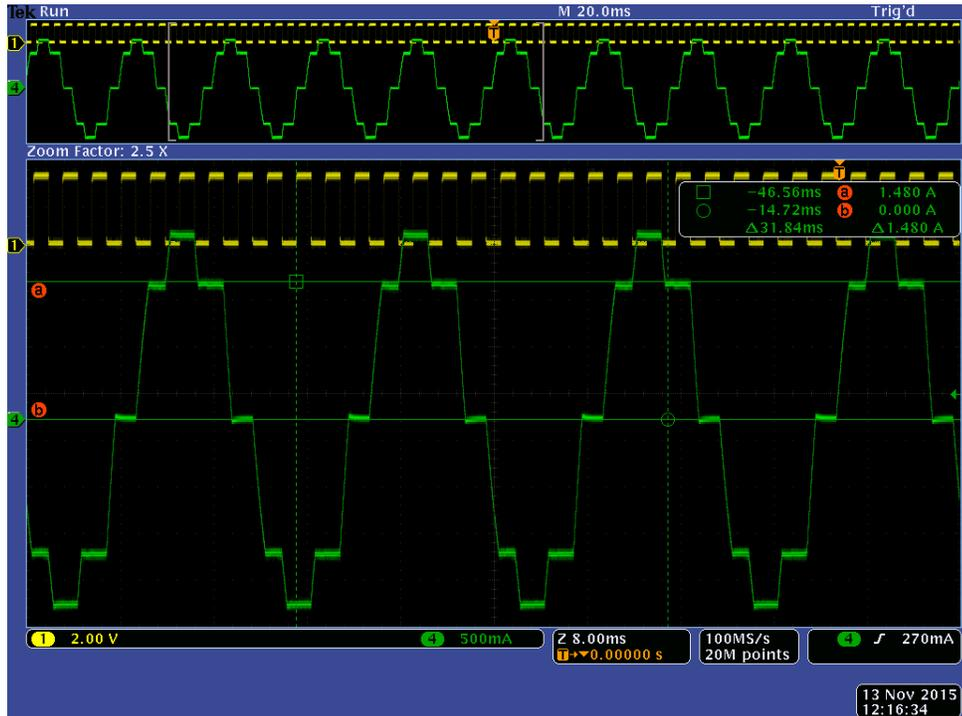
Figure 5. Motor #1 Peak 2A(RMS1.43A) at Half step
