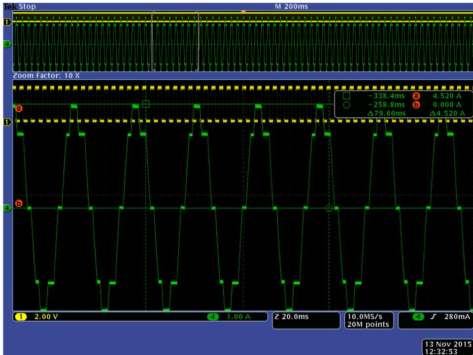
Figure 14. Motor #2 Peak 4.5A(RMS3.2A) at Half step
