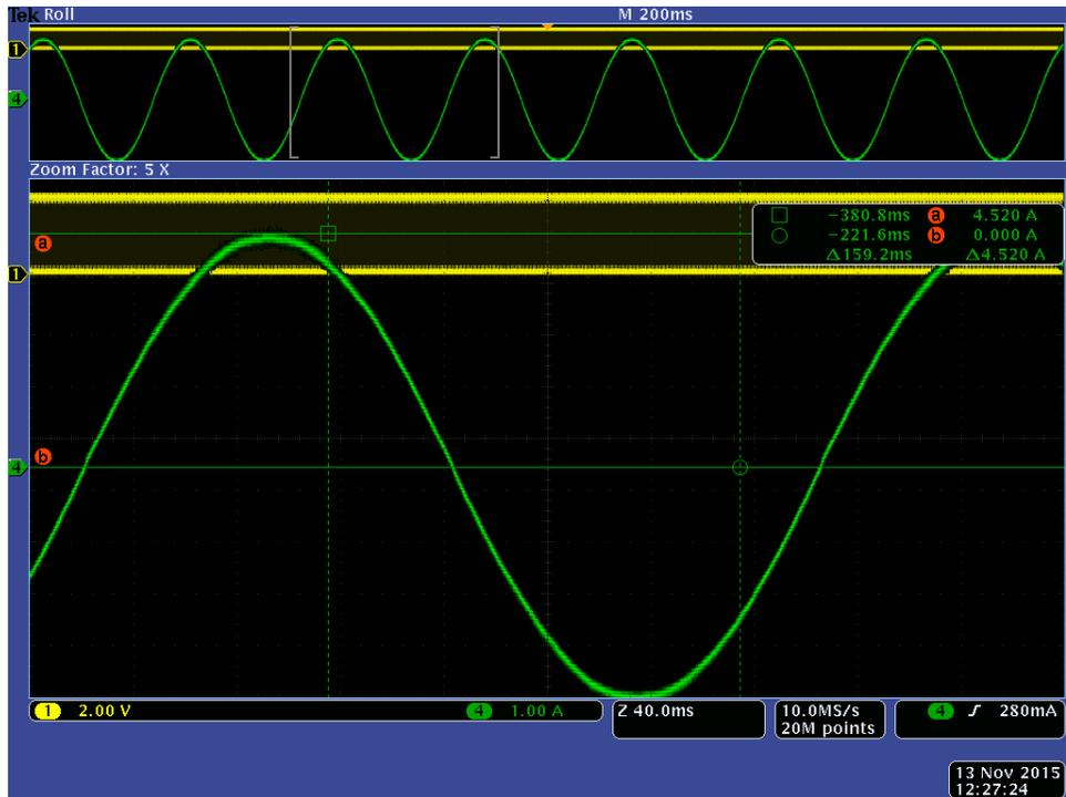
Figure 20. Motor #2 Peak 4.5A(RMS3.2A) at 1/128 micro-stepping
