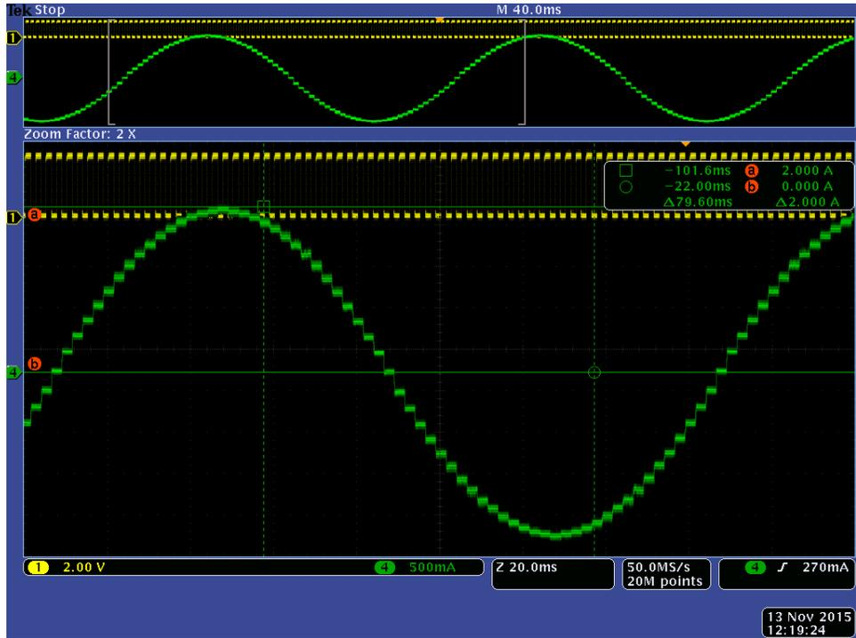
Figure 8. Motor #1 Peak 2A(RMS1.43A) at 1/16 micro-stepping
